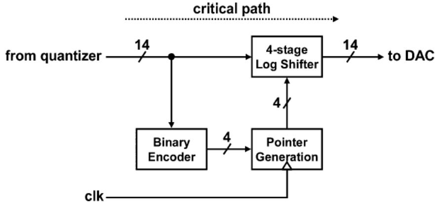
Fig. 3-16. Architecture of the DWA core logic.
