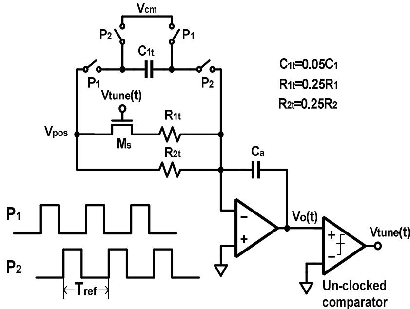
Fig. 6-3. SR tuning circuit.
