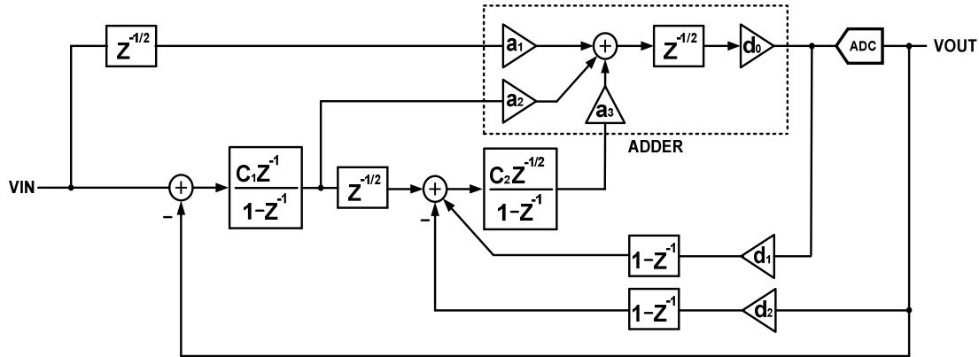
Fig. 2-5. Architecture of the proposed low-power delta-sigma ADC.
