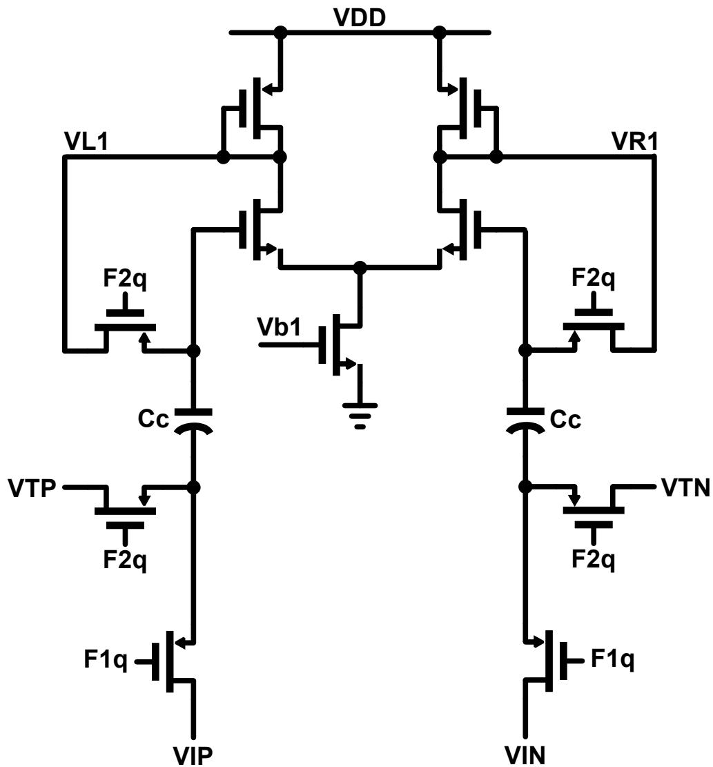
Fig. 3-11. The preamplifier with the offset cancellation scheme.
