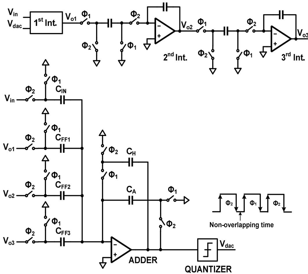
Fig. 5-7. Modified low-distortion  $\Delta\Sigma$  ADC.
