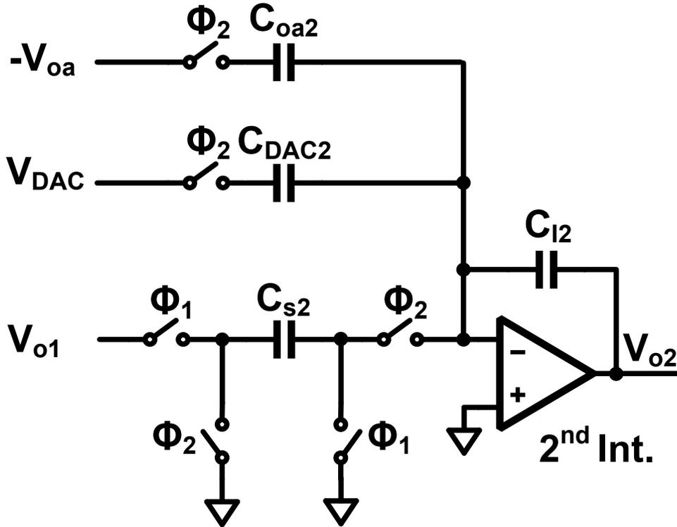
Fig. 3-6. The second integrator with differentiated quantization noise injection.
