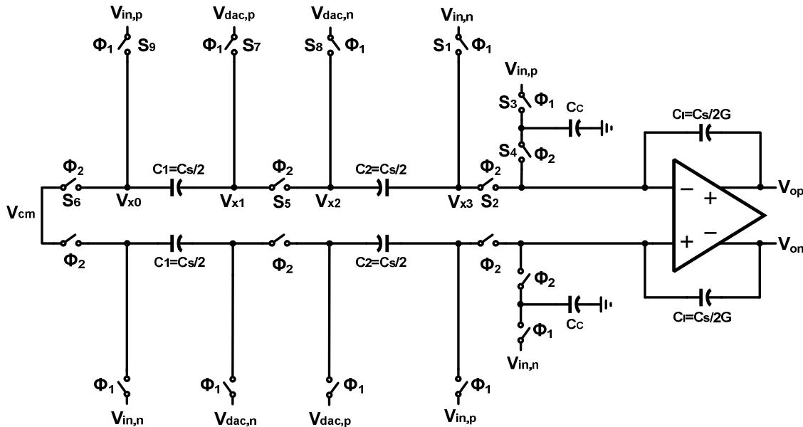
Fig. 5-5. Proposed low-power parasitic-insensitive SC integrator.
