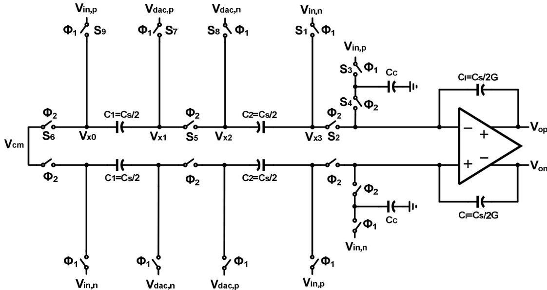
Fig. 5-5. Proposed low-power parasitic-insensitive SC integrator.
