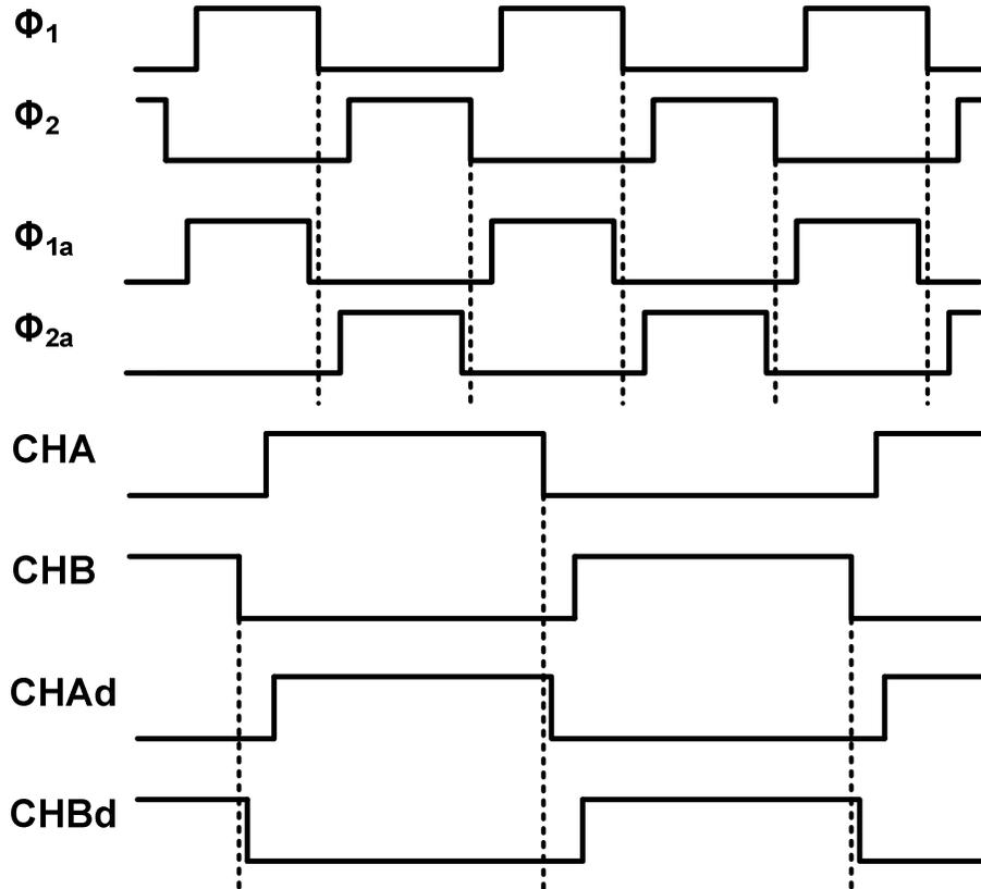
Fig. 3-2. The timing of the first integrator.
