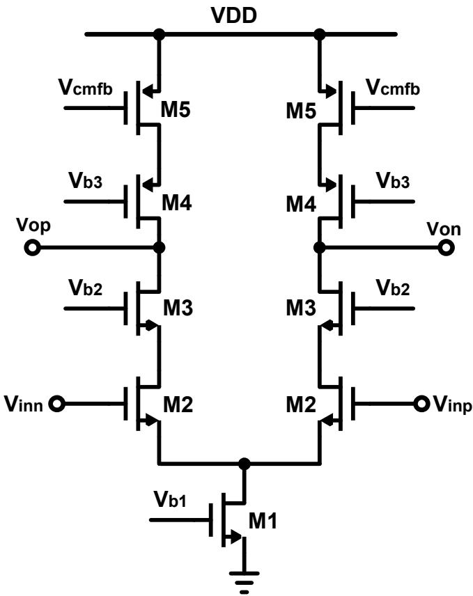
Fig. 3-7. NMOS-input cascode single-stage opamp for the second integrator.
