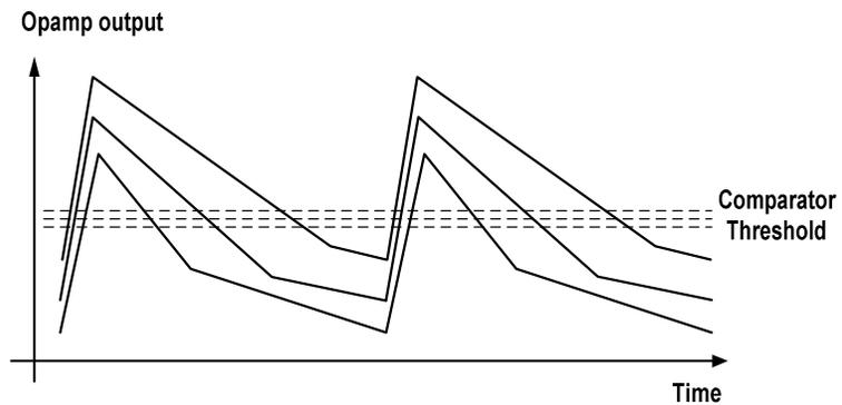
Fig. 6-4. Opamp output of the tuning circuit. Top curve: slow condition (both R and C have a +25% error), middle curve: typical condition (no errors in R and C), bottom curve: fast condition (both R and C have a -25% error).
