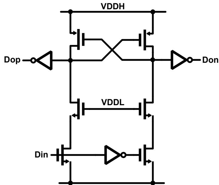
Fig. 3-15. Circuit diagram of the LHVT.
