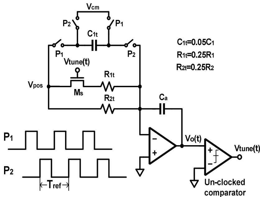
Fig. 6-3. SR tuning circuit.
