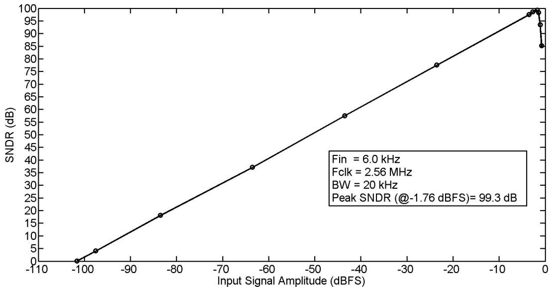
Fig. 4-5. SNDR versus input amplitude.
