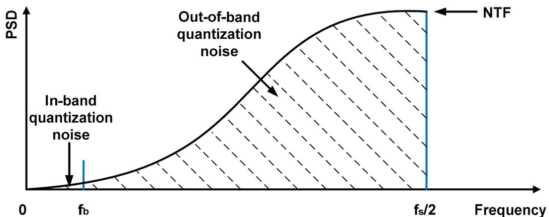
Fig. 2-3. High-pass function from the NTF of the low-pass delta-sigma modulator.
