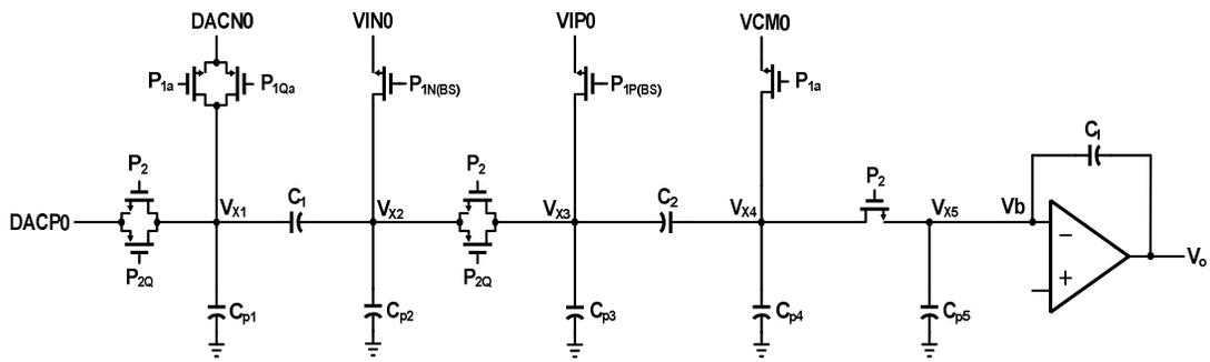
Fig. 5-6. Proposed low-power parasitic-sensitive SC integrator.
