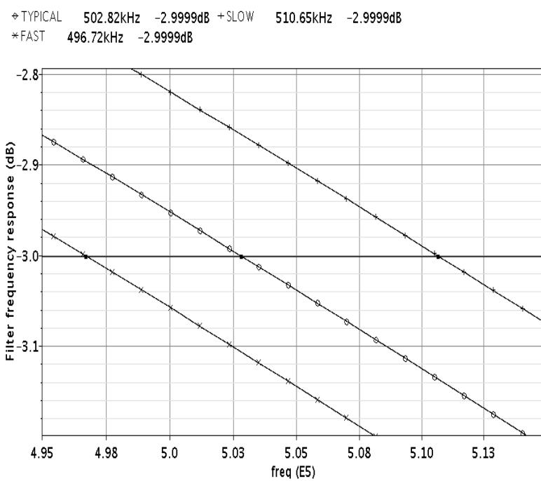
Fig. 6-7. Filter cutoff frequency variation.
