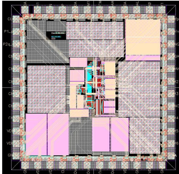
Fig. 3-18. Layout of the proposed ADC.
