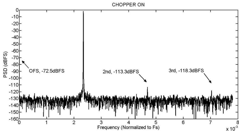
Fig. 4-9 PSD of the modulator output within the signal bandwidth (Chopper on).
