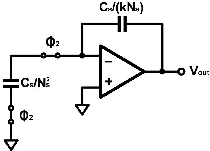
Fig. 5-4. Low-power SC integrator in the integration phase.
