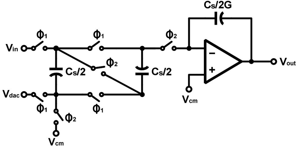
Fig. 5-2. Low-power parasitic-sensitive SC integrator.
