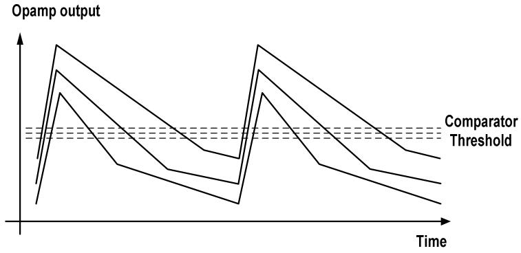
Fig. 6-4. Opamp output of the tuning circuit. Top curve: slow condition (both R and C have a +25% error), middle curve: typical condition (no errors in R and C), bottom curve: fast condition (both R and C have a -25% error).
