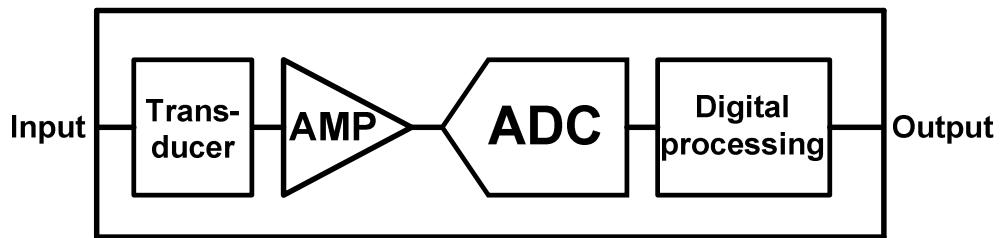
Figure 1-1. Analog-front-end composition.
