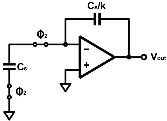
Fig. 5-3. Conventional SC integrator in the integration phase.
