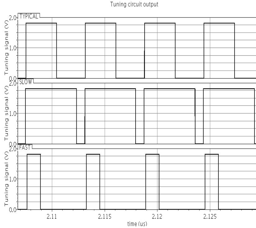
Fig. 6-5. Tuning signal with variable duty cycle.
