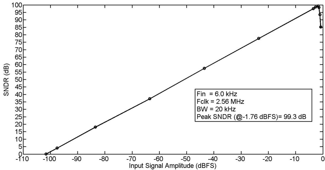
Fig. 4-5. SNDR versus input amplitude.
