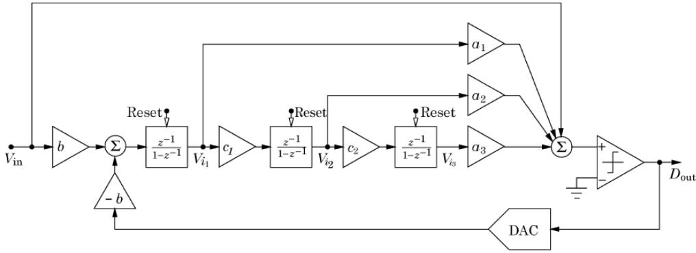
Fig. 2-4. Block diagram of a high-order feed-forward incremental ADC.
