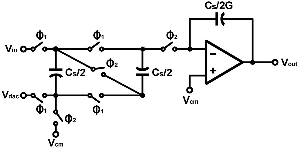
Fig. 5-2. Low-power parasitic-sensitive SC integrator.
