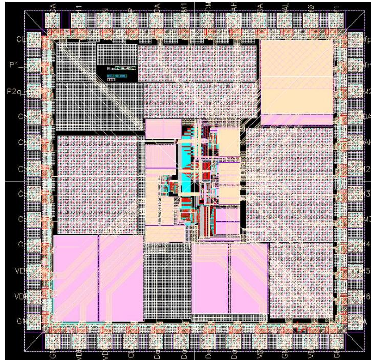
Fig. 3-18. Layout of the proposed ADC.
