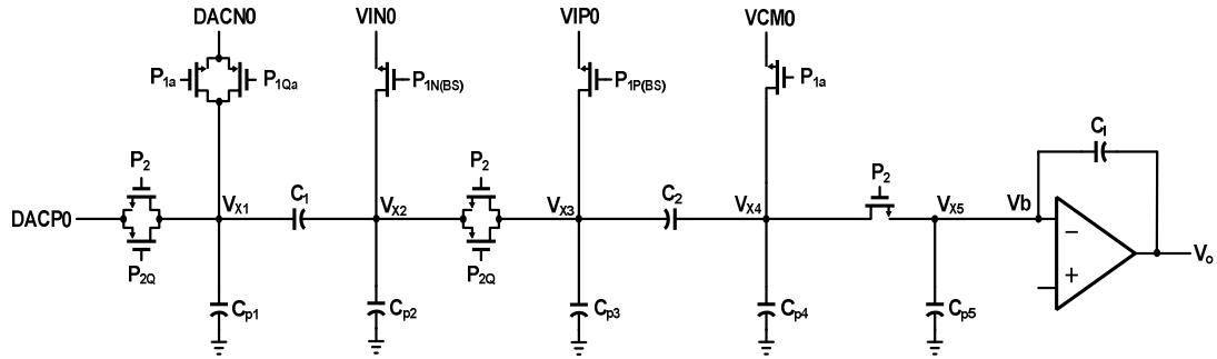
Fig. 5-6. Proposed low-power parasitic-sensitive SC integrator.
