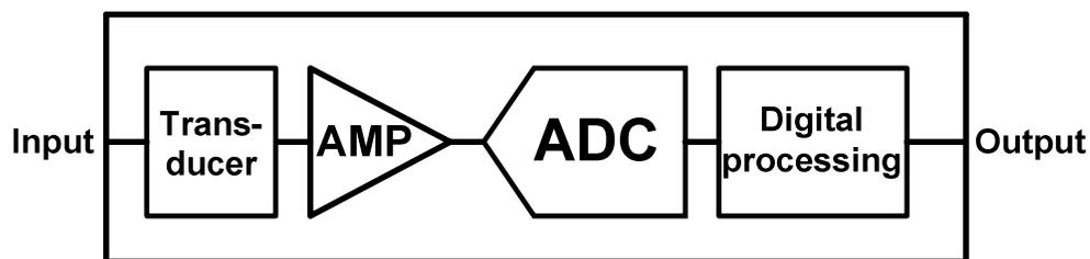
Figure 1-1. Analog-front-end composition.
