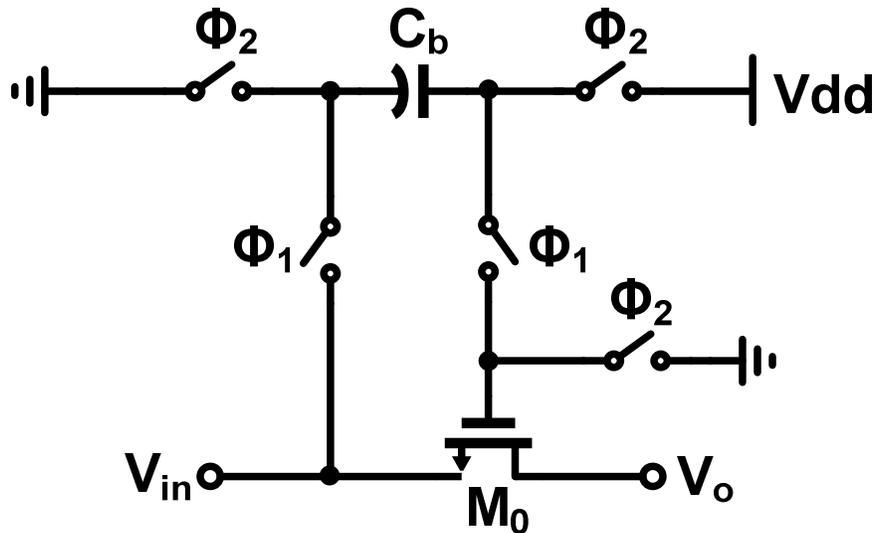
Fig. 3-3. Principle of bootstrapping technique.
