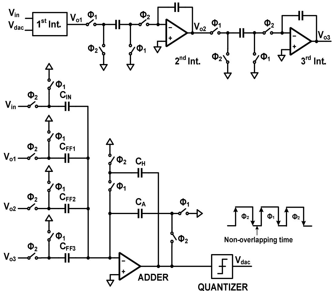
Fig. 5-7. Modified low-distortion  $\Delta\Sigma$  ADC.
