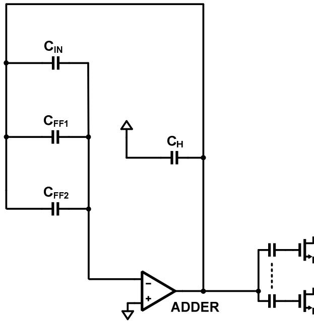
Fig. 3-9. The capacitive loading of the DCT adder during phase  $\Phi_1$ .
