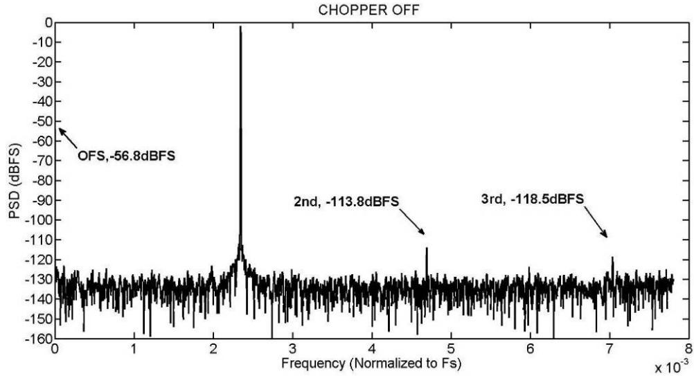
Fig. 4-8 PSD of the modulator output within the signal bandwidth (Chopper off).
