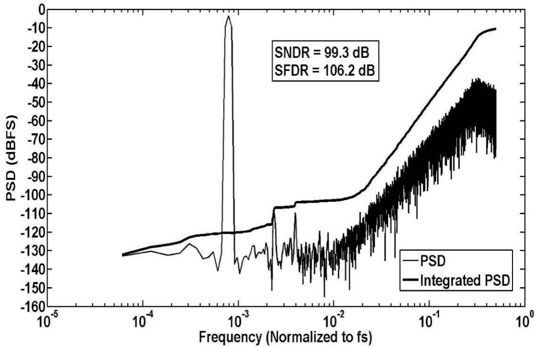
Fig. 5-8. PSD of the modulator output.
