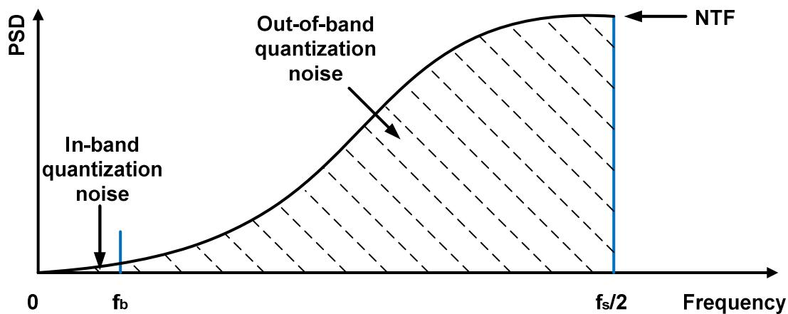
Fig. 2-3. High-pass function from the NTF of the low-pass delta-sigma modulator.
