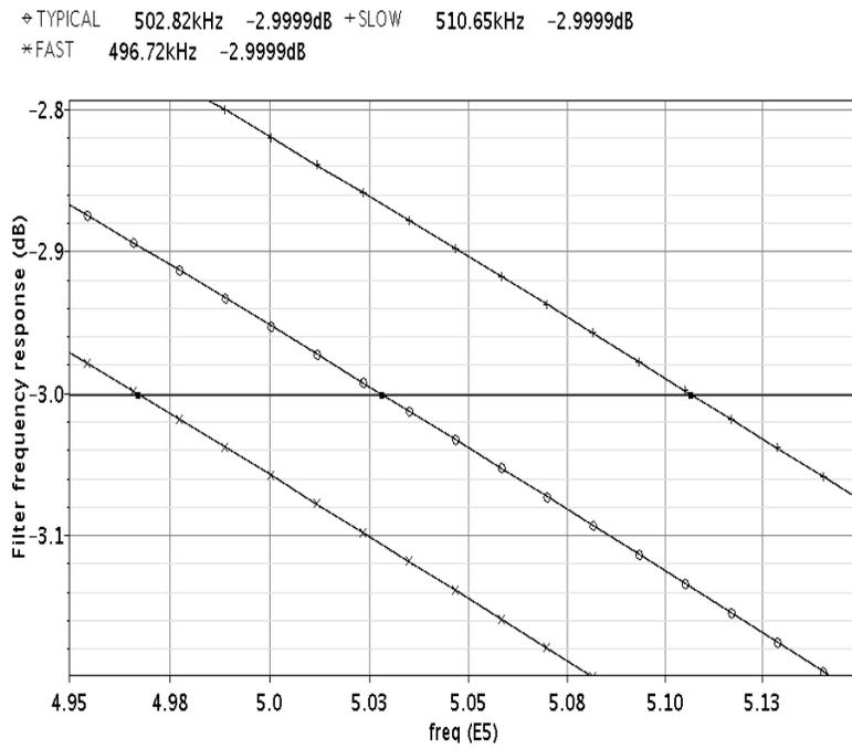
Fig. 6-7. Filter cutoff frequency variation.
