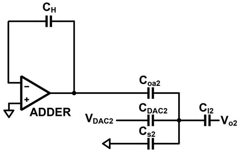
Fig. 3-8. The capacitive loading of the DCT adder during phase  $\Phi_2$ .
