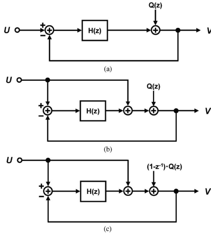
Fig. 2-8. Principle of noise-coupling technique: (a) Conventional delta-sigma modulator. (b) Low-distortion delta-sigma modulator. (c) Low-distortion delta-sigma modulator with first-order noise-coupling.
