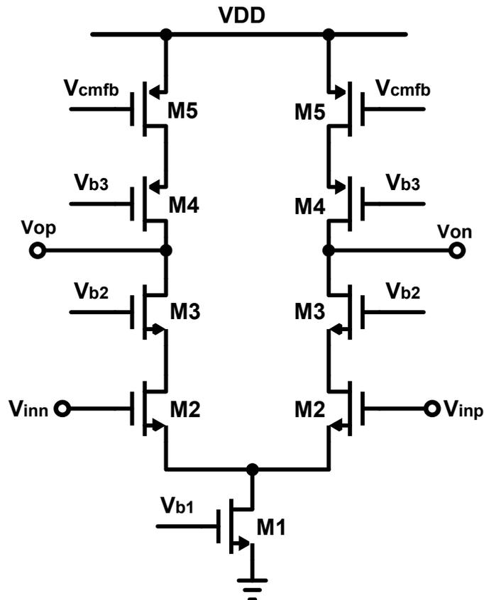
Fig. 3-7. NMOS-input cascode single-stage opamp for the second integrator.
