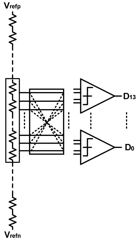
Fig. 3-10. Circuit diagram of the quantizer.
