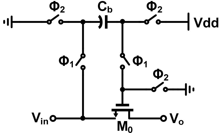
Fig. 3-3. Principle of bootstrapping technique.
