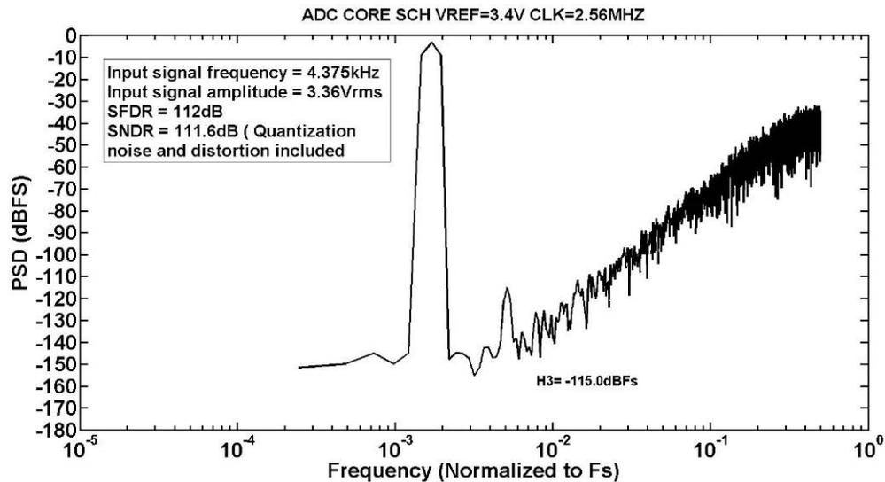
Fig. 3-19. Simulated PSD of the modulator output.
