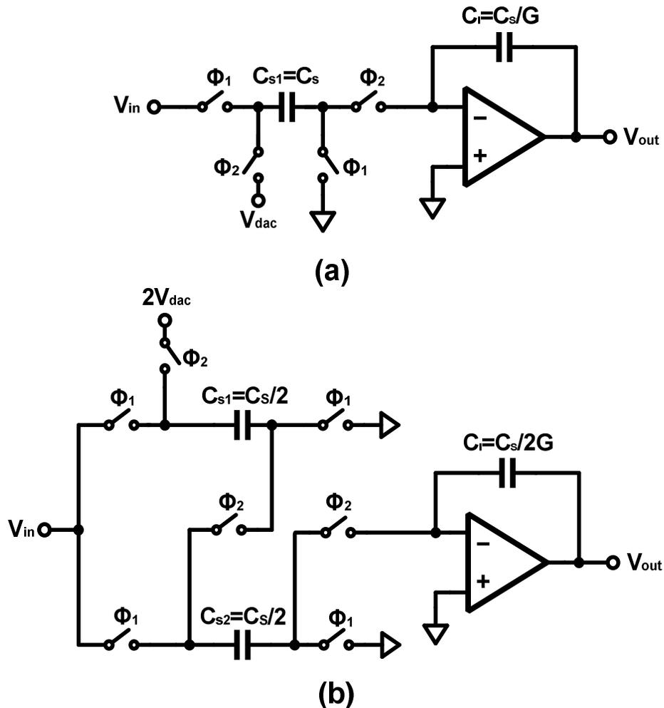
Fig. 5-1. (a) Conventional SC integrator. (b) Nilchi-Johns integrator.
