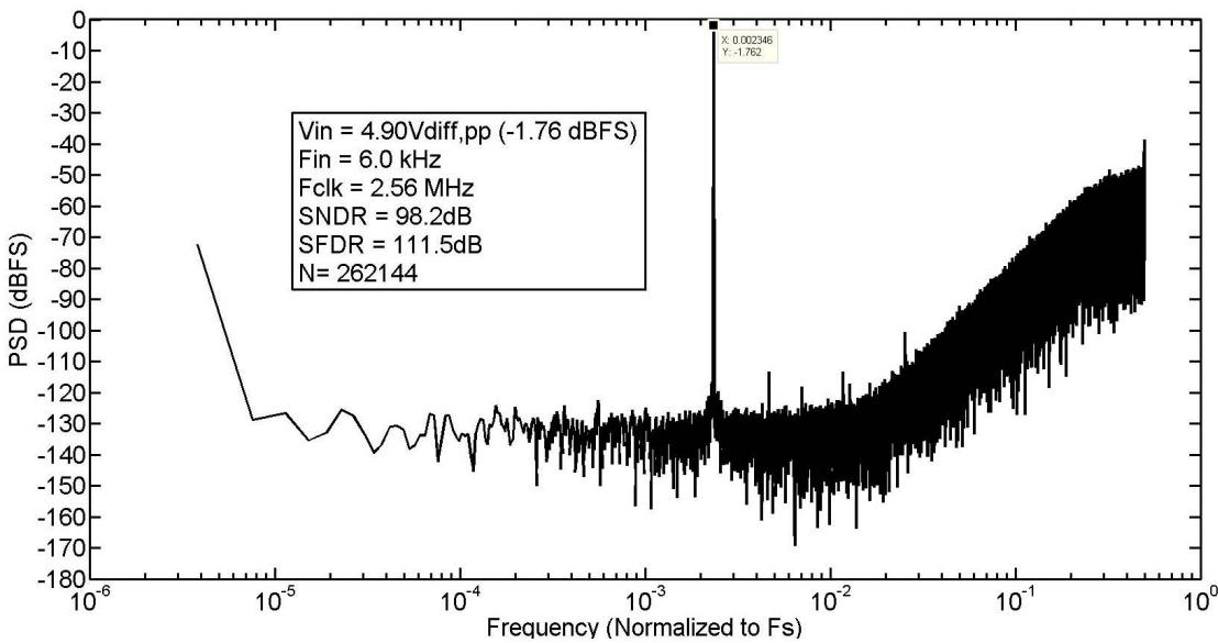
Fig. 4-7. PSD of the modulator output (Chopper on).
