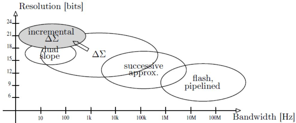
Figure 1-2. Applications of A/D converter structures for typical resolution and bandwidth requirement
