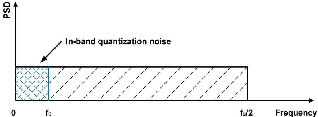
Fig. 2-1. PSD reduction of quantization noise by using oversampling technique.
