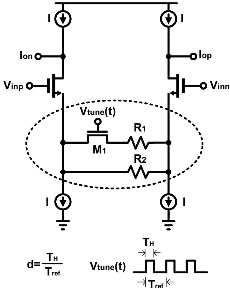
Fig. 6-1. Gm cell with SR source degeneration.
