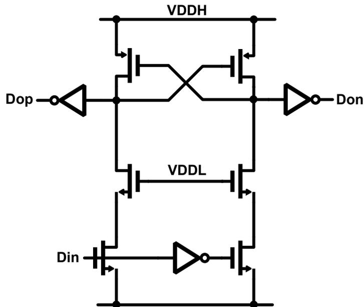
Fig. 3-15. Circuit diagram of the LHVT.
