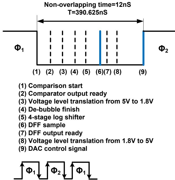
Fig. 3-17. DWA logic timing.
