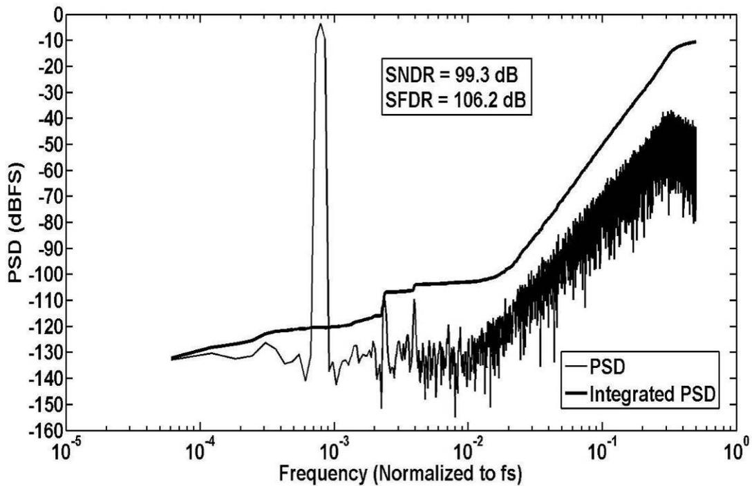
Fig. 5-8. PSD of the modulator output.
