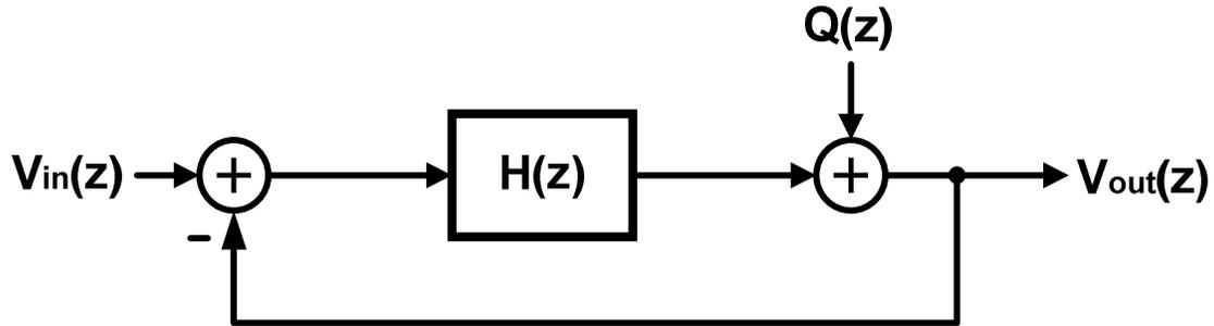
Fig. 2-2. General single feedback delta-sigma modulator topology.
