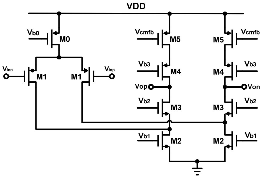
Fig. 3-4. PMOS-input folded cascode single-stage operational amplifier.
