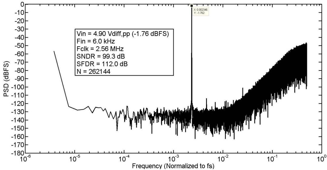
Fig. 4-6. PSD of the modulator output (Chopper off).
