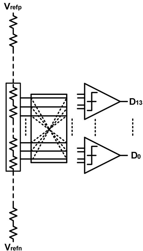
Fig. 3-10. Circuit diagram of the quantizer.
