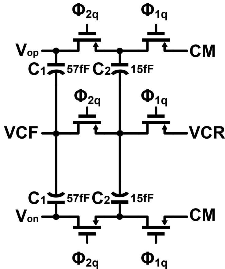
Fig. 3-5. Switched-capacitor CMFB circuit for the opamp of the first integrator.
