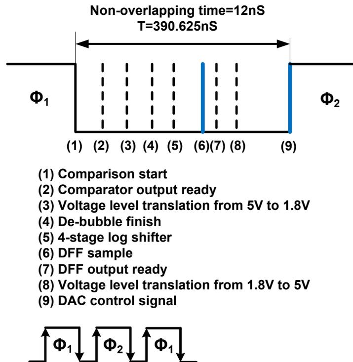
Fig. 3-17. DWA logic timing.
