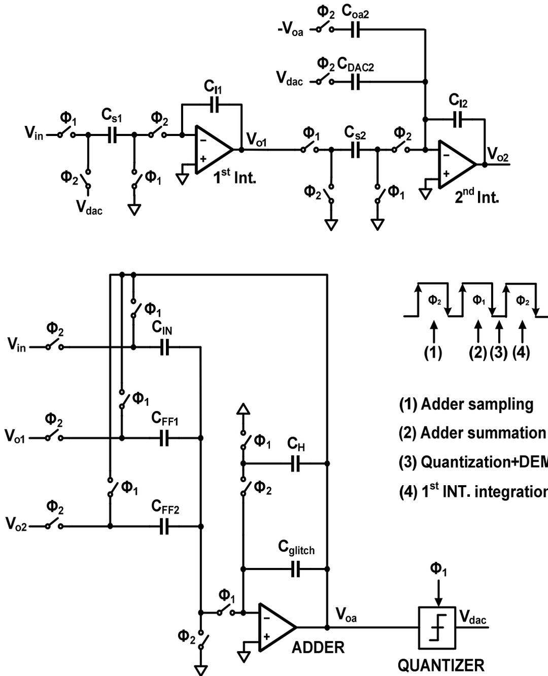
Fig. 2-6. Circuit diagram of the proposed delta-sigma ADC.
