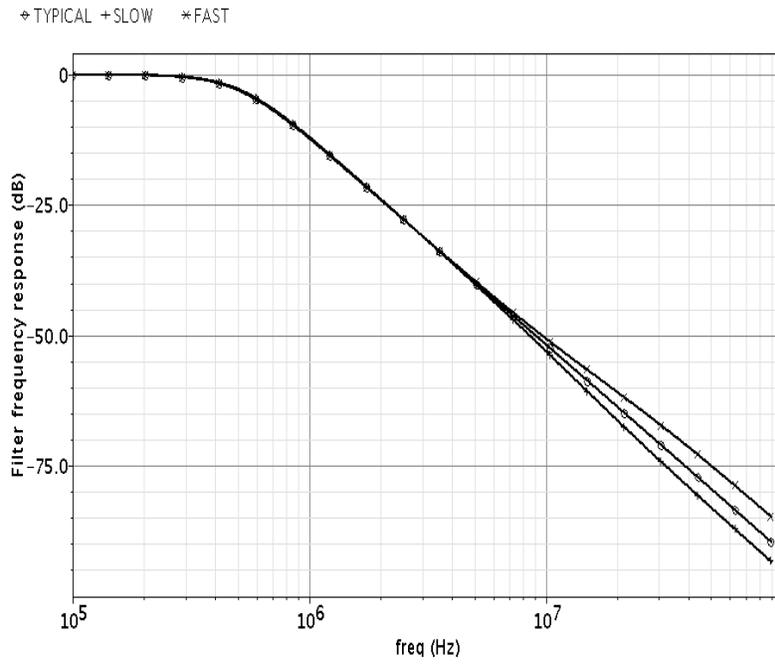
Fig. 6-6. Tuned filter frequency responses under different conditions. Top curve: fast condition, middle curve: typical condition, bottom curve: slow condition.
