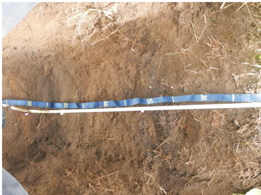
Figure 9. Pit dug in the restored pasture of Curi-cancha. The total depth of the pit was 108 cm. Contact with the root restrictive clay was made from 99-108 cm.
