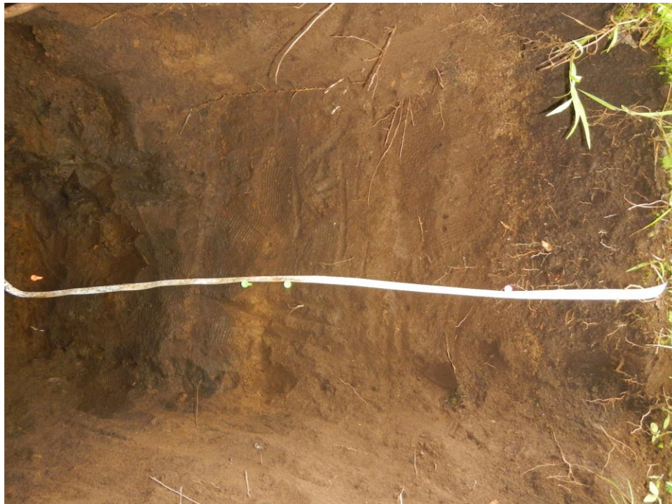
Figure 8. Pit dug in the restored farm of Finca Rodriguez. The total depth of the pit was 108 cm. Contact was not made with the root restrictive clay later
