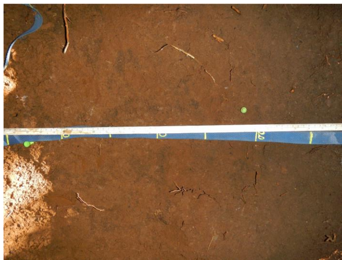
Figure 12. The first pit dug at La Calandria. The total depth of the pit was 72 cm. Contact with the root restrictive clay layer was made from 72-105 cm.
