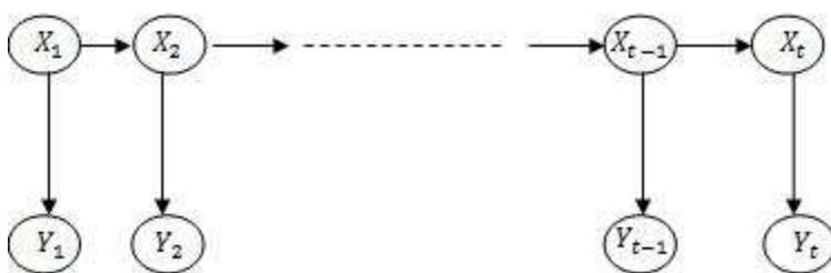
Figure 4.2. Unrolling the hidden Markov model in time slice. X can take values from S . Y can take any values in V .
