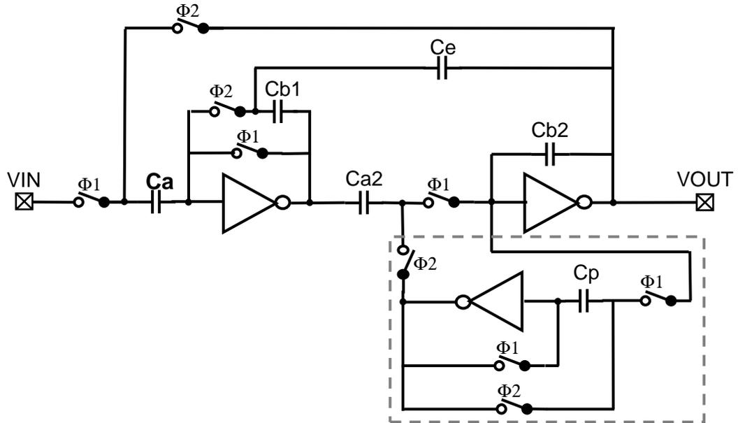
Figure 2.8. The e-damping biquad LPF based on inverters
