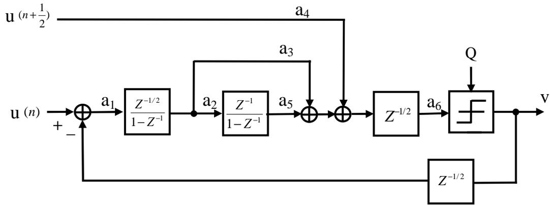
Figure 5.2. Inverter based second order delta-sigma ADC topology
