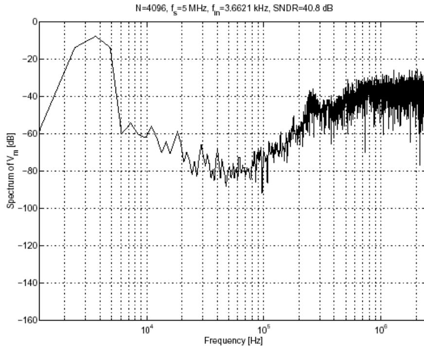
Figure 6.3. FFT result of the transistor level simulation
