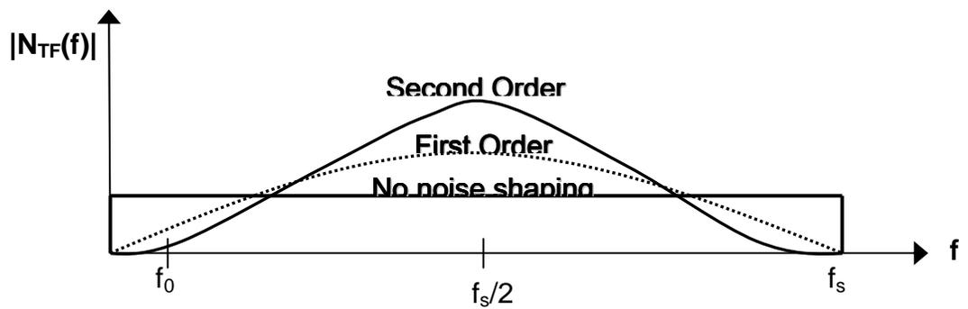
Figure 4.5. Some different noise-shaping transfer functions [12]
