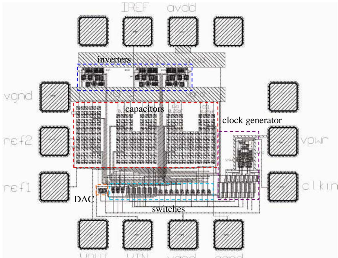
Figure 7.3. Inverter based second-order delta-sigma modulator layout
