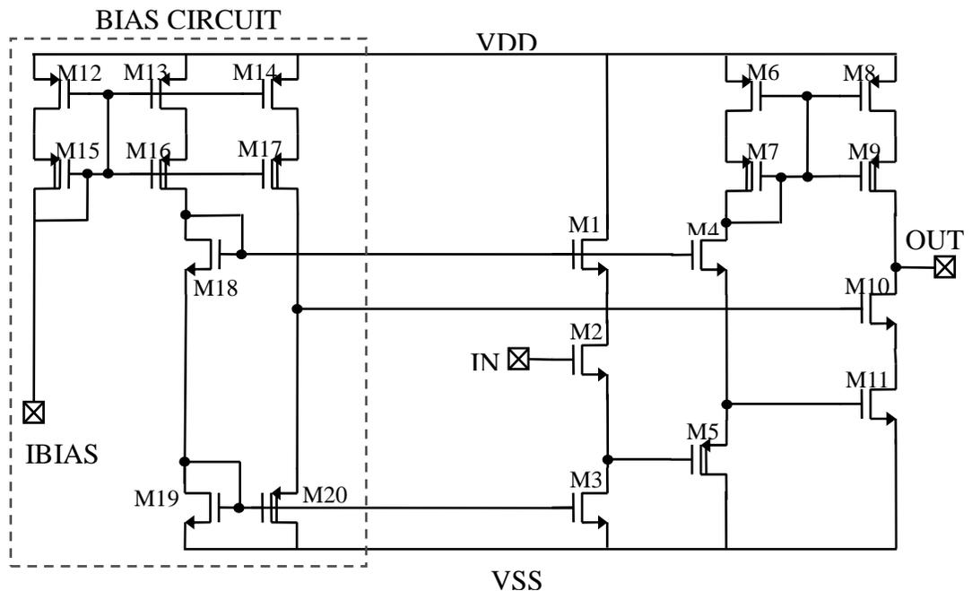
Figure 3.1. Inverter design based on cascode structure
