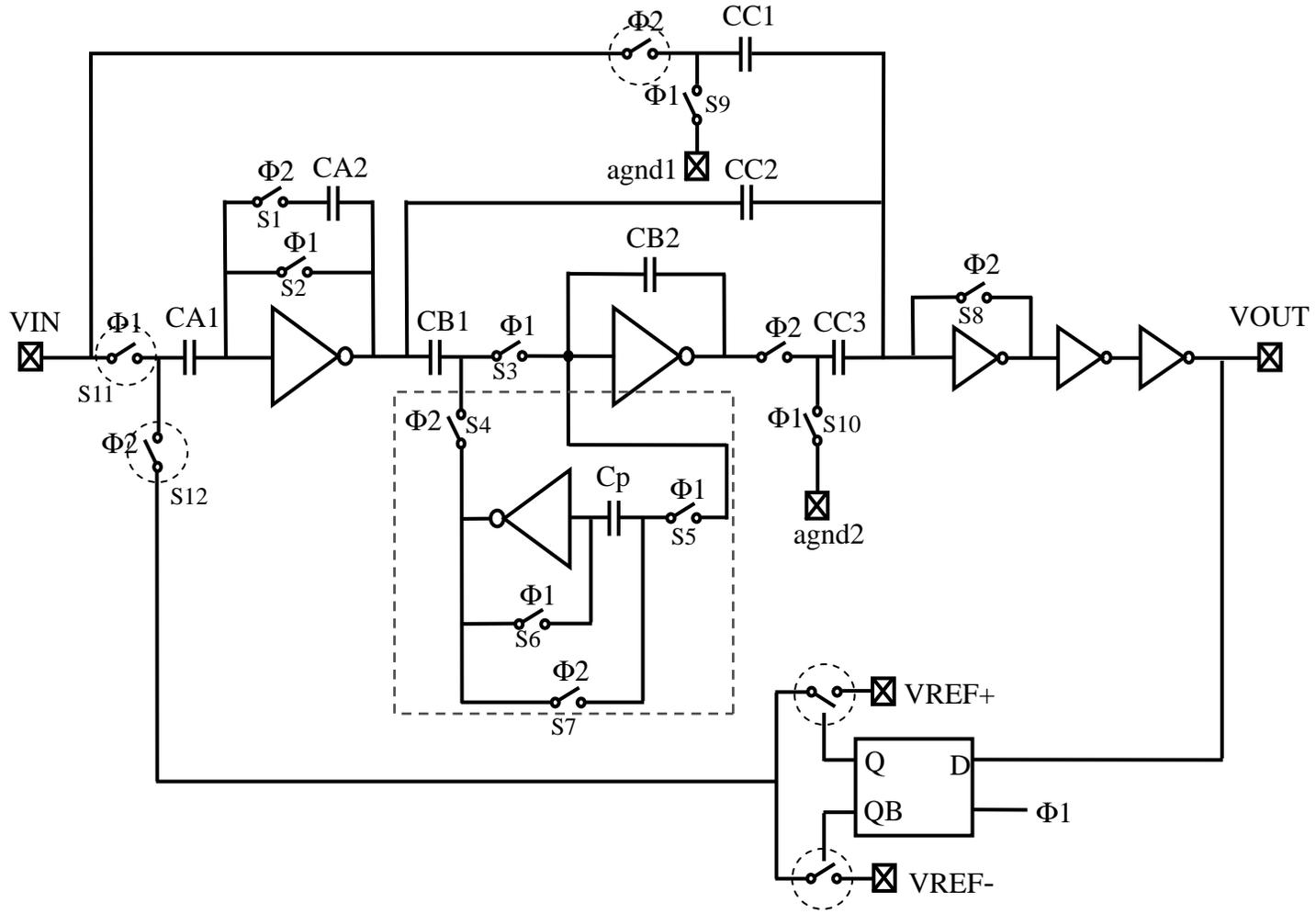
Figure 5.6. Circuit level design of inverter based second order delta-sigma ADC
