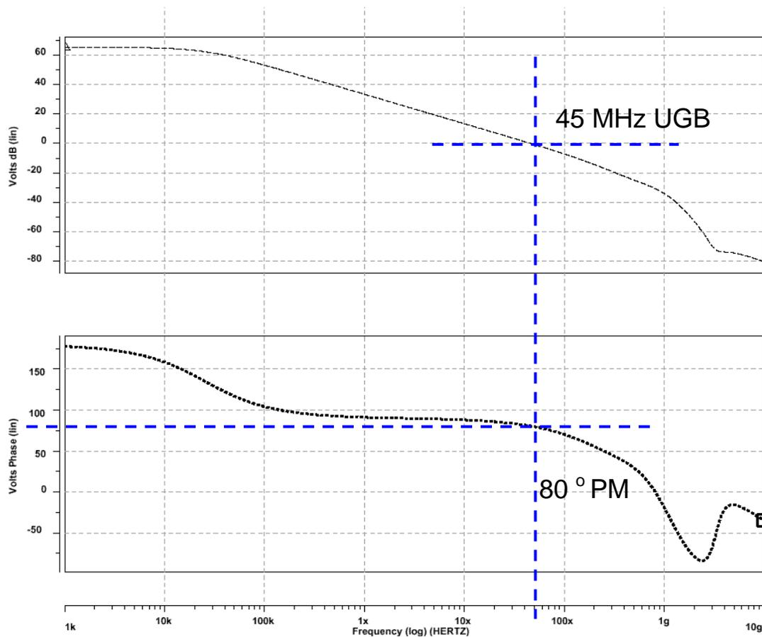
Figure 3.3. AC characteristic of the inverter
