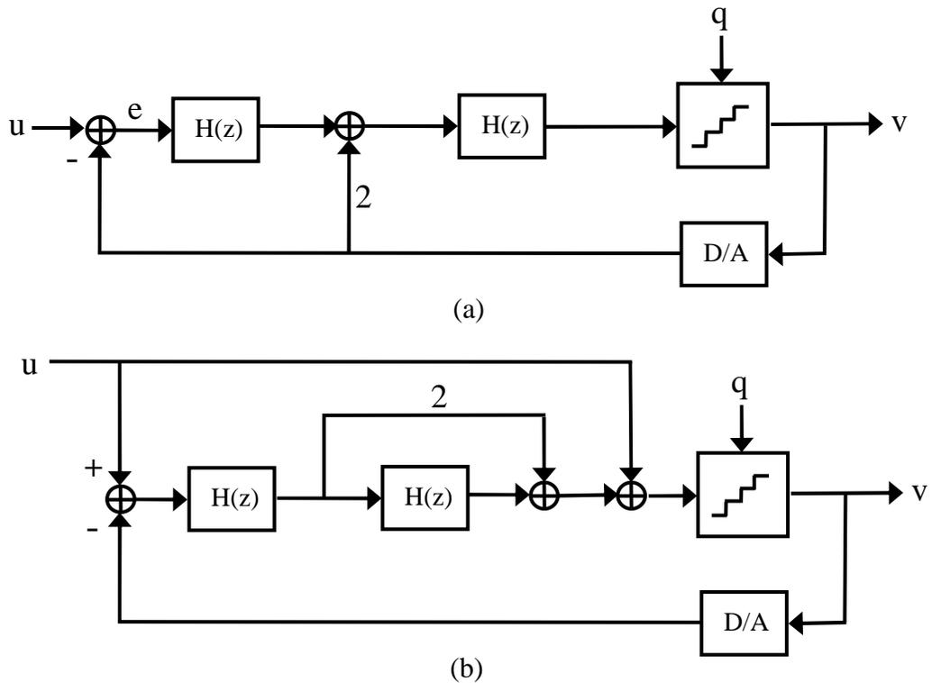
Figure 5.1. (a) Traditional Topology, (b) Reduced distortion topology
