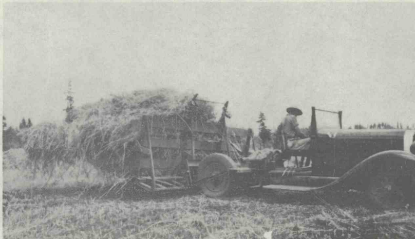
Figure 5. Auto buck rake with load in transport position.
