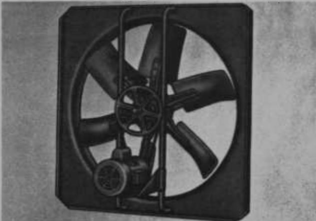
Vertically-mounted fan can be ducted for either "whole house" ventilation or flushing air from attic only. These units come in sizes from 16 inches to 42 inches in diameter and are usually belt-driven by 1/4 to 1 hp continuous-duty motors. CFM ratings should be at 1/10 (0.10) or 1/8 (0.125) inch static pressure.
