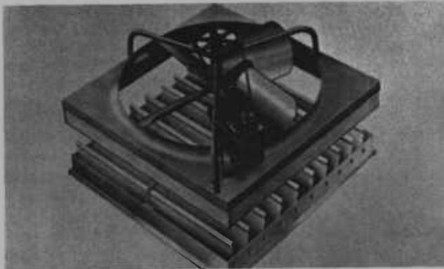
Horizontally-mounted ceiling fan with accompanying shutter can be used only for "whole house" ventilation. Specifications are similar to vertically-mounted units. Vertically-mounted motor and fan must be equipped with thrust or ball bearings. Shutter area should be carefully covered during winter months with vapor barrier-protected insulation to reduce heat loss and moisture migration to attic.
