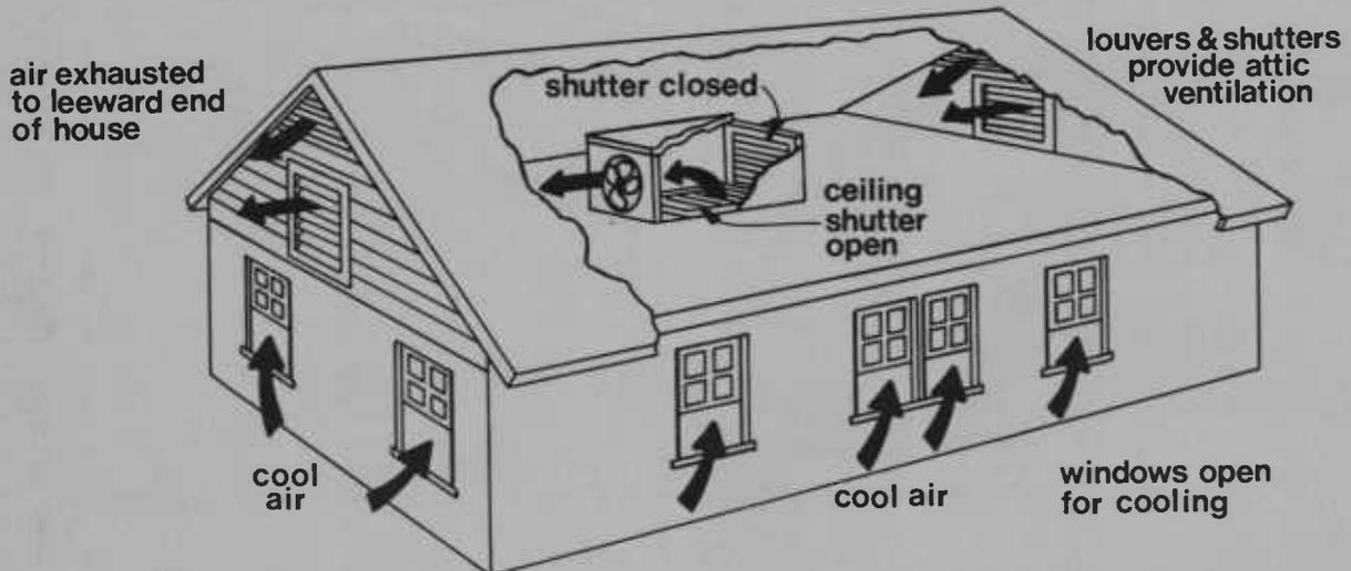
"Whole house" ventilation system draws cool outdoor air into living area of house through open windows and exhausts warm indoor air through attic vents, thus also flushing hot air from
