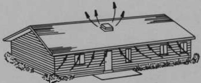
Attic area ventilation flushes hot air out of attic and replaces it with cooler, outdoor air. No air is drawn through living area.
