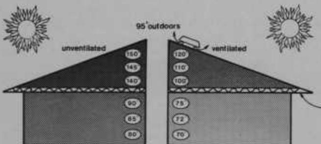
Unventilated attics can build up temperatures reaching 150° F during a hot, sunny day. This trapped heat radiates to rooms below, creating uncomfortably hot conditions and imposing heavy cooling loads on air conditioners.
