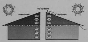
Unventilated attics can build up temperatures reaching 150° F during a hot, sunny day. This trapped heat radiates to rooms below, creating uncomfortably hot conditions and imposing heavy cooling loads on air conditioners.
