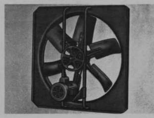
Vertically-mounted fan can be ducted for either "whole house" ventilation or flushing air from attic only. These units come in sizes from 16 inches to 42 inches in diameter and are usually belt-driven by 1/4 to 1 hp continuous-duty motors. CFM ratings should be at 1/10 (0.10) or 1/8 (0.125) inch static pressure.
