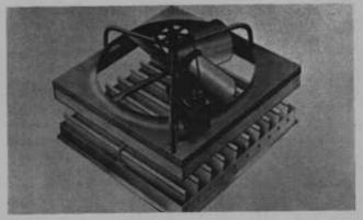
Horizontally-mounted ceiling fan with accompanying shutter can be used only for "whole house" ventilation. Specifications are similar to vertically-mounted units. Vertically-mounted motor and tan must be equipped with thrust or ball bearings. Shutter area should be caretully covered during winter months with vapor barrier-protected insulation to reduce heat loss and moisture migration to attic.
