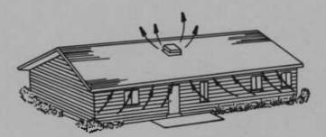
Attic area ventilation flushes hot air out of attic and replaces it with cooler, outdoor air. No air is drawn through living area.
