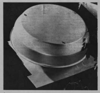
Roof-mounted attic fan should be centered on roof, near peak. These units fit between rafters, come in sizes from 500 to 1800 CFM (rated at 0.03 inch static pressure) with 1/15 to 1/4 hp slow-speed (1025-1550 RPM) motors. Hood is molded fiberglass, high impact thermostyrene plastic or aluminum. Hood has built-in insect screen and is wind, rain and snow proof.
