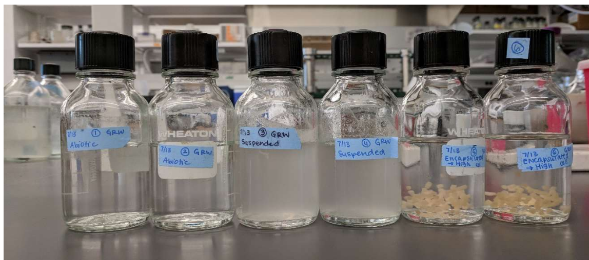
Figure 12. Long-term CoC transformation reactors. Abiotic, Suspended ATCC 21198, and Gellan Gum Encapsulated ATCC 21198 in duplicate reactors, left to right, respectively.
