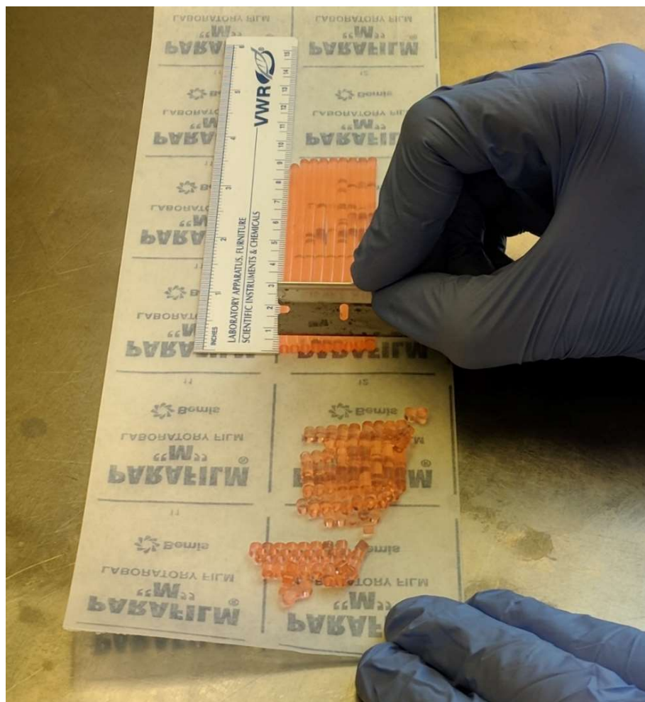
Figure 10. Manual cutting of gellan gum strands into 2mm right cylinders for experimental use. Orange dye was added such that GG pre-gel solution could be better visualized.
