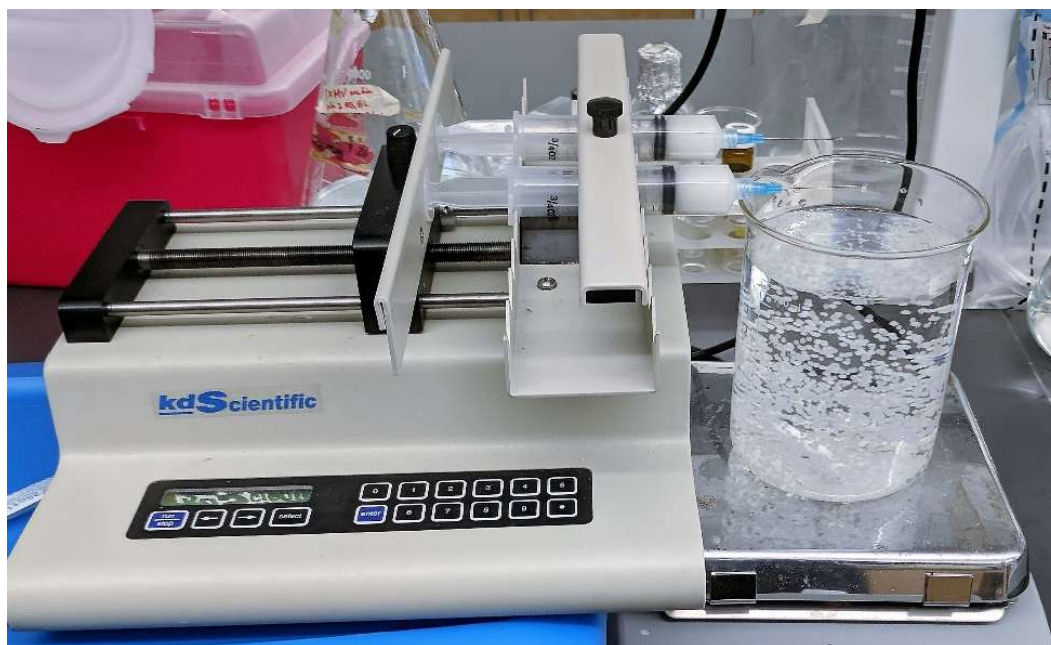
Figure 4. Calcium-alginate macro-bead formation by extrusion into crosslinking solution.
