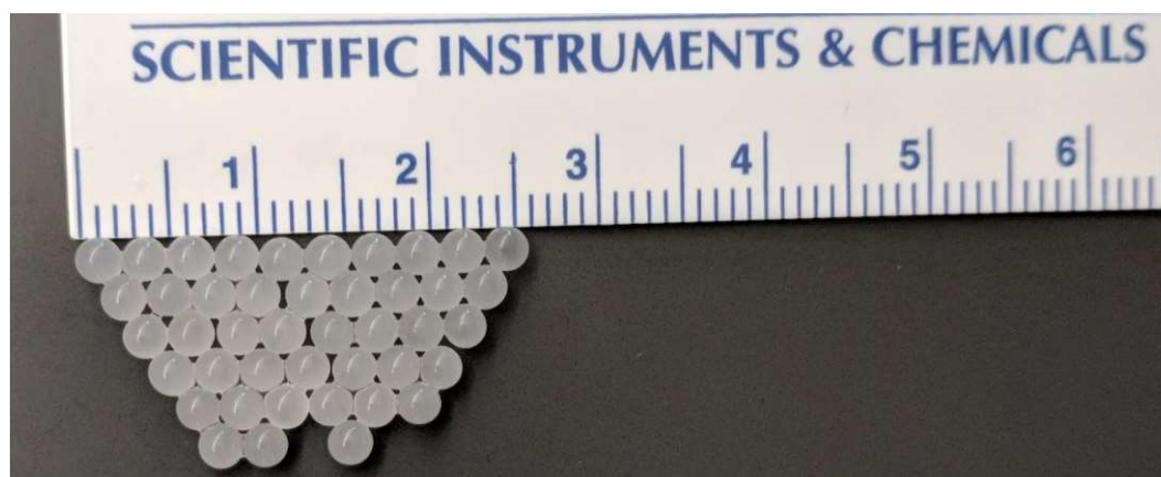
Figure 5. Gelated alginate macro-beads with a VWR ruler for scale.
