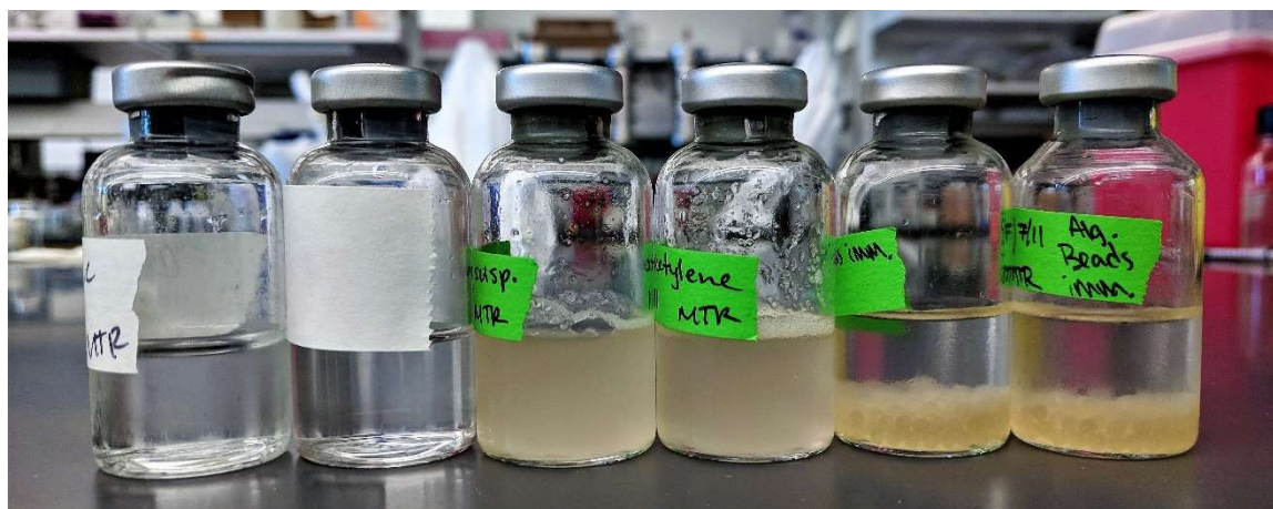
Figure 11. Short-term batch substrate (IB) utilization kinetic tests. (Left two bottles) Abiotic (Middle two bottles) Suspended cells. (Right two bottles) Encapsulated cells.
