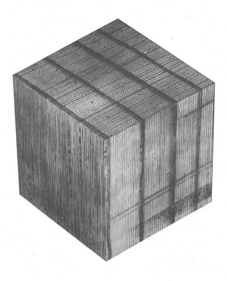
How a small cube of redwood, about 1/4 inch on each side, looks under the compound microscope.
