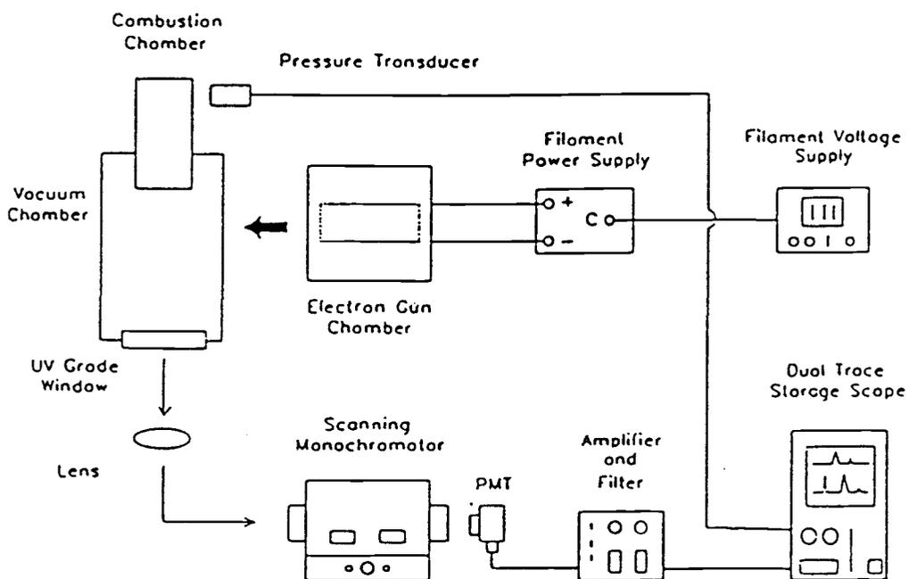
(b) Instrumentation for transient measurements.
