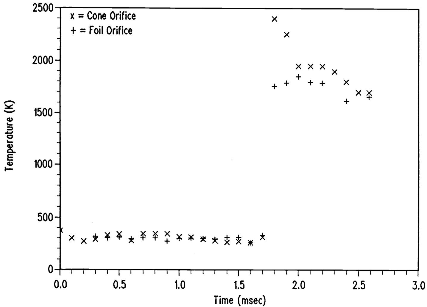
Fig. 26 Predicted temperatures during combustion.
