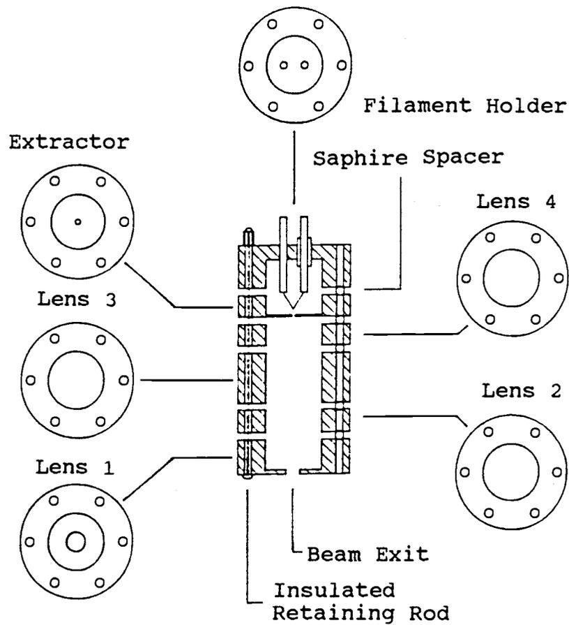
Fig. 3 Diagram of an electron gun.
