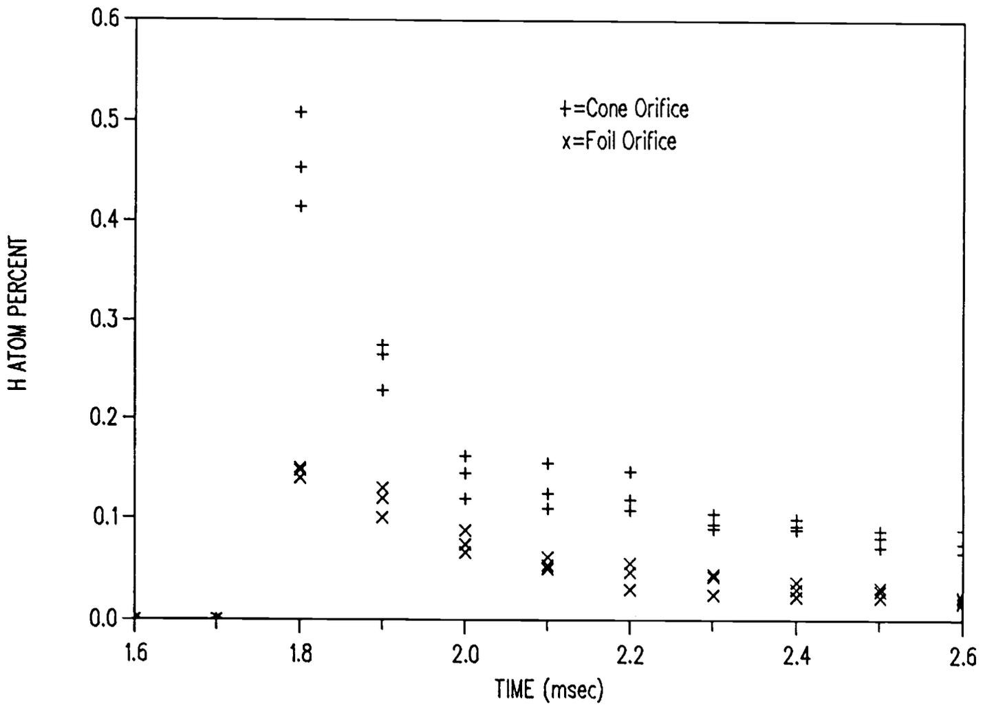
Fig. 29 Hydrogen mole fractions during combustion.
