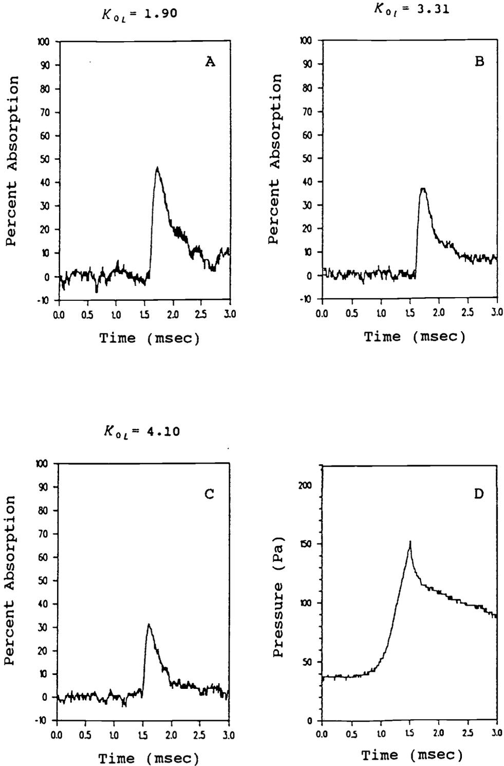
Fig. 27 Resonant absorption by atomic hydrogen and flow tube pressure for foil sampling orifice experiments.
