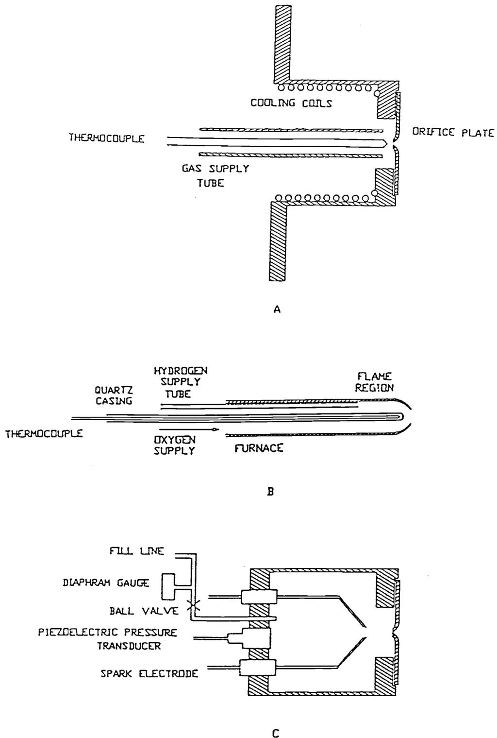
Fig. 4 Diagram of various source arrangements. (a) Insert with inner tube for high temperature sampling. (b) Burner for sampling from lean combustion. (c) Combustion chamber for transient experiments.
