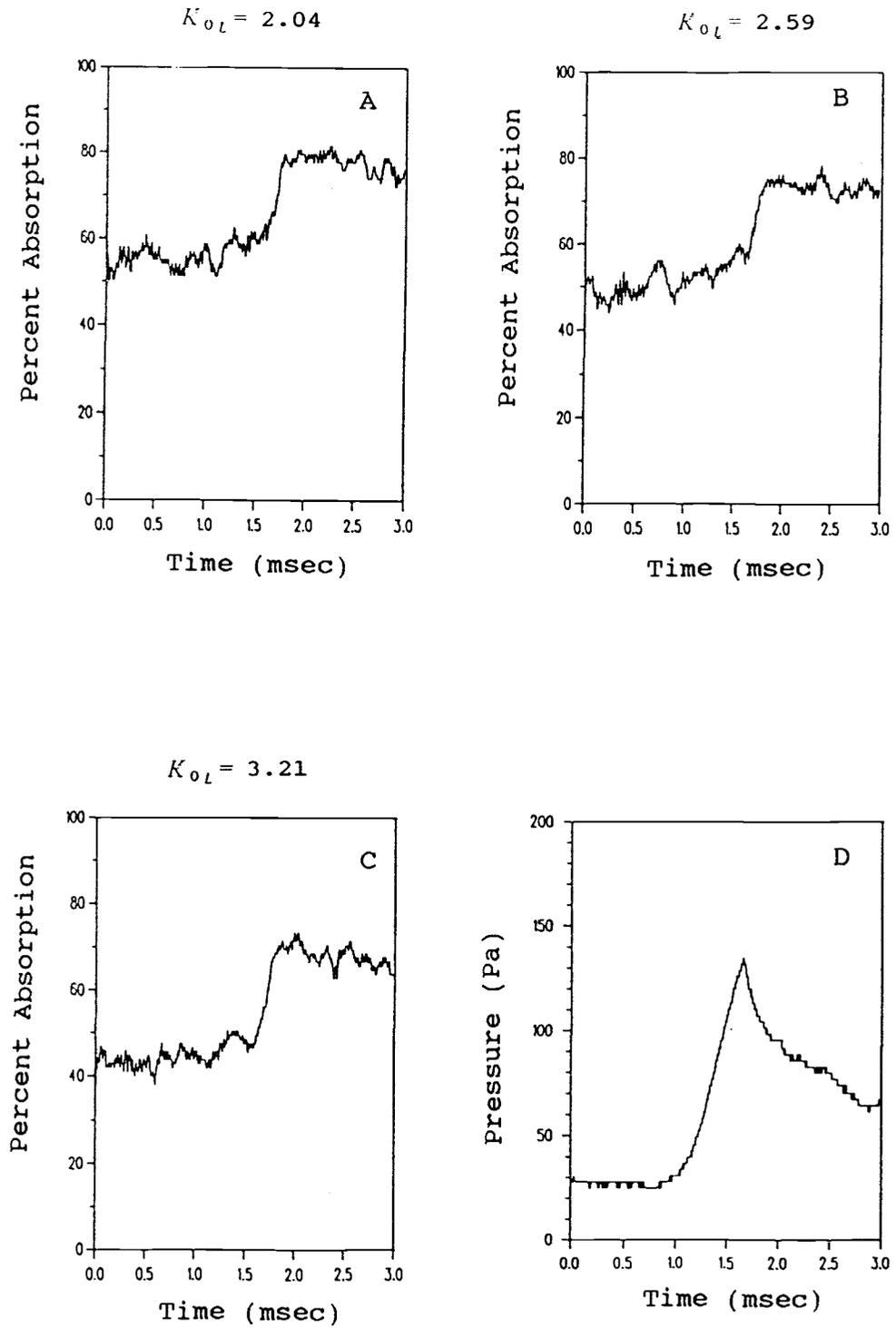
Fig. 25 Resonant absorption by krypton and flow tube pressure for conical sampling orifice experiments.
