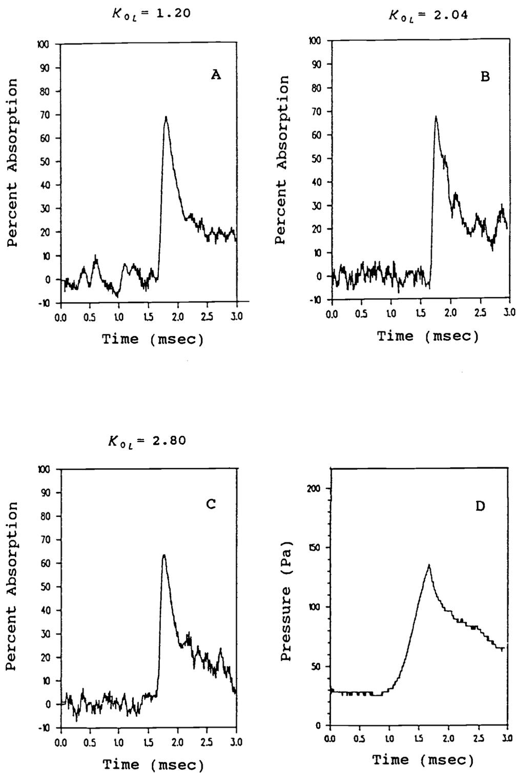
Fig. 28 Resonant absorption by atomic hydrogen and flow tube pressure for conical sampling orifice experiments.
