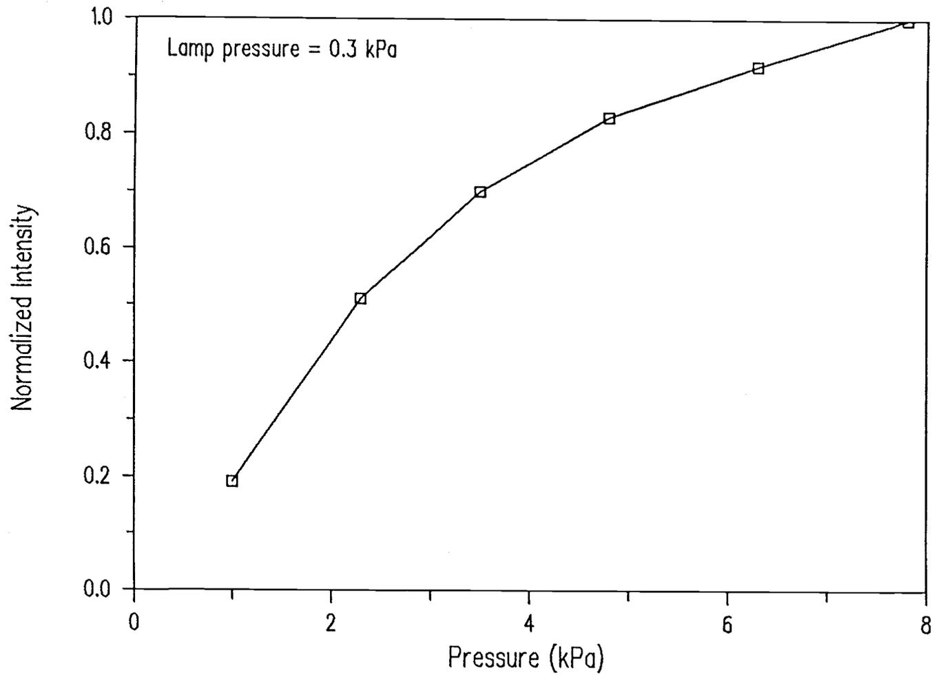
Fig. 16 Variations of Lyman- $\alpha$  signal strength with emitter gas supply pressure.
