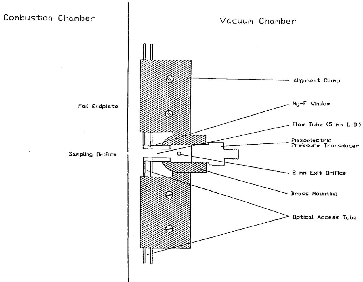
Fig. 12 Flow tube for absorption measurements.
