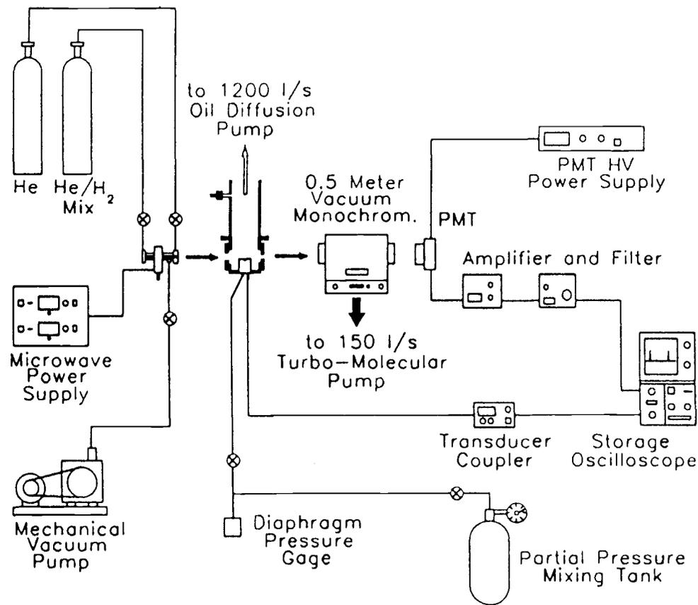
Fig. 13 Schematic diagram of the DSARAS instrumentation.
