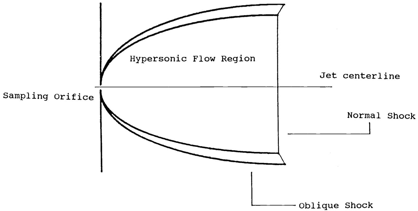
Fig. 1 Structure of a free jet.
