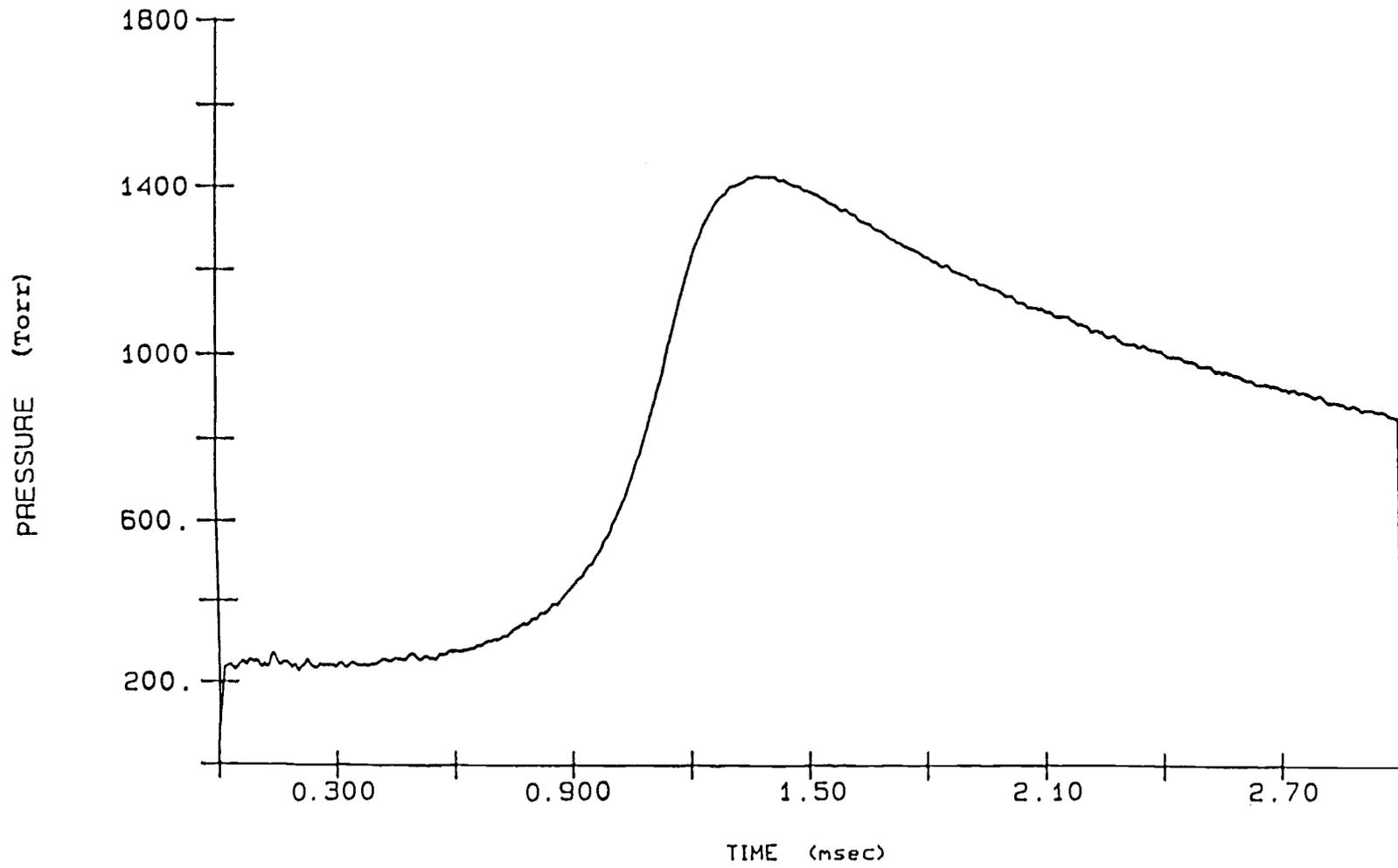
Fig. 8 Combustion chamber pressure during transient combustion.
