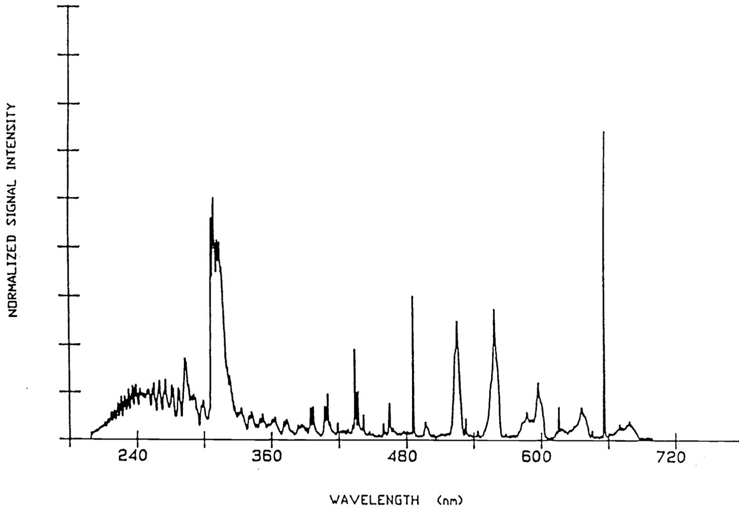
Fig. 7 DSEIF spectrum of lean hydrogen/oxygen combustion.
