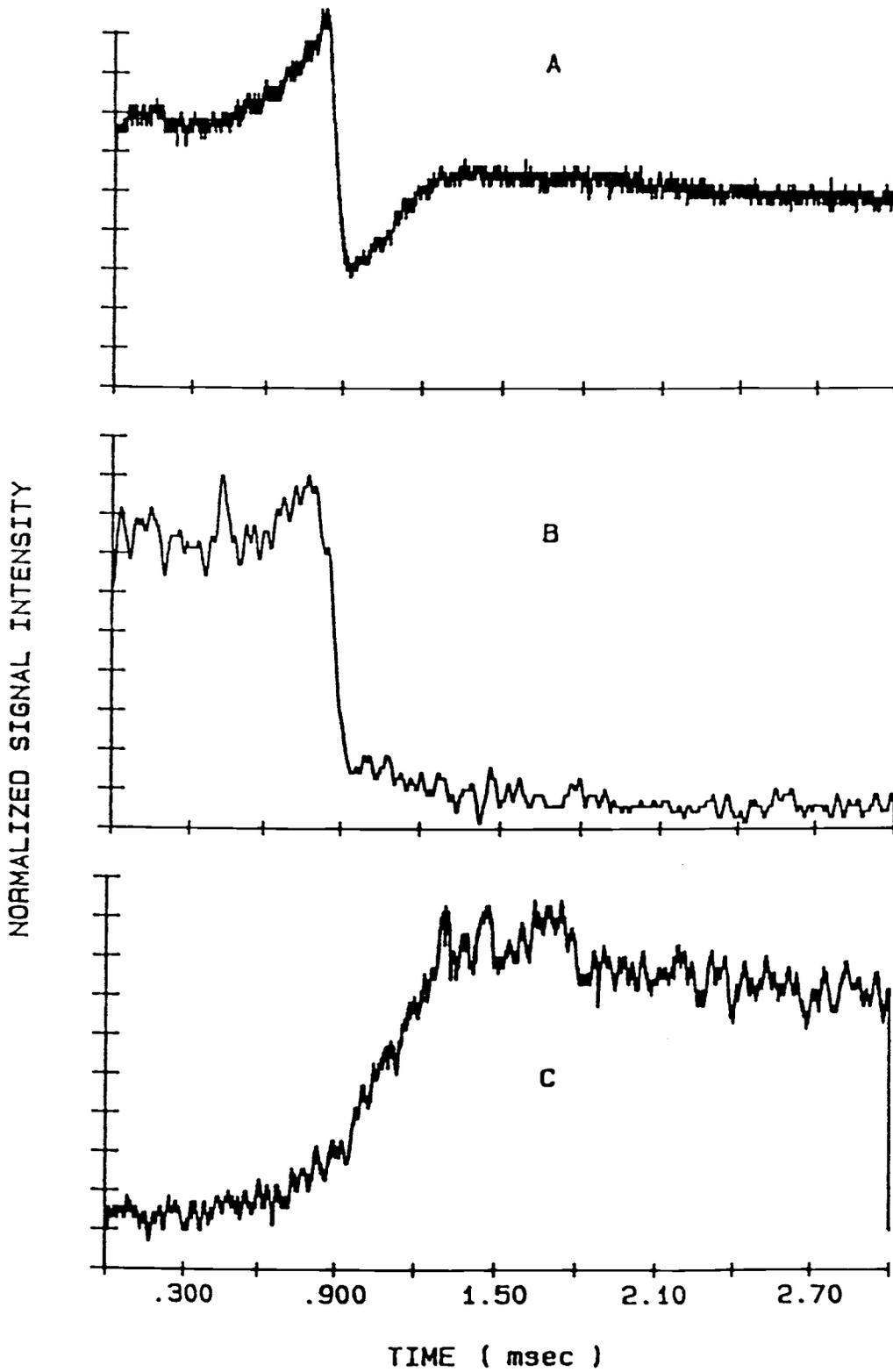
Fig. 9 Emission intensity versus time. Curve (a) was recorded at 391.1 nm, curve (b) at 559.7 nm, and curve (c) at 307.5 nm.
