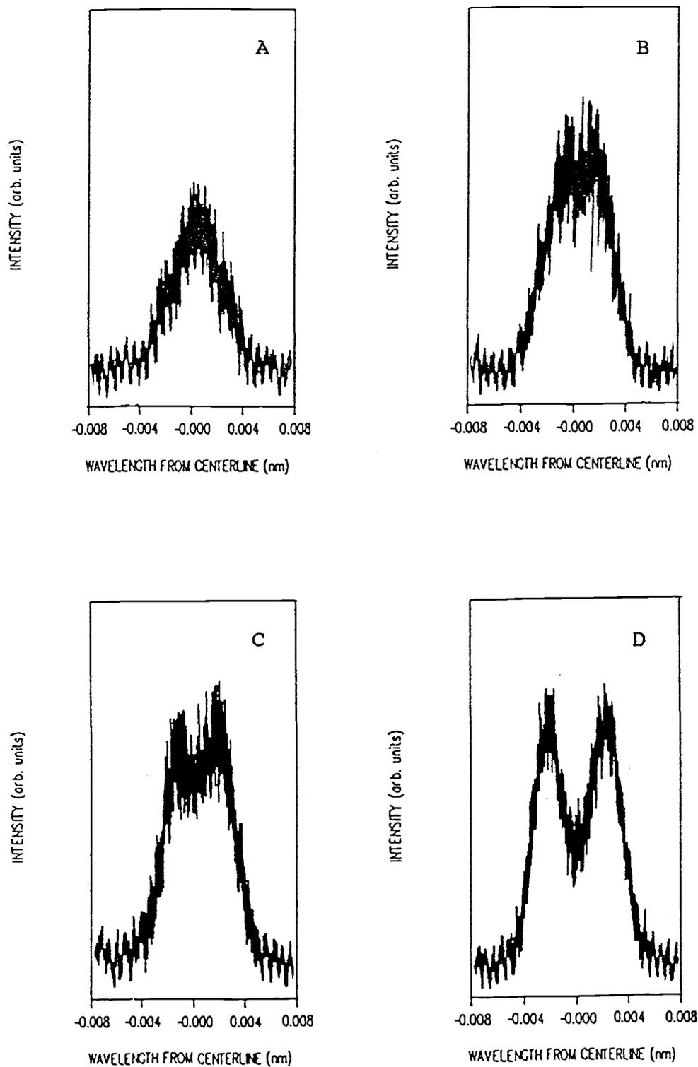
Fig. 18 Spectra recorded from high resolution scans of the 47th order hydrogen Lyman- $\alpha$  line.
