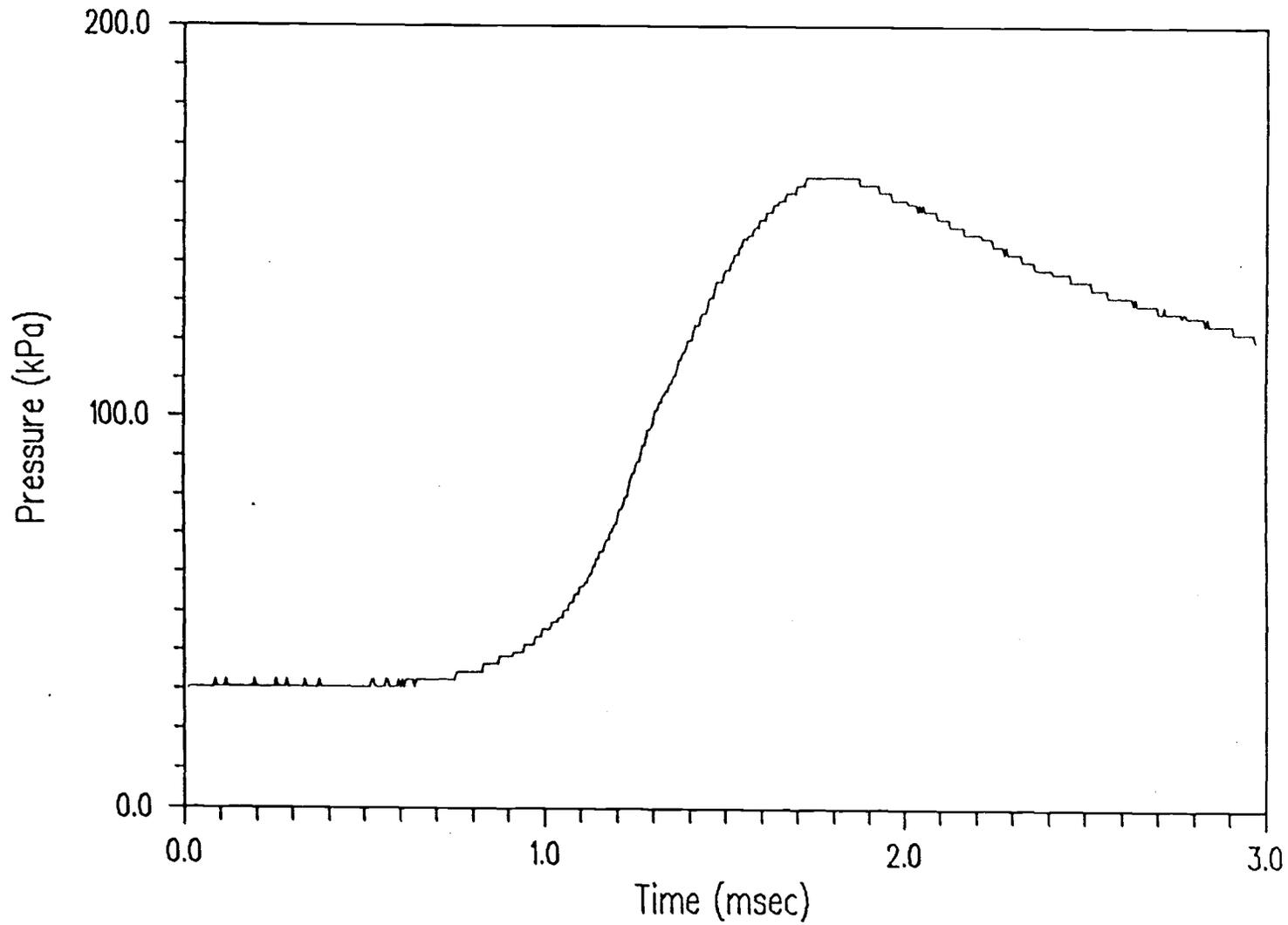
Fig. 23 Chamber pressure during DSARAS experiments.
