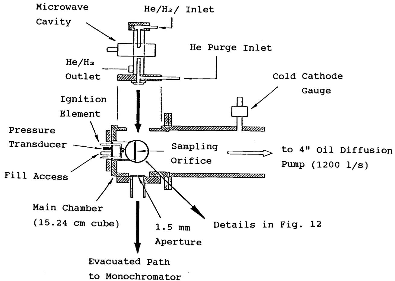
Fig. 11 Diagnostic portion of Direct Sampling Atomic Resonance Absorption Spectroscopy (DSARAS) apparatus.
