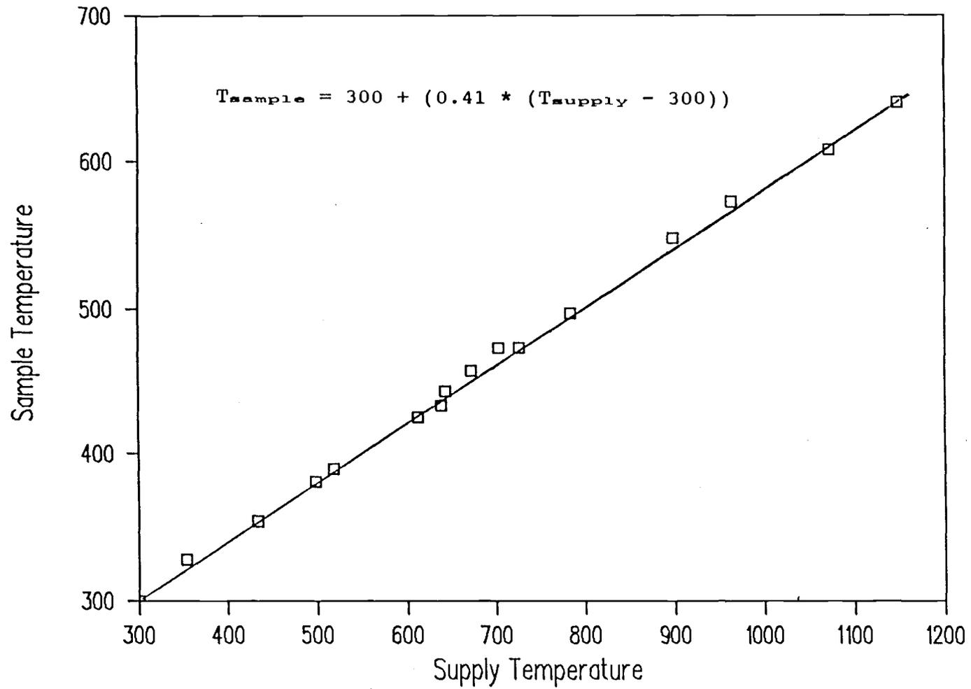
Fig. 22 Correlation of measured temperatures used in validating model.
