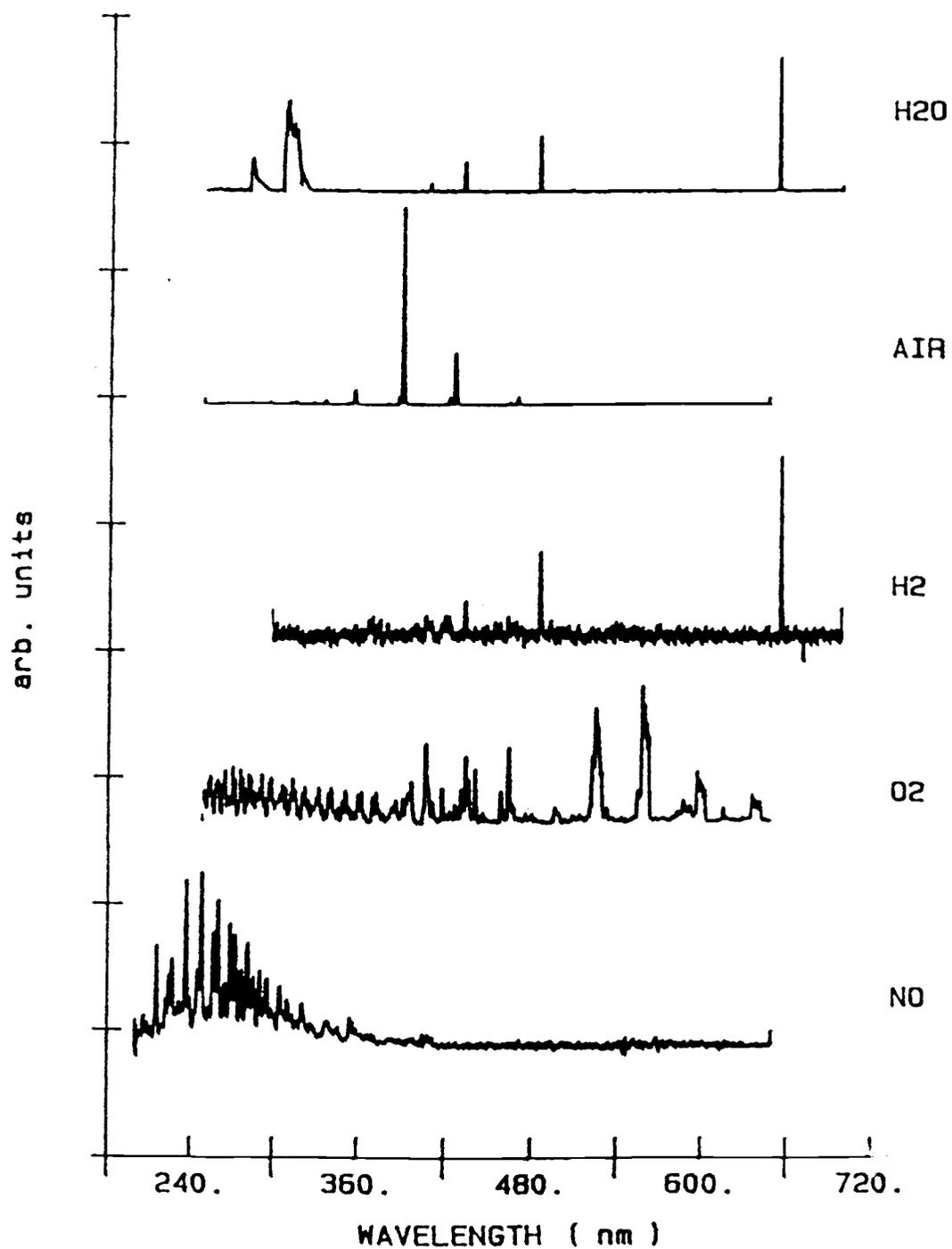
Fig. 6 DSEIF spectra of low temperature gases.
