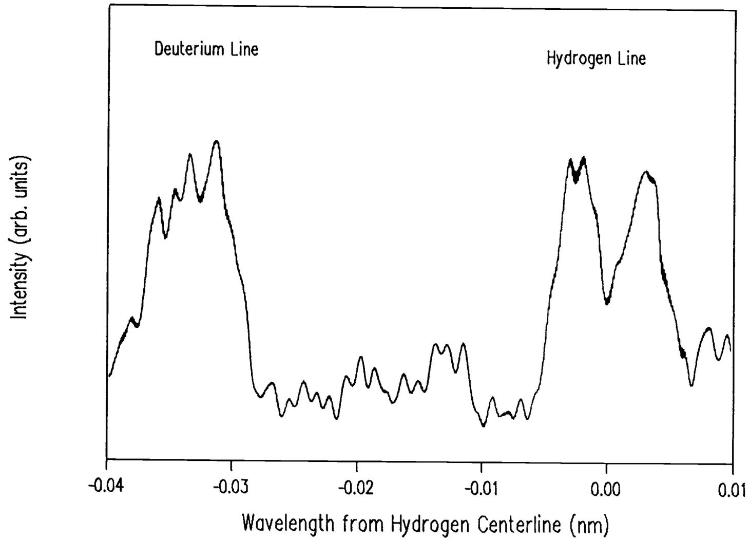
Fig. 20 Spectrum containing 47th order hydrogen and deuterium Lyman- $\alpha$  lines.
