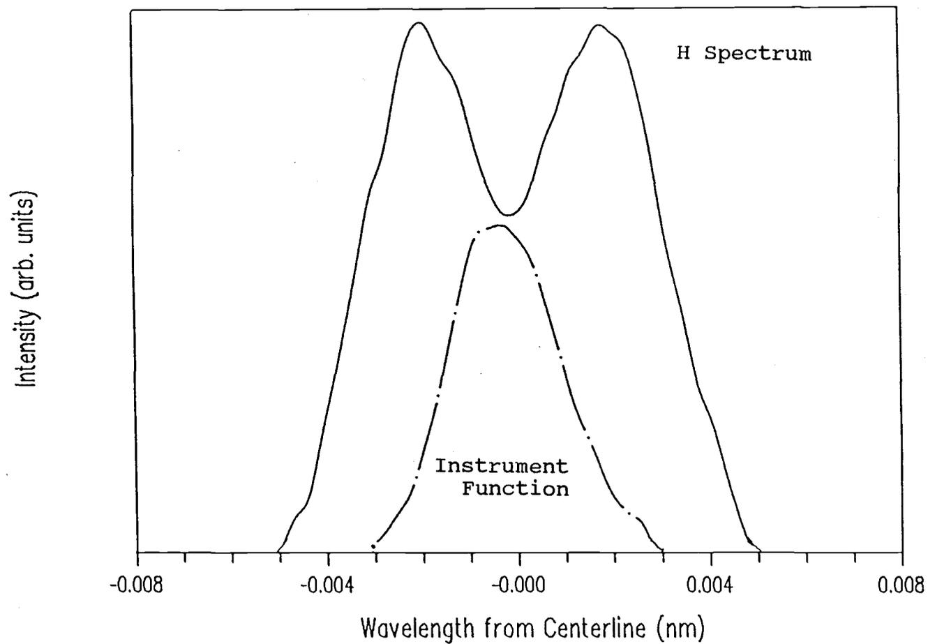
Fig. 21 Recorded hydrogen emission line along with the monochromator instrument function
