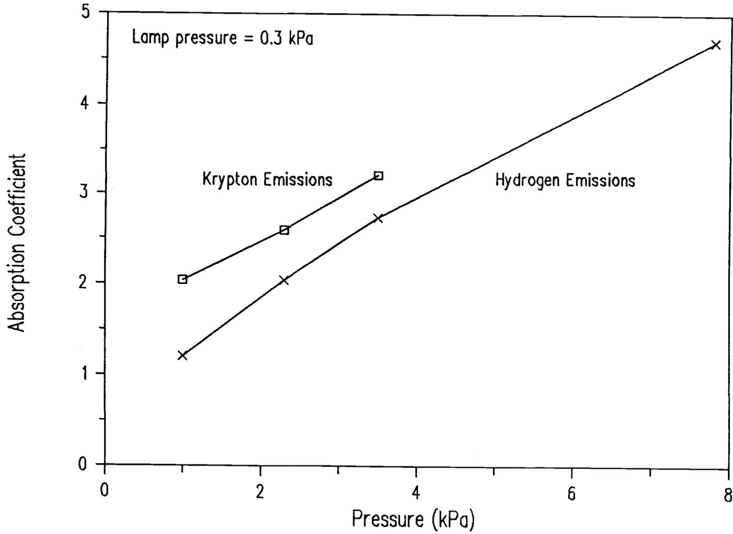
Fig. 17 Variations of  $K_{oL}$  with emitter gas supply pressure.
