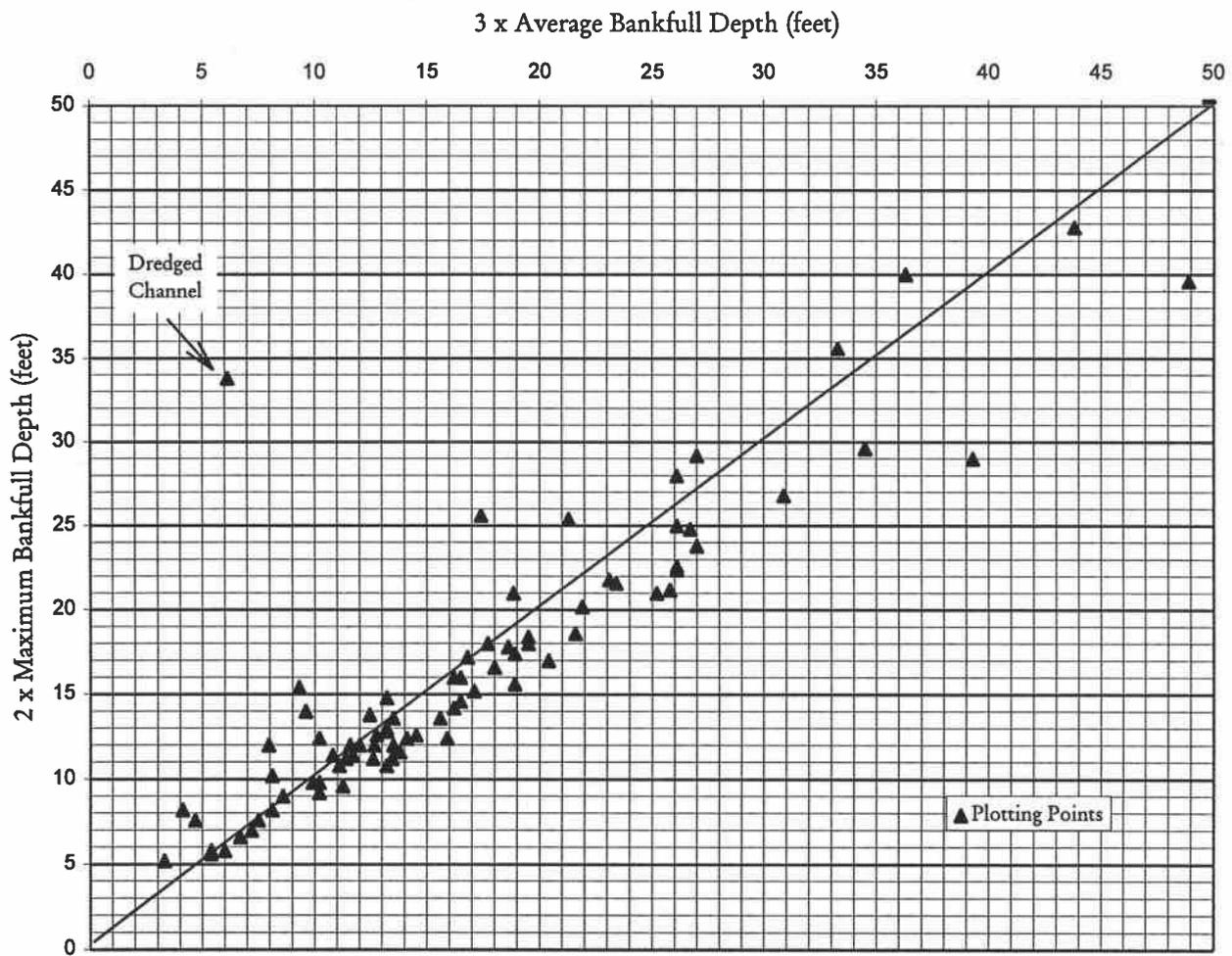
Figure 2.4 Floodprone Depth Calculation Comparison
