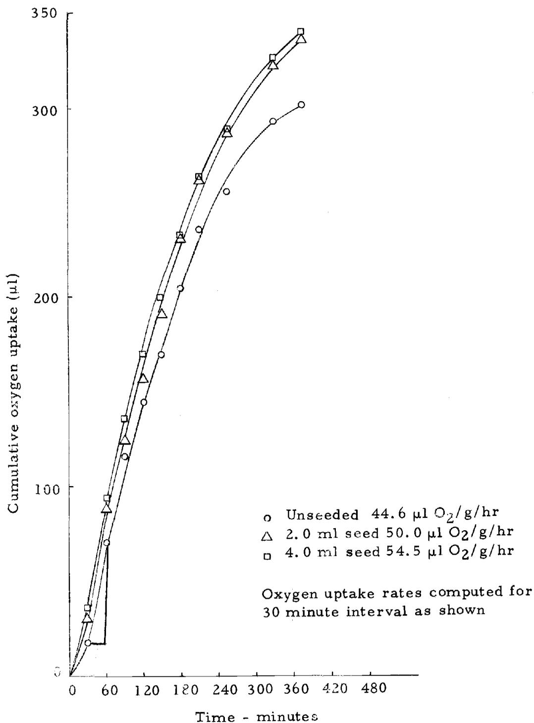
Figure 5. Cumulative oxygen uptake vs. time for unseeded and bacterially seeded estuarine bottom sediments. (Core II, from Smith River at the Umpqua Estuary on the southern Oregon Coast.
