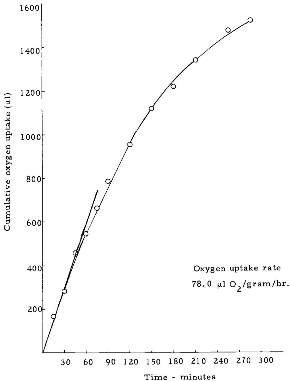
Figure 8. Cumulative oxygen uptake vs. time for resuspended estuarine bottom sediment after storage at  $4^{\circ}\text{C}$  for 4 days.
