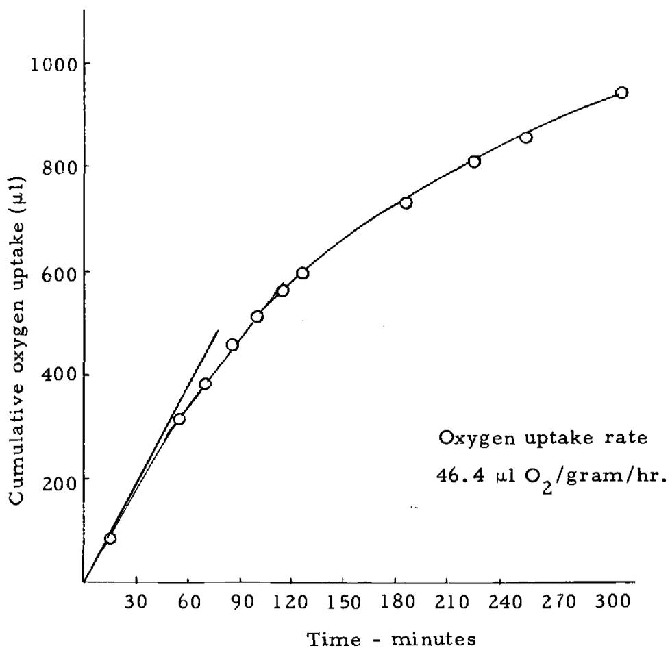
Figure 7. Cumulative oxygen uptake vs. time for resuspended estuarine bottom sediment after storage at  $4^\circ\text{C}$  for 2 days. (Core I from the Smith River at the Umpqua Estuary on the southern Oregon Coast.)
