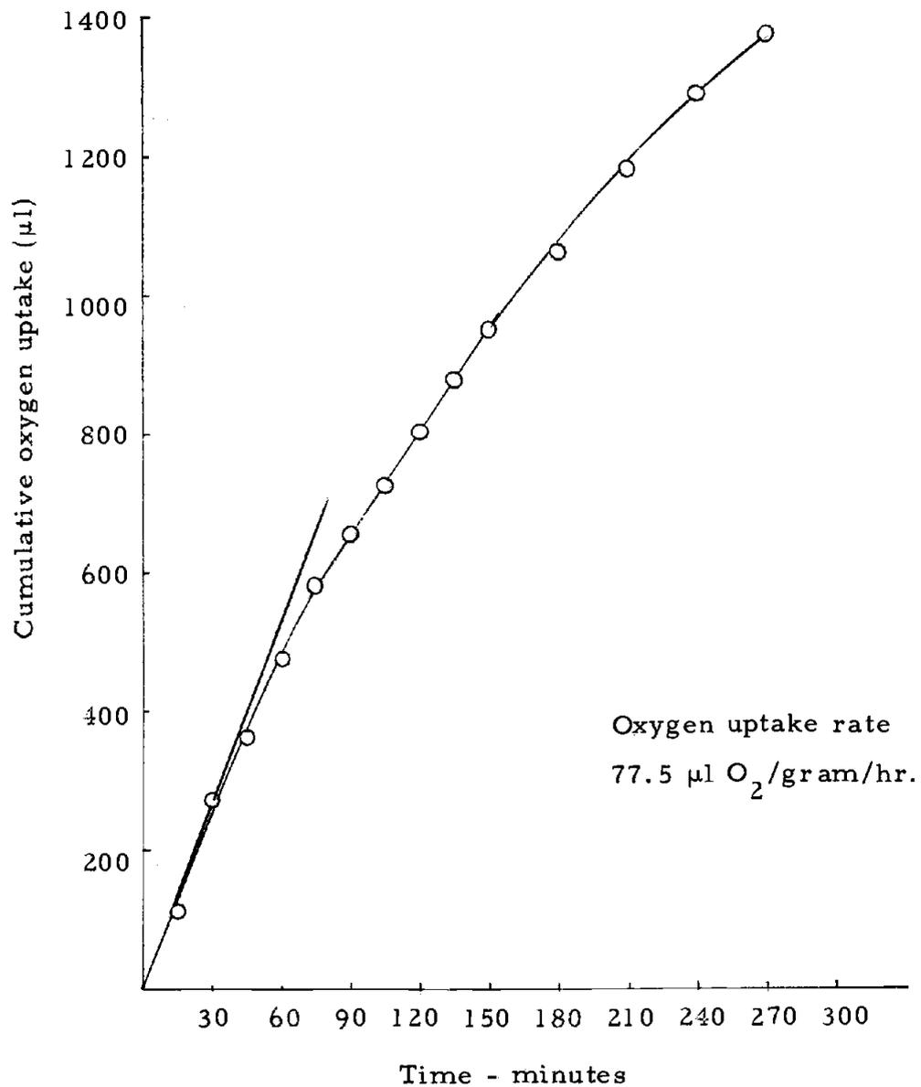
Figure 9. Cumulative oxygen uptake vs. time for resuspended estuarine bottom sediments after storage at  $4^\circ\text{C}$  for 8 days.
