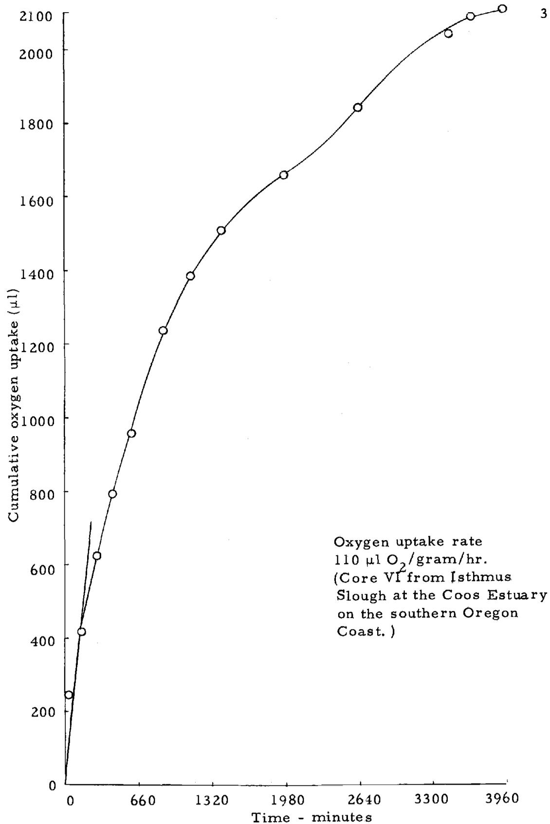
Figure 14. Cumulative oxygen uptake vs. time for resuspended estuarine bottom sediment.
