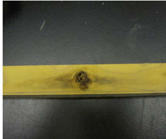
Figure 3.2: Specimen with a knot at mid-height of the face
