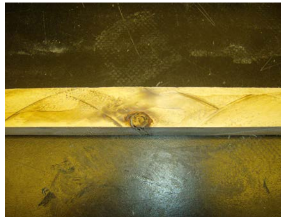
Figure 3.2: Specimen with a knot at mid-height of the face
