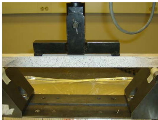
Figure 3.4: Specimen with a knot in tension
