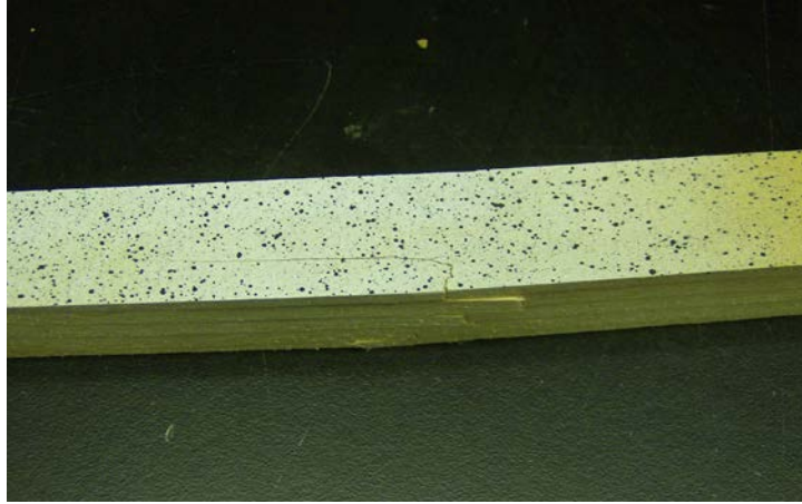
Figure 4.8: Failure crack on tension side for clear beam.
