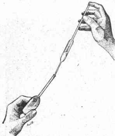
Fig. 3—Correct position for holding test bottle and pipette.
