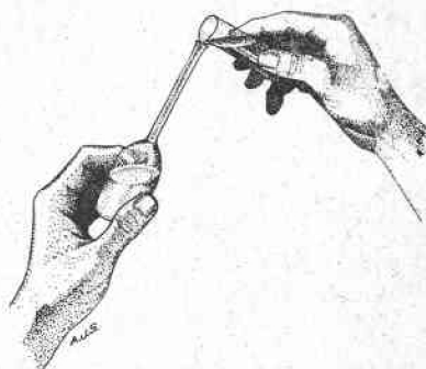
Fig. 4—Correct position for holding test bottle when pouring acid.
