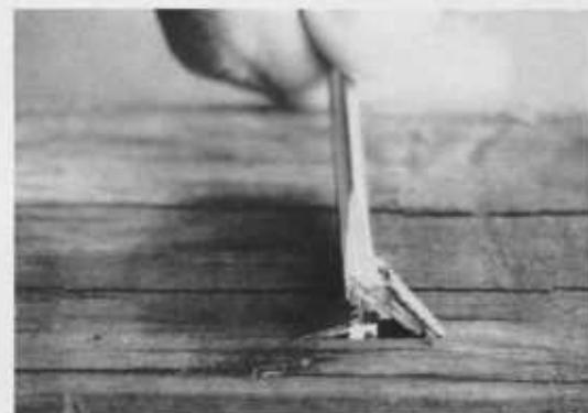
Figure 5.—The splinter test is useful for detecting decayed wood. Long splinters (above) indicate sound wood. Soft, easily broken wood around the probe (below) indicates decay.
