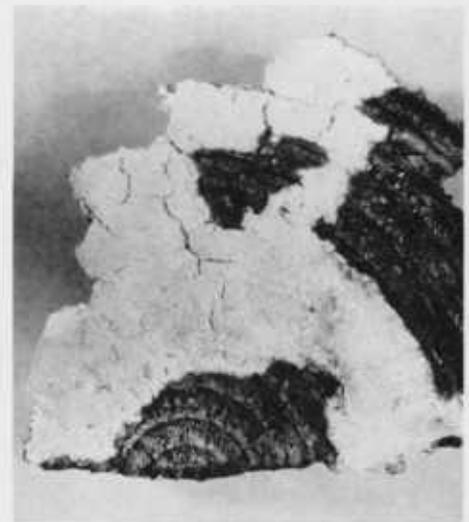
Figure 1.—These shelflike brackets (left) are fruiting bodies of a decay fungus within these boards. A whitish to yellowish mat of a fruiting body (right) indicates a decay fungus within this Douglas-fir.
