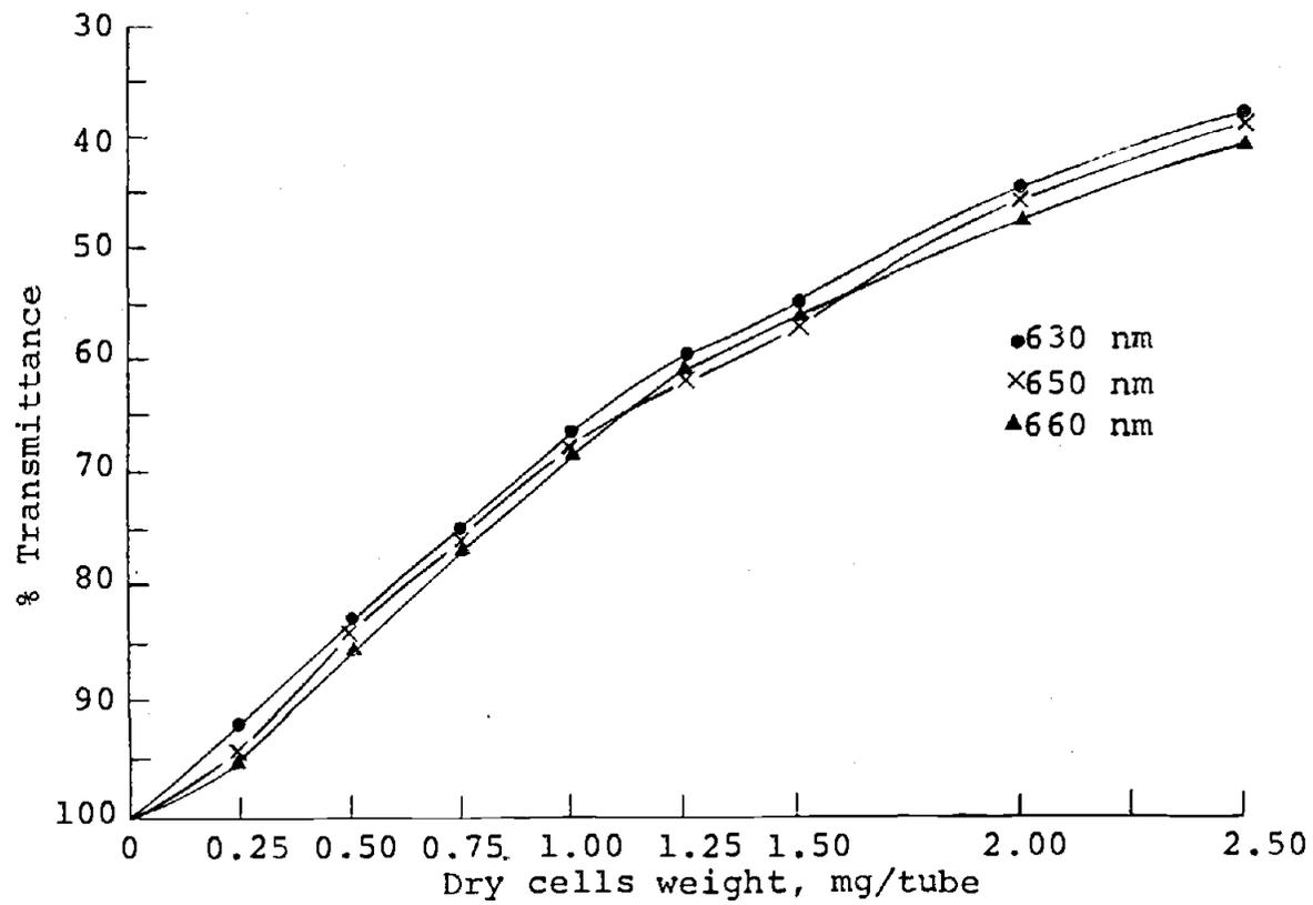
Figure 2. Calibration of Spectronic 20.
