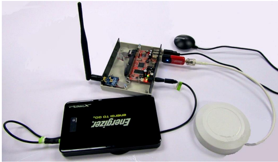
Figure 3: Bluetooth Data Collection Unit
