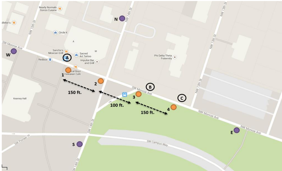
Figure 10: Bluetooth Data Collection System for the Fourth Data Collection Experiment
