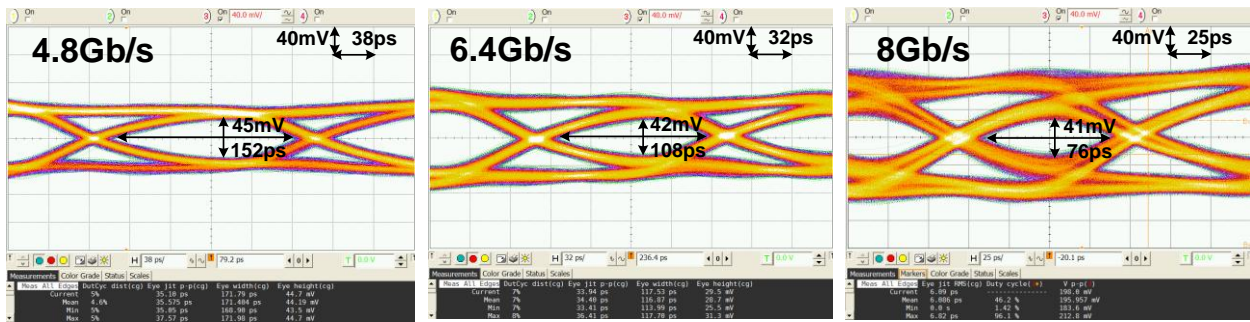
Fig. 20. 4.8Gb/s, 6.4Gb/s, and 8Gb/s transmitter output eye diagrams.
