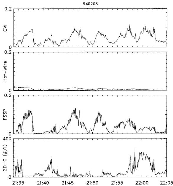
FIG. 3. Condensed water content as a function of time measured in a mountain wave cloud on 3 February 1994. The top trace is from the CVI, the second is from the hot-wire probe, the third is from the FSSP-100, and the fourth is number concentration from the PMS 2D-C probe. All units are grams per cubic meter except for the 2D-C, which is in units per liter.
