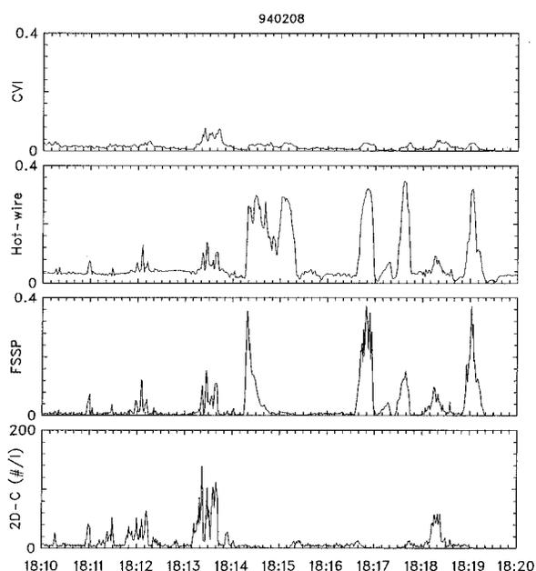
FIG. 2. Condensed water content as a function of time measured during a winter storm on 8 February 1994. The top trace is from the CVI set at a 20- $\mu\text{m}$  cut size, the second is from the CSIRO King hot-wire probe, the third is from the FSSP-100, and the fourth is number concentration from the PMS 2D-C probe. All units are grams per cubic meter except for the 2D-C, which is in units per liter.
