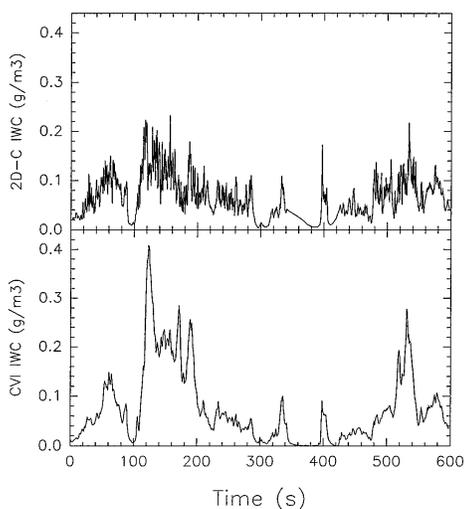
FIG. 5. Condensed water content measured in a cold wave cloud on 4 March 1994 between 2040 and 2050 UTC. Top trace is from the PMS 2D-C probe and bottom is from the CVI.
