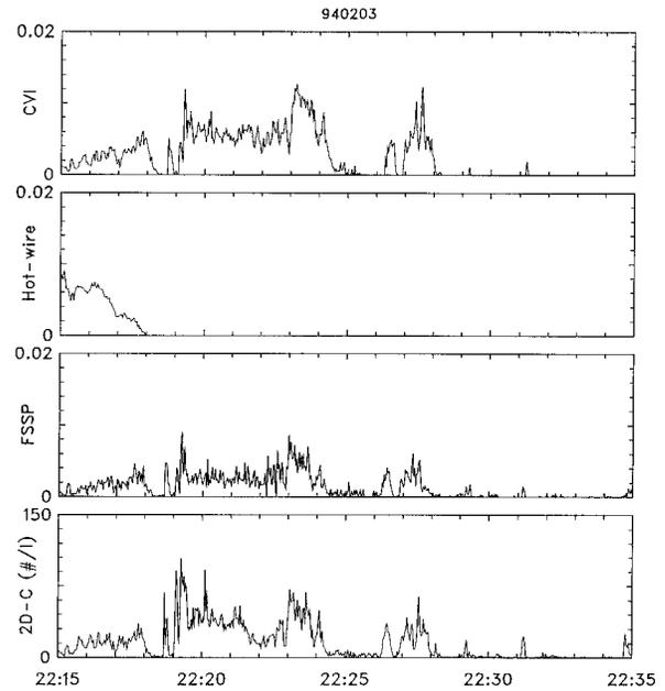
FIG. 4. Condensed water content as a function of time measured in a mountain wave cloud on 3 February 1994 (at a higher altitude than in Fig. 3). The top trace is from the CVI, the second is from the hot-wire probe, the third is from the FSSP-100, and the fourth is number concentration from the PMS 2D-C probe. All units are grams per cubic meter except for the 2D-C, which is in units per liter.
