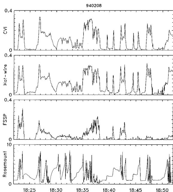
FIG. 1. Condensed water content as a function of time (UTC) measured during a winter storm on 8 February 1994. The top trace is from the CVI, the second is from the CSIRO King hot-wire probe, the third is from the FSSP-100, and the fourth is from the Rosemount icing detector. All units are in grams per cubic meter except for the Rosemount, which is in volts.
