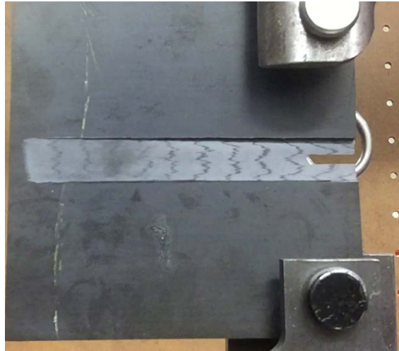
Figure 3. Compact Compression specimen with a machined taper. 0.5-inch width taper, starting at the notch tip; specimen thickness increases to the left in the image. Dimensions are of those in Figure 1 [29].
