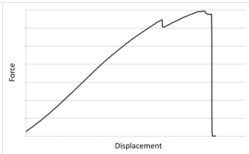
Figure 4. Load-displacement plot of the machined-taper specimen. Note: units and values have been removed due to proprietary nature [29].
