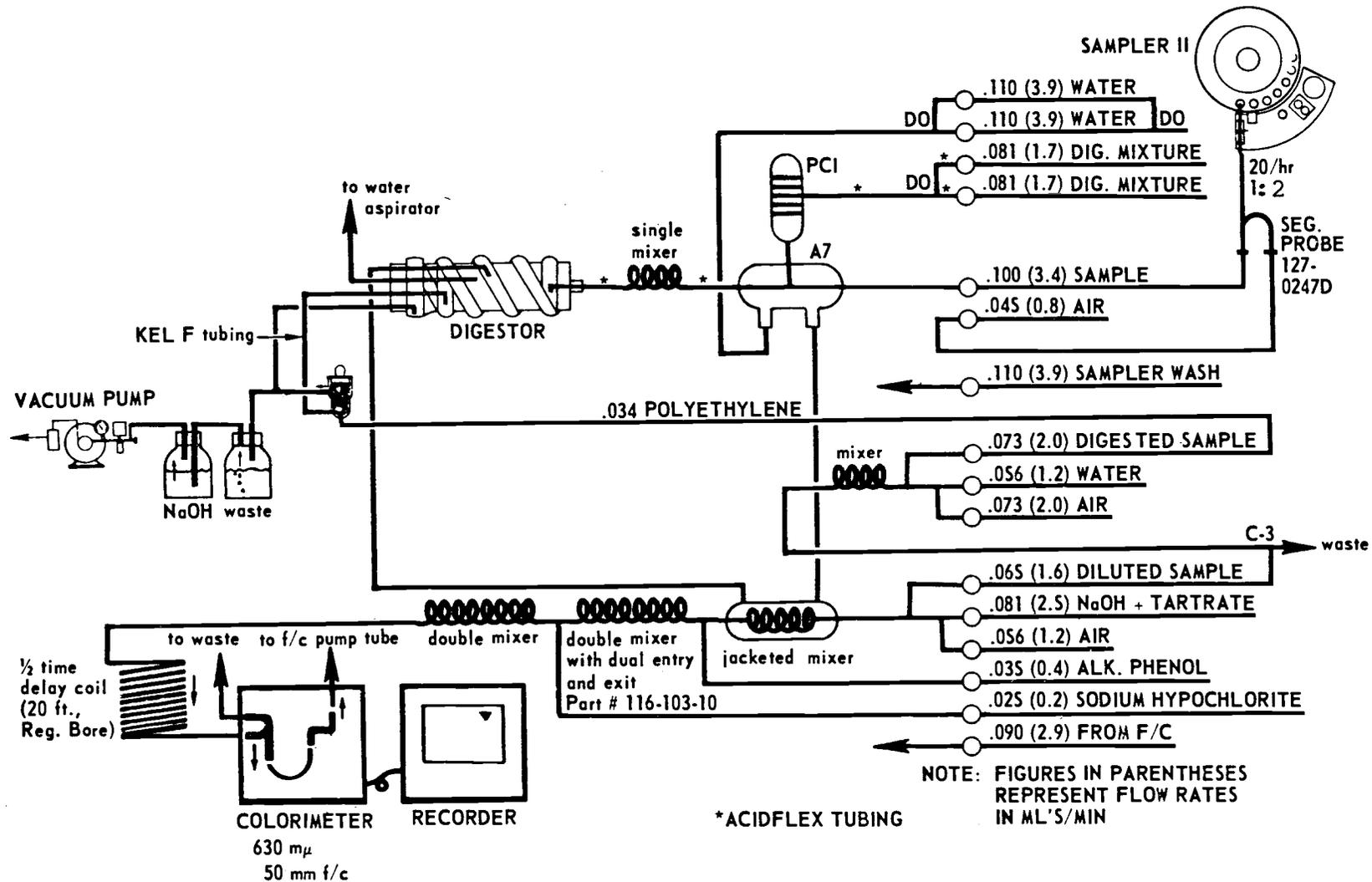
Figure 1. Flow diagram for Kjeldahl nitrogen determination using Technicon AutoAnalyzer.
