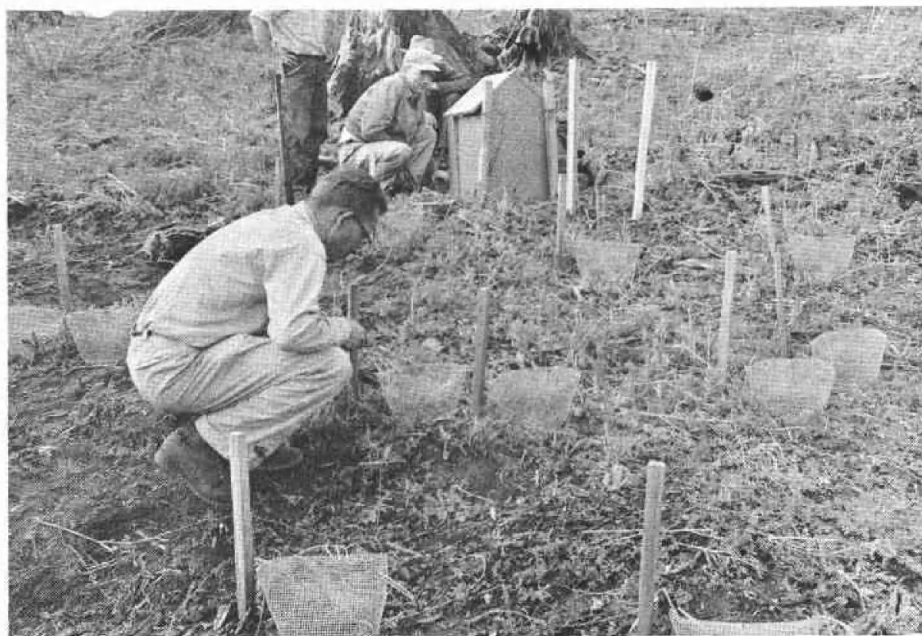
Plate 7. South exposure, May 1955, showing the hoods employed to protect the seeds, and the shelter protecting the soil-air thermograph.
