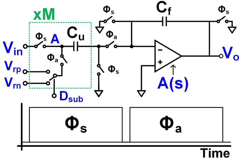
Figure 2.10: A multiplying digital-to-analog converter switched-capacitor circuit is presented. In the sampling phase ( $\Phi_s$ ), the input signal is sampled onto  $M$  unit capacitors. In the amplification phase ( $\Phi_a$ ), the capacitors are switched respective to  $D_{sub}$  to create the quantization error and amplify it.
