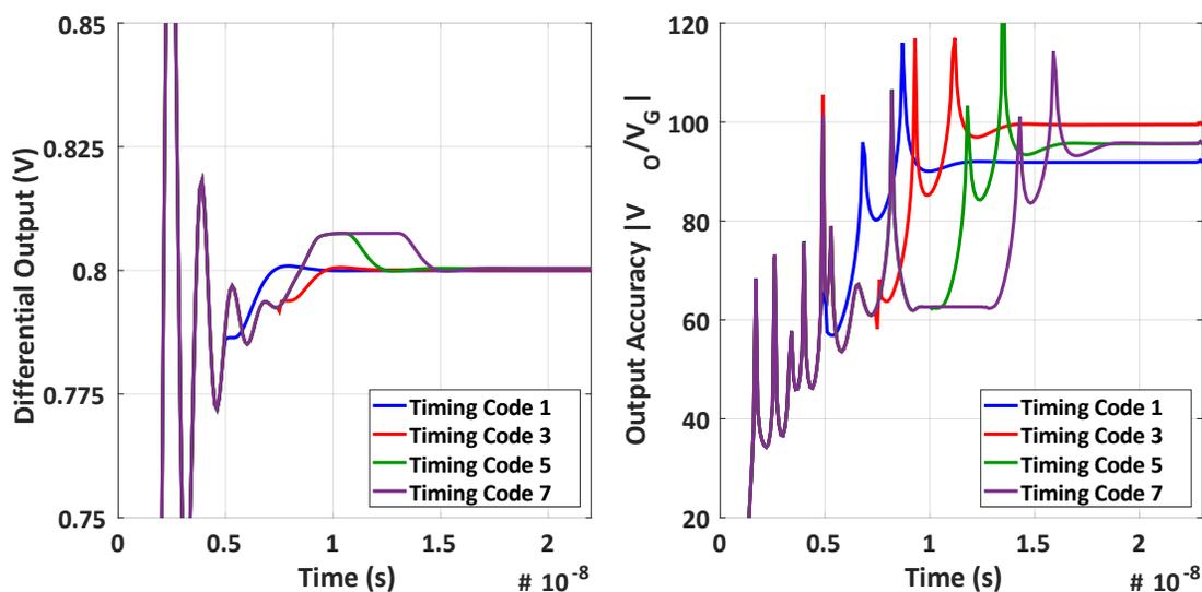
Figure 5.12: Timing of the estimate and fine amplification phases is varied and the settling performance of the dual-path ring amplifier is observed.
