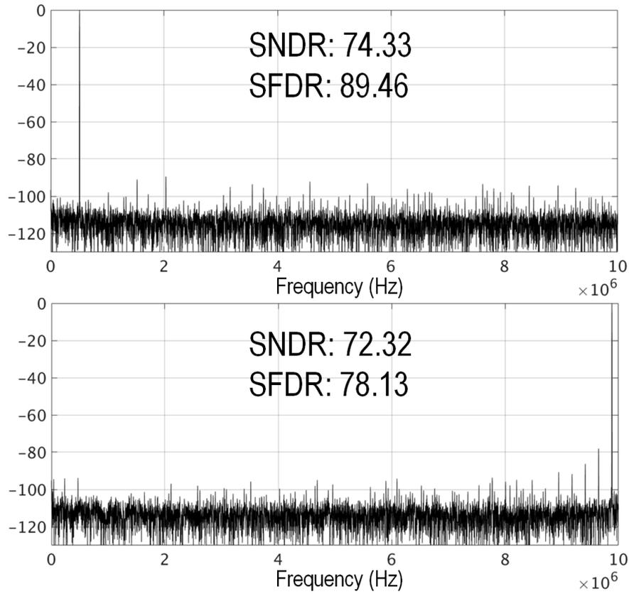
Figure 4.18: High and Low Frequency PSDs with a 10 MHz and 500 KHz input respectively with the ADC operated at 20 MSPS.
