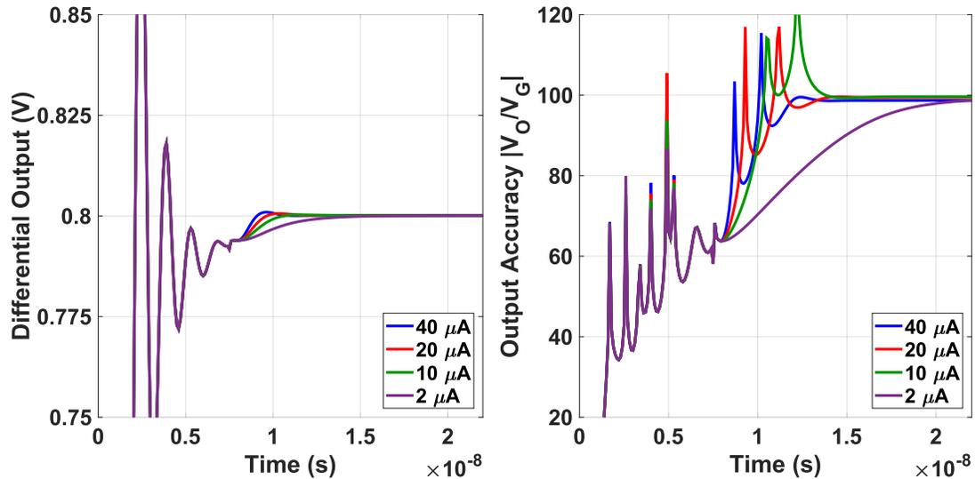
Figure 5.13: Bias current of the fine output stage is varied and the settling performance of the dual-path ring amplifier is observed.
