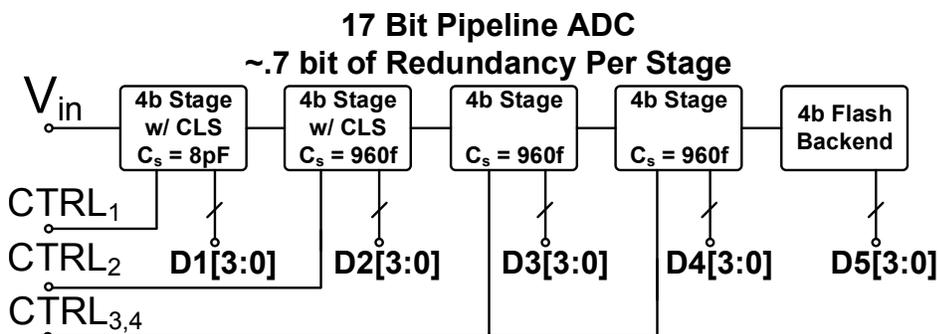
Figure 5.14: This the top level diagram of the 17b pipelined ADC implemented with the dual-path ring amplifiers in a correlated level shifting MDAC in stages 1 and 2. In stages 3 and 4 a standard differential input current-starved inverter ring amplifier in Figure 5.1.
