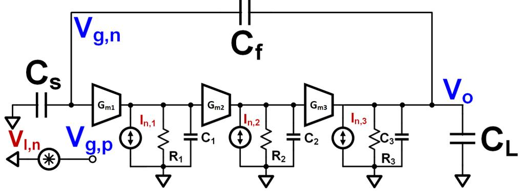
Figure 4.9: A simple linearized small-signal model of a ring amplifier during amplification with device noise sources added. Used to analyze the small signal noise performance of a ring amplifier.
