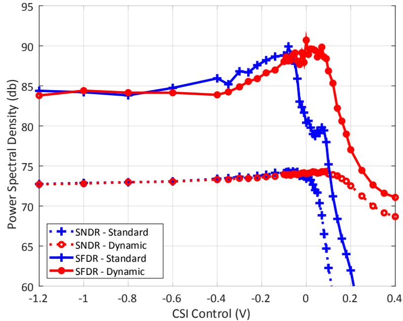
Figure 4.20: A plot of the measurement results of the pipelined ADC. SNDR and SFDR are plotted across control voltages with and without the dynamic deadzone circuitry enabled.
