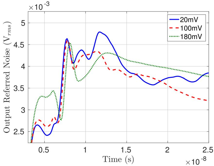
Figure 4.11: Instantaneous root-mean square output noise voltage of the current-starved inverter ring amplifier during amplification.
