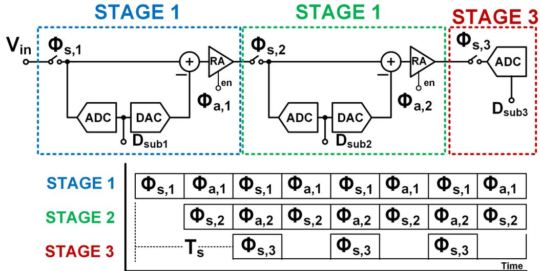
Figure 2.7: This is a system level and timing diagram of a three-stage pipelined ADC.
