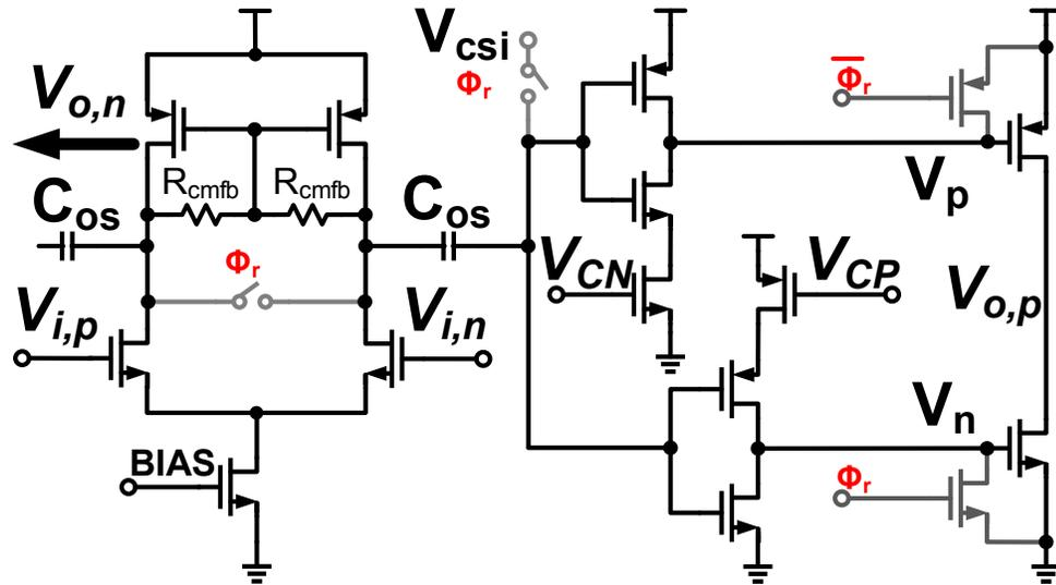
Figure 5.1: This is a circuit diagram of a current-starved inverter ring amplifier with a differential input stage.
