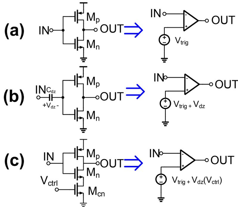
Figure 4.2: Three different inverter implementations and their analogous representation with a differential amplifier.
