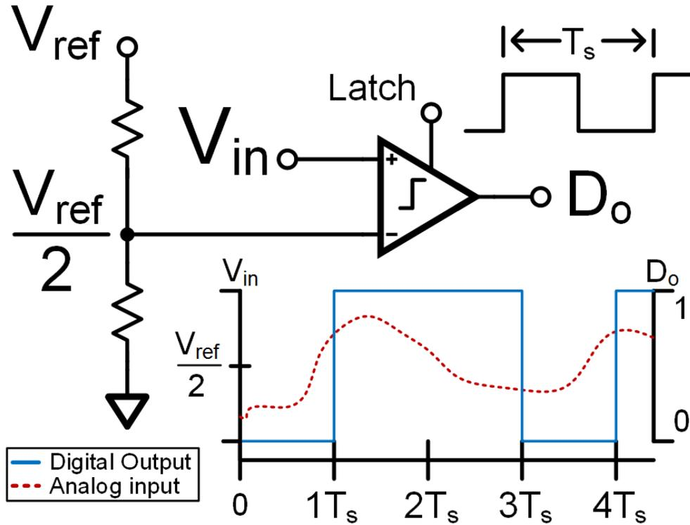
Figure 2.4: Shown is a comparator configured as a one bit ADC with a resistor ladder providing the reference threshold.
