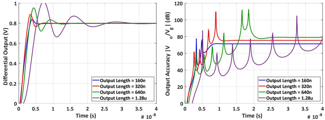
Figure 5.4: This contains the settling response of a ring amplifier when output length is swept and current-density is maintained. Loading of the second-stage by the devices in the third stage degrades performance when larger channel lengths are used.
