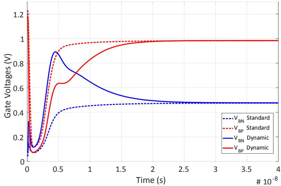
Figure 4.8: This is a waveform of the gate settling voltages of a current-starved inverter ring amplifier with and without dynamic deadzone control.
