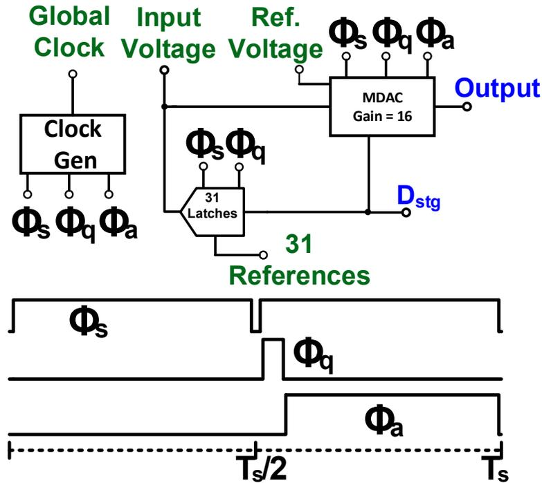
Figure 4.14: Seen is the system level diagram of the first stage of the pipelined ADC along with the timing diagram.
