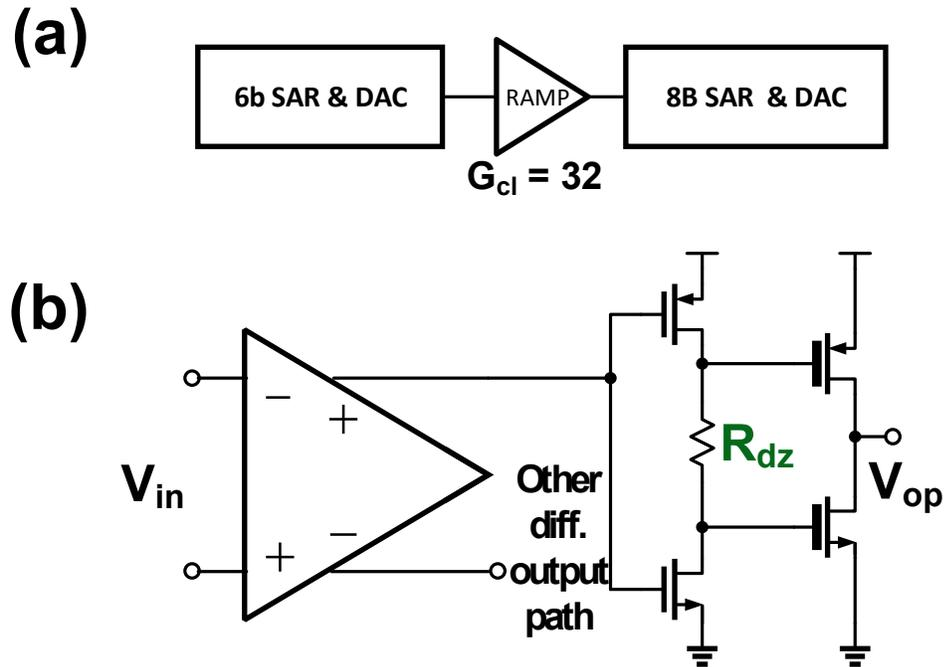
Figure 3.8: A simplified top level diagram of a pipelined-SAR with a ring amplifier (a). The resistor-based output stage of the ring amplifier used in the pipelined-SAR (b).
