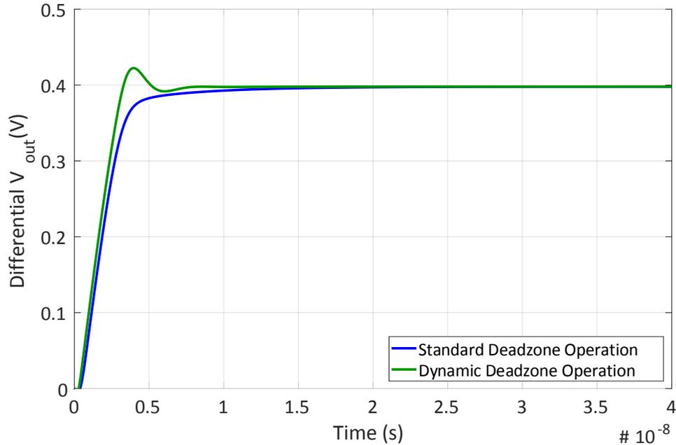
Figure 4.7: This is a settling waveform of an over-damped current-starved inverter ring amplifier with and without a dynamic deadzone enabled.
