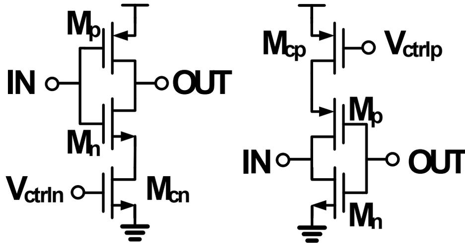
Figure 4.1: Two circuit implementations of a current-starved inverter are shown one with a NMOS control FET and the other with a PMOS control FET
