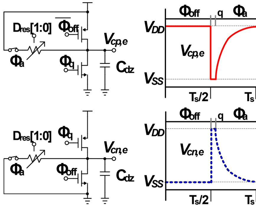
Figure 5.10: A dynamic deadzone generation circuit for the dual-path ring amplifier's estimate output path is presented.
