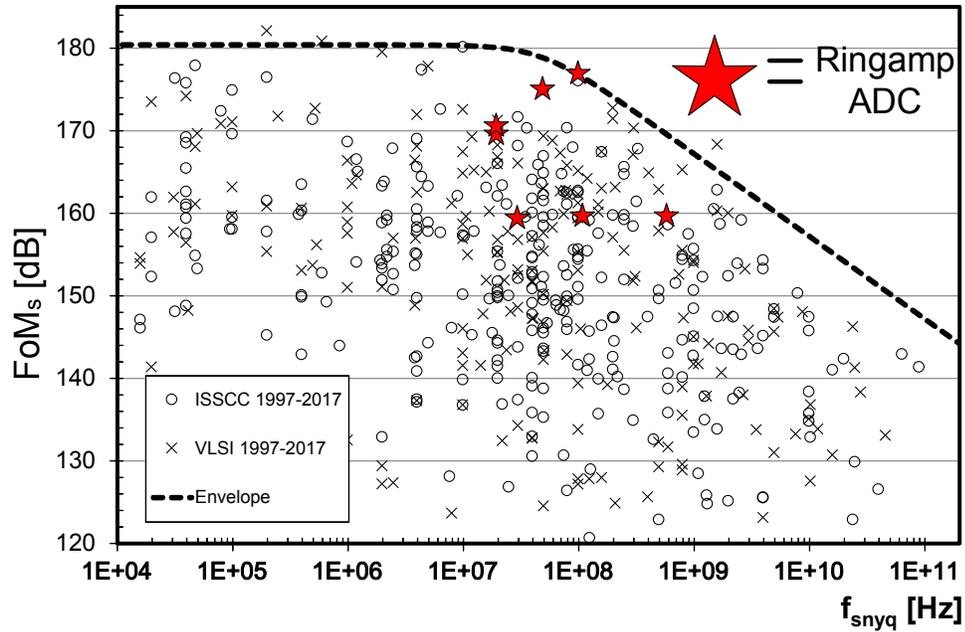
Figure 1.2: A plot of ADC performance versus Nyquist input frequency with ring amplifier based ADCs highlighted.
