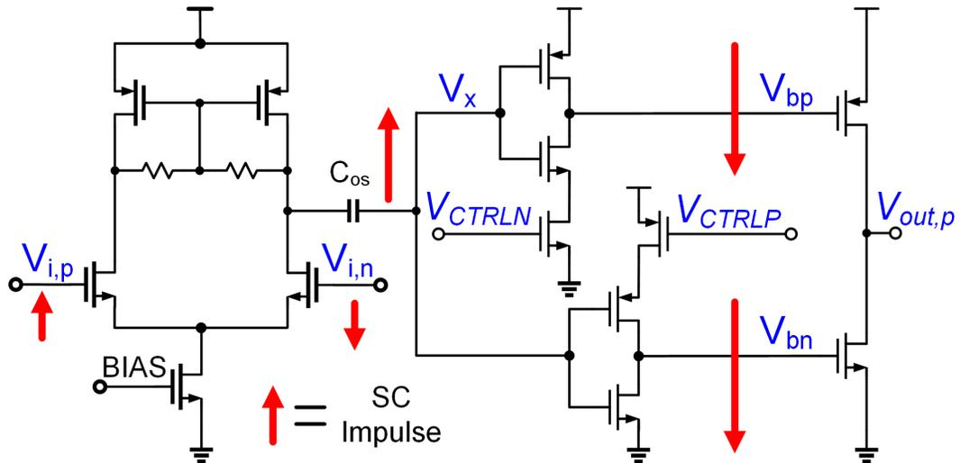
Figure 3.4: Initial impulse directions due to a switched-capacitor input are used to demonstrated how the signal of a ring amplifier can alter the bias of the output stage.
