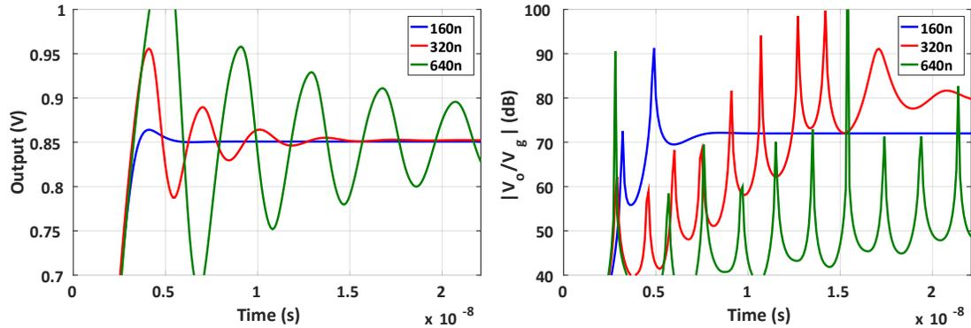
Figure 5.3: Settling performance of a current-starved inverter with first-stage lengths swept and current-density maintained is presented. Performance rapidly degrades with an increase in length.
