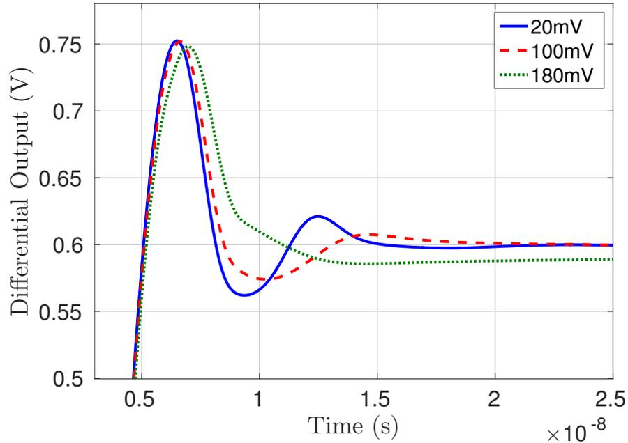
Figure 4.10: Settling response of current-starved inverter ring amplifier used in the first stage of the noise investigation pipelined ADC is shown. Three different control voltages are represented in the graph
