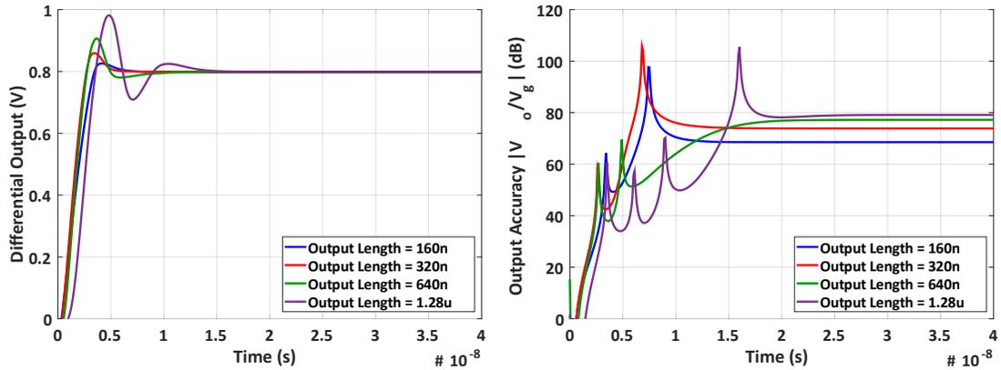
Figure 5.5: This contains the settling response of a ring amplifier when the length of output transistors is swept and current-density is maintained. The ring amplifier used in these waveforms consumes four times as much current in the second stage in Fig 5.4
