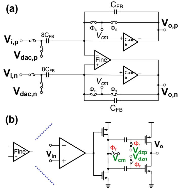
Figure 3.9: The simplified coarse-fine ring amplifier only amplification structure used in (a). The structure the ring amplifier used for fine amplification (b).
