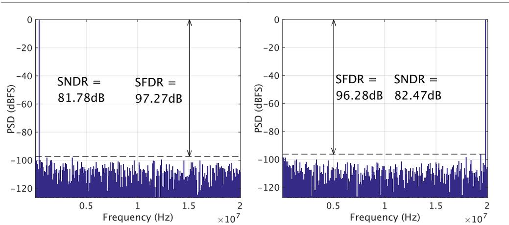
Figure 5.17: Simulated 512 point FFT power spectral density of the dual-path ring amplifier pipelined ADC with a low and high frequency input with a sampling frequency of 40 MHz.
