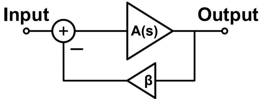
Figure 2.8: This is a system level diagram of a generalized negative feedback system used to achieve.
