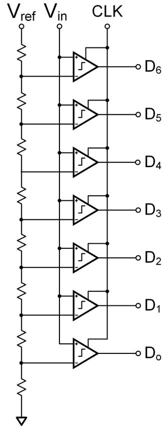
Figure 2.5: A simplified schematic of an 3 bit flash analog-to-digital converter is shown. This figure includes the 7 references generated by a resistor ladder and 7 comparators to achieve 3 bit resolution.
