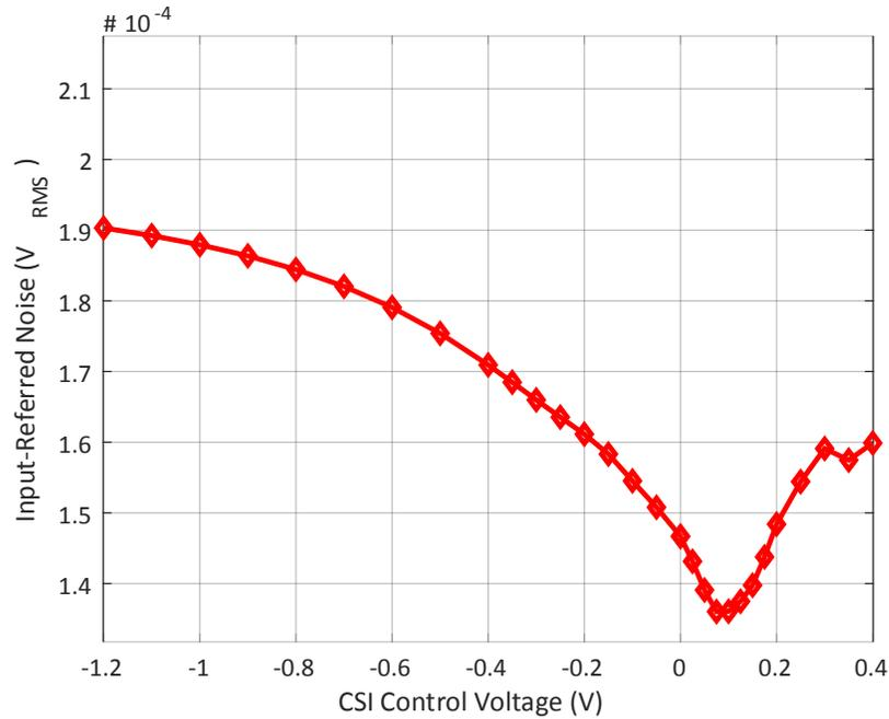
Figure 4.12: Output noise root-mean square voltage at the end of amplification for the current-starved inverter ring amplifier over a usable range of control voltages.
