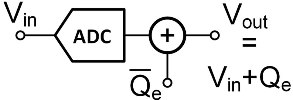
Figure 2.2: This is a model of a generalized ADC with quantization noise modeled as an additive noise source after quantization.
