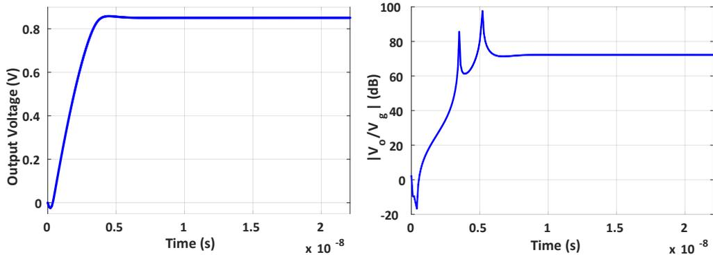
Figure 5.2: Settling performance of the current-starved inverter ring amplifier when all transistors are chosen with minimum lengths is presented.
