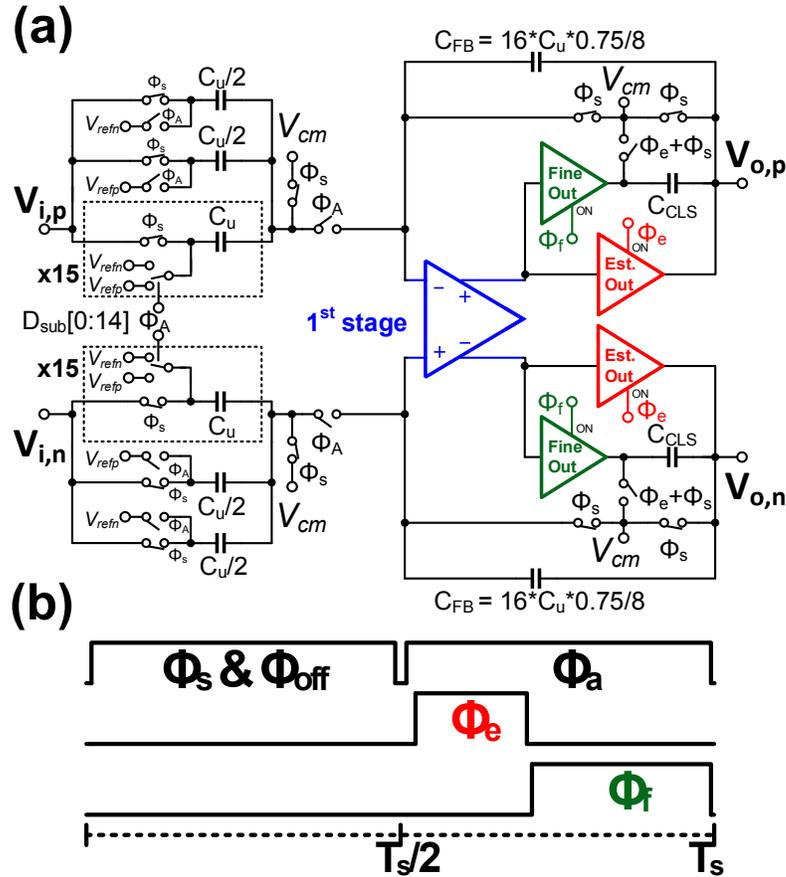
Figure 5.7: The differential multiplying digital-to-analog converter used with a dual-path ring amplifier (a). This structure provides a closed loop gain of 10 and  $2/3$ . Timing diagram of the circuit is shown (b).
