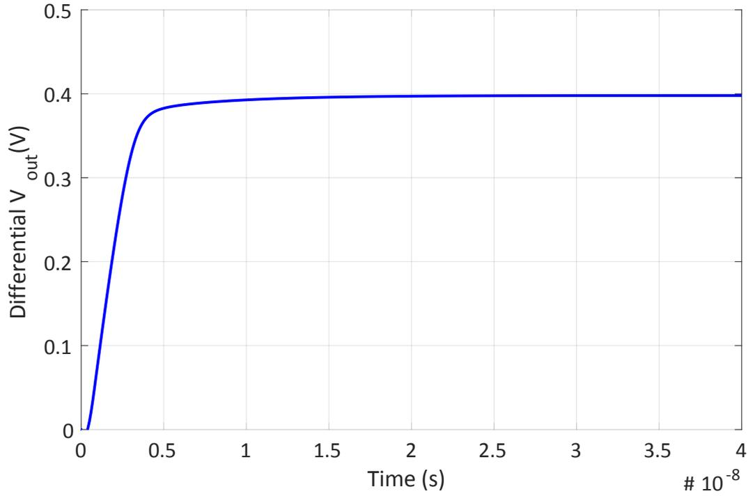
Figure 4.5: This is a settling waveform of an over-damped ring amplifier settling response.
