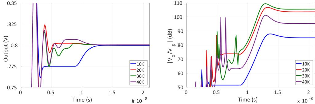
Figure 5.11: Resistor used in the dynamic deadzone biasing of the estimate path (Figure 5.10) is swept and the settling performance of the dual-path ring amplifier is observed.
