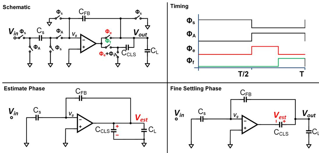
Figure 5.6: This is a diagram of a correlated level shifting amplification scheme.
