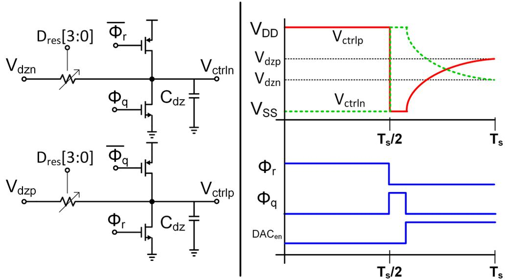
Figure 4.6: This is the circuit diagram used to implement a dynamic deadzone for current-starved inveter ring amplifiers.
