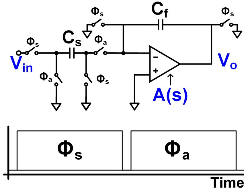
Figure 2.9: Seen is a a switched-capacitor gain stage circuit and timing diagrams. A high-gain amplifier is configured in negative feedback to achieve a precision gain value.
