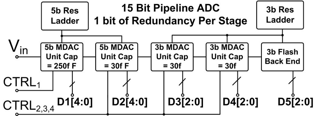
Figure 4.13: Top-level system architecture of the 15b pipelined ADC used to investigate the noise-properties of ring amplifiers.
