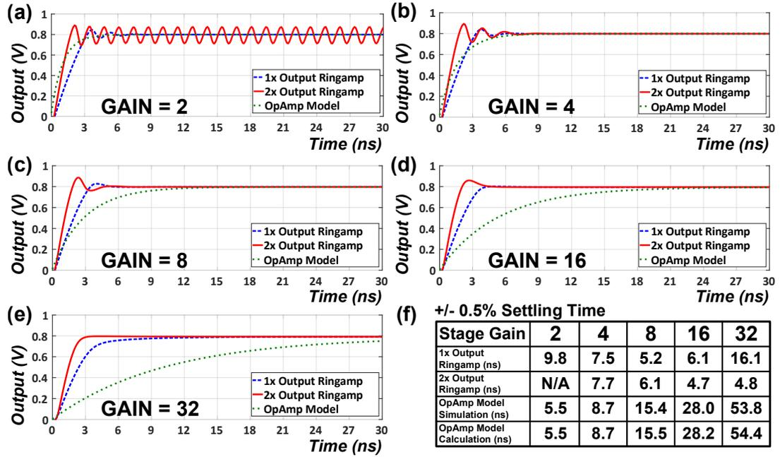
Figure 3.7: Settling response of two example ring amplifier designs in comparison with the OpAmp model across different closed loop gains (a-e). Experimentally obtained and calculated settling times are summarized in a table (f).
