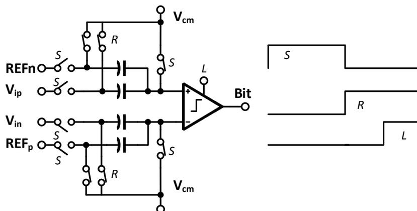
Figure 5.16: A circuit and timing diagram of a one bit slice of a 16 level flash-ADC used in the pipeline stage. In order to implement a 4b flash ADC 15 slices are used in parallel and the appropriate references are sent to each slice at nodes ( $REF_n$  &  $REF_p$ ). The 4b flash is used as the backend and  $ADC_{sub}$  of this pipelined ADC.
