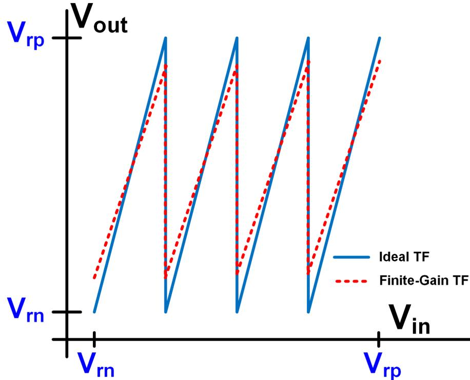
Figure 2.11: A graph of the an ideal 4 level pipeline stage transfer function and the same transfer function when the operational amplifier in the stage has finite-gain limitations
