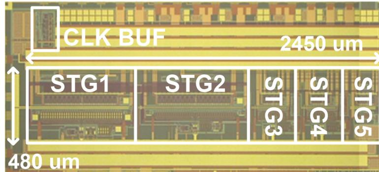
Figure 4.17: A die photo of the prototype 15b pipelined ADC with pseudo-differential current-starved inverters is presented.
