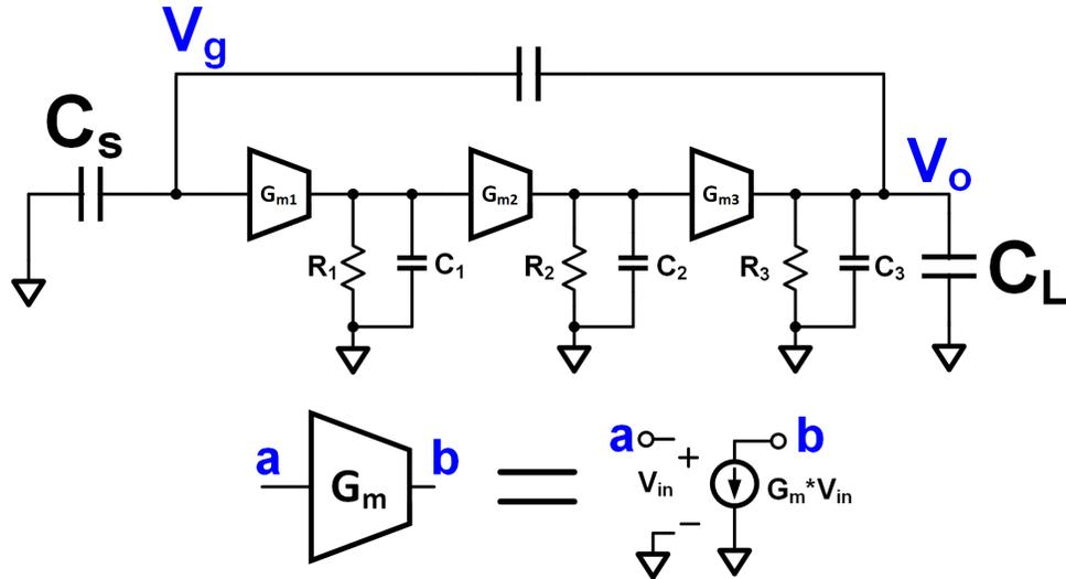
Figure 3.3: A simple linearized small-signal model of a ring amplifier during switched-capacitor amplification is shown. Each gain stage of the ring amplifier is assumed to consist of a transconductance block, resistor and capacitor.
