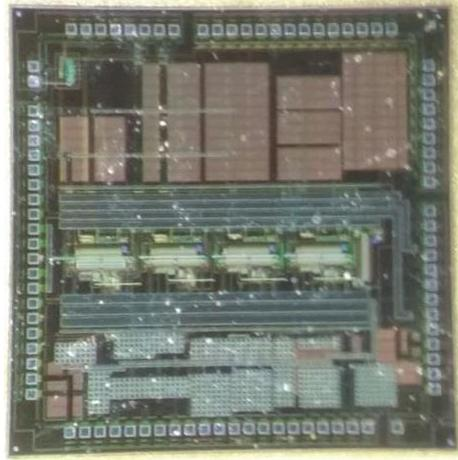
Figure 5.18: This is a die photo of the prototype ADC fabricated in a 180 nm CMOS process.
