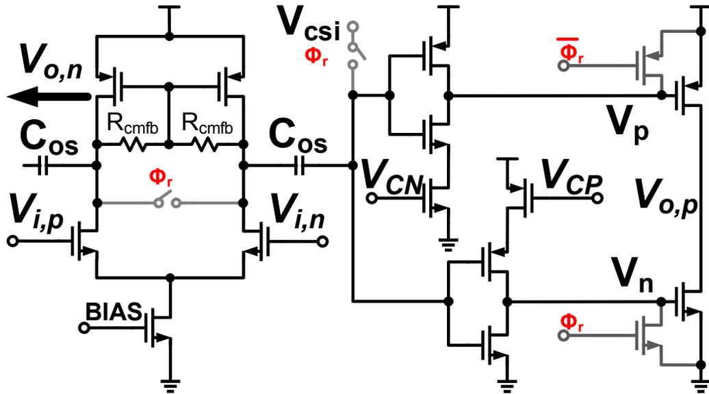
Figure 3.2: This is a differential input current-starved inverter ring amplifier used to discuss ring amplifier biasing and operation. The second and third stages of the negative output  $V_{o,n}$  path are not shown for figure clarity.
