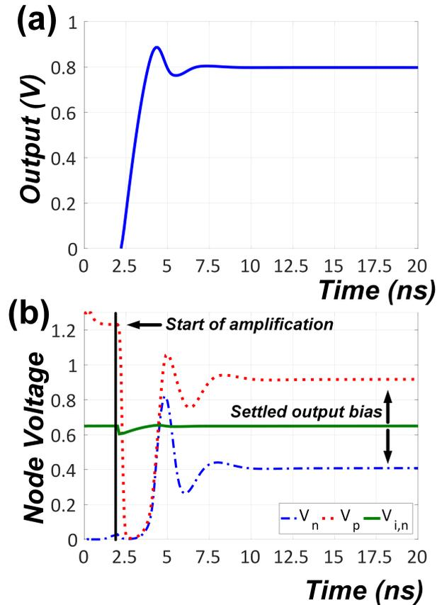
Figure 3.5: Various waveforms of a ring amplifier during switched-capacitor amplification are shown. In (a) the differential output voltage is shown. In (b) the voltage at the gates of the output stage are shown.
