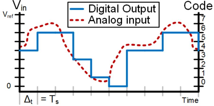
Figure 2.1: This is a demonstration of quantization performed by analog-to-digital converters. The input is rounded to one of 8 levels.
