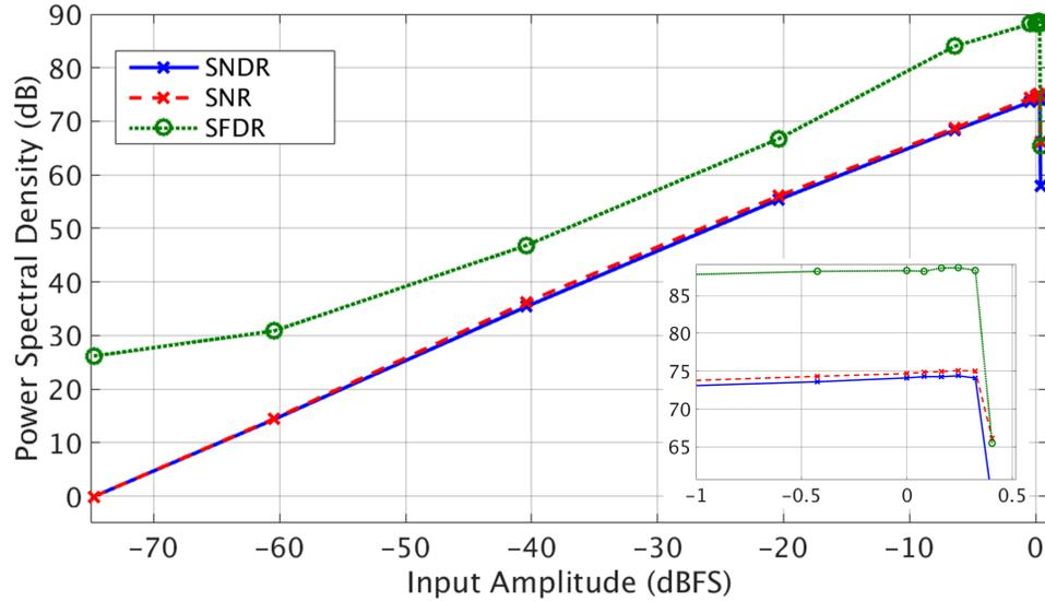
Figure 4.19: Performance measurements of the prototype ADC are plotted versus input amplitude.
