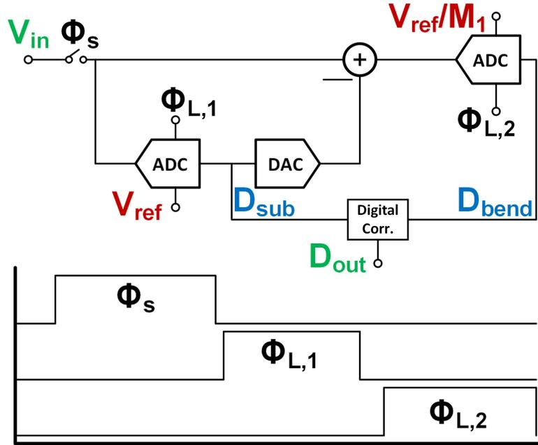
Figure 2.6: A two-stage simplified system level diagram of a sub-ranging ADC is shown. After the input is sampled and quantized by the first ADC, the quantization error is sent to a another ADC which further reduces the overall quantization error of the ADC.
