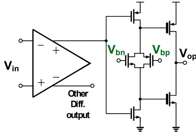
Figure 3.10: Ring amplifier structure used in a 600 MSPS pipelined ADC. The resistors in Figure 3.8(b) have been replaced by biased MOSFET devices.
