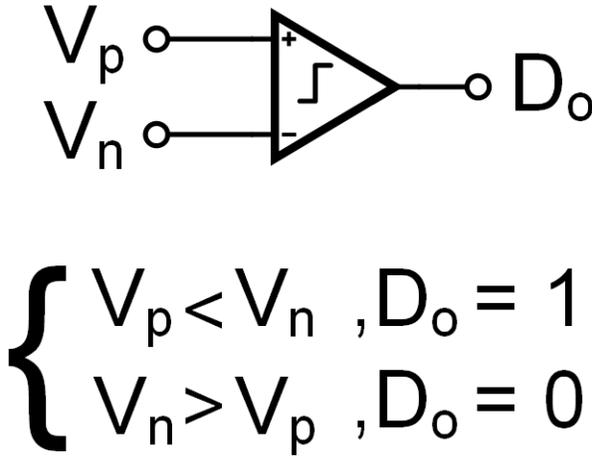
Figure 2.3: A circuit diagram of a comparator and its ideal input-output transfer function are shown
