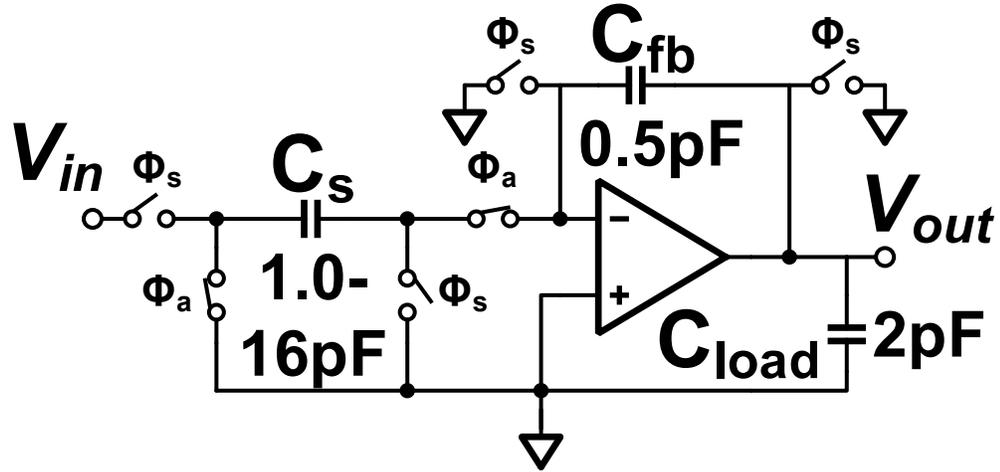
Figure 3.6: Switched-capacitor amplification stage used to investigate dynamic bandwidth of ring amplifiers in comparison with operational amplifiers.  $C_s$  is varied to create different closed-loop gains of the structure while minimizing the change in load seen by the amplifier under test.
