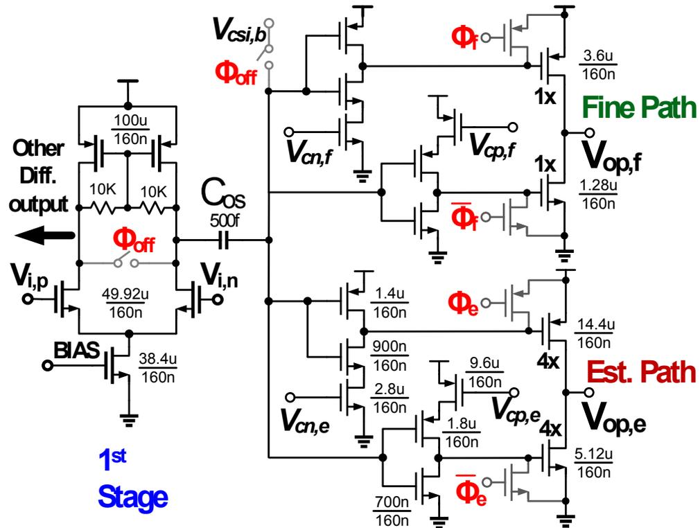
Figure 5.8: Circuit architecture and sizing of the differential dual-path current-starved inverter ring amplifier used in the first stage of the pipelined ADC. One of the differential output paths is omitted for clarity. Sizing of the second-stage is the same in both the estimate and fine output paths
