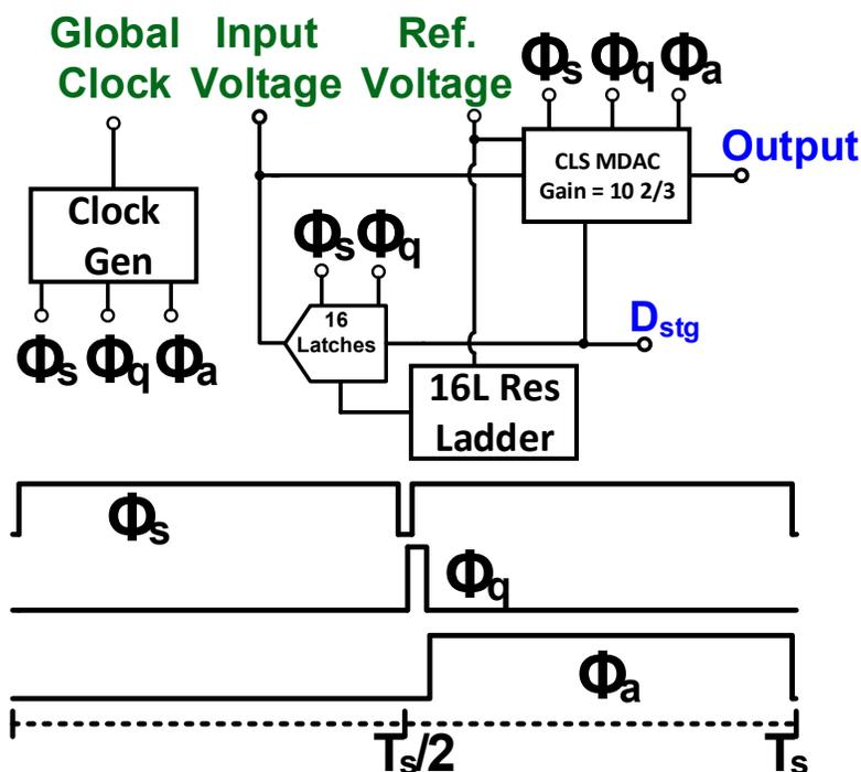
Figure 5.15: A system level and timing diagram of the pipelined stages used in the prototype 17b ADC.
