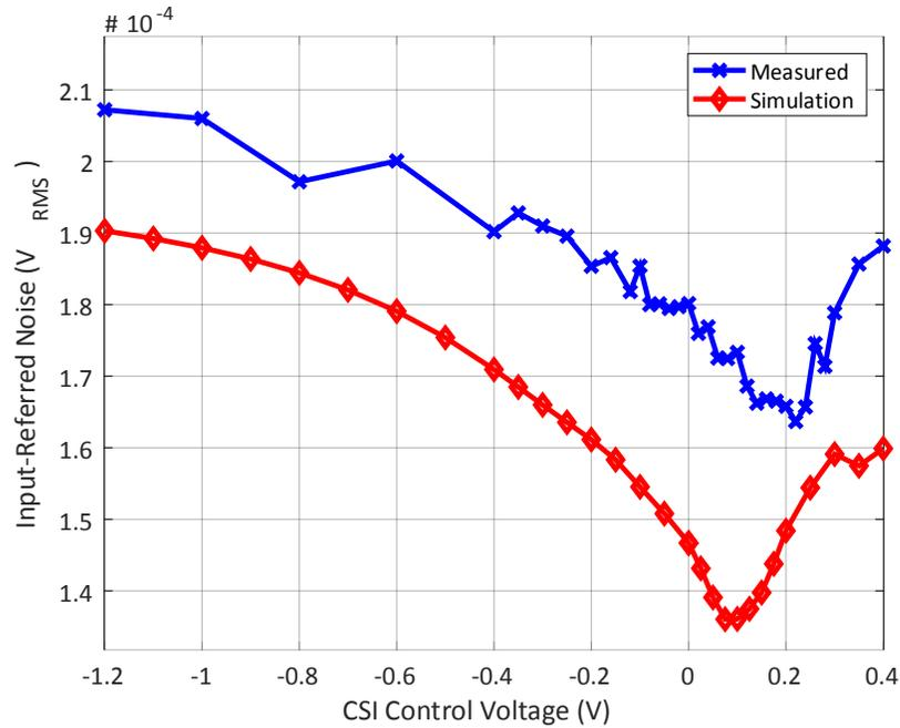
Figure 4.21: Measured and simulated noise floor of the ADC when CSI control voltage is swept.
