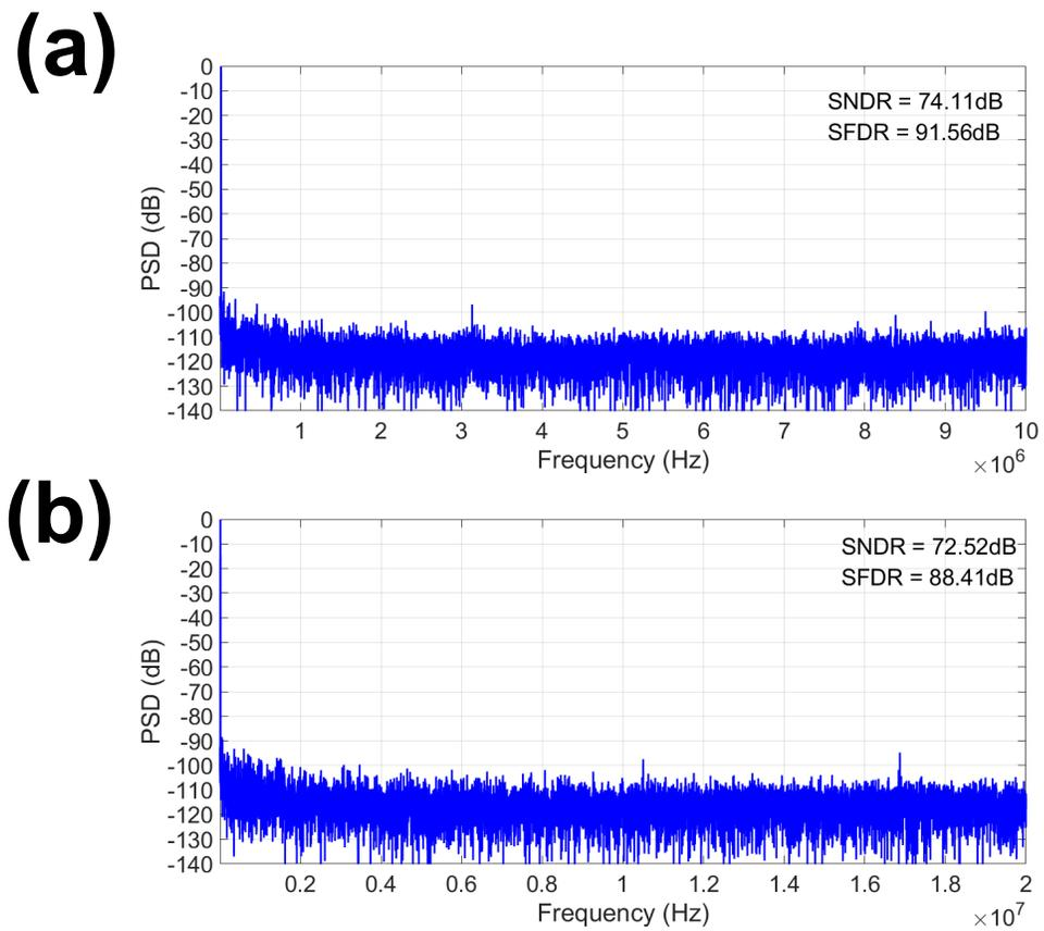
Figure 5.19: This is the measured  $2^{15}$  point FFT PSD of the prototype ADC operated at 20 MSPS (a) and 40 MSPS (b) both with a full-scale 17 KHz input.
