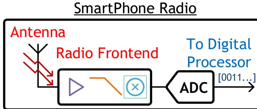
Figure 1.1: A representation of a smartphone radio with an analog-to-digital converter is presented.
