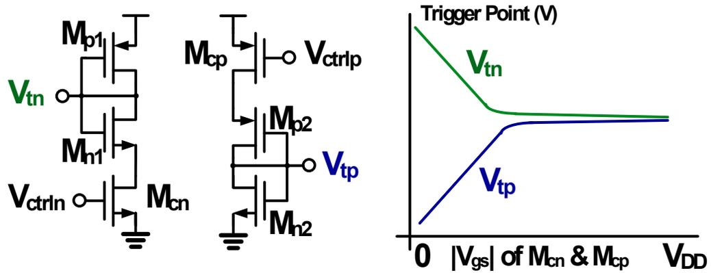
Figure 4.3: Trigger point of two current-starved inverters versus the absolute value of their gate voltages is seen. The variants of the current-starved inverters have either PMOS or NMOS control transistors.
