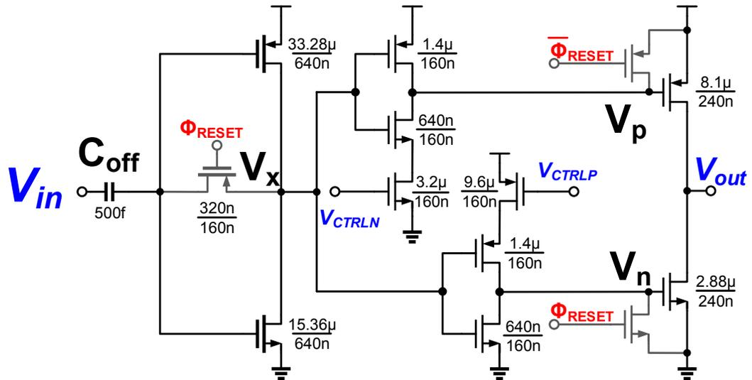
Figure 4.4: Circuit diagram of the pseudo-differential current-starved inverter ring amplifier used in this prototype pipelined ADC. Sizing is shown for amplifier in the first stage of the pipelined ADC.
