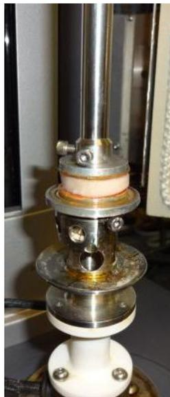
Figure 1: A blubber sample coin loaded in the AR2000ex rotational rheometer to measure the dynamic shear moduli  $G'$  and  $G''$ .
