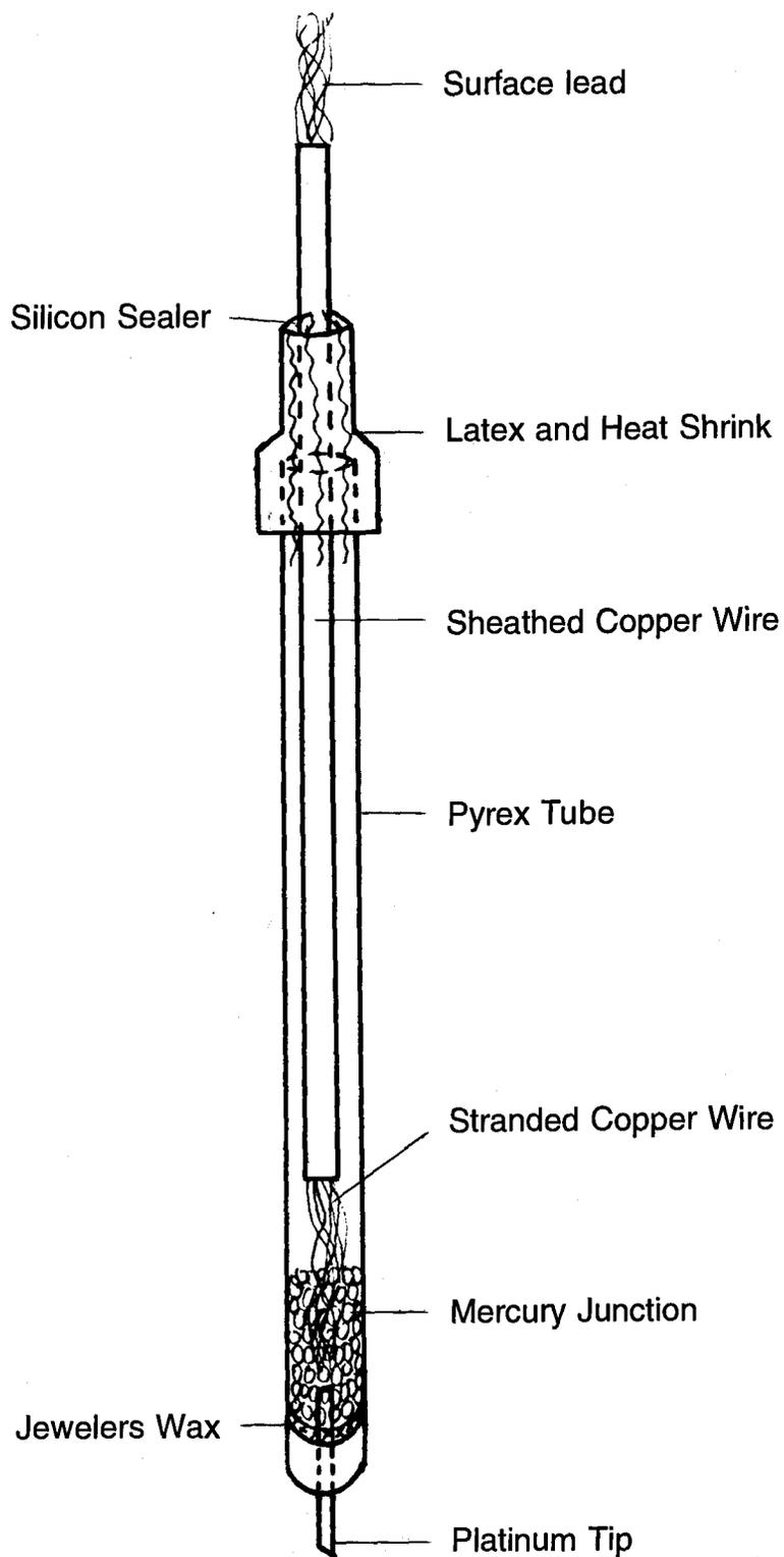
Figure 38. Field setup for electrode measurements.
