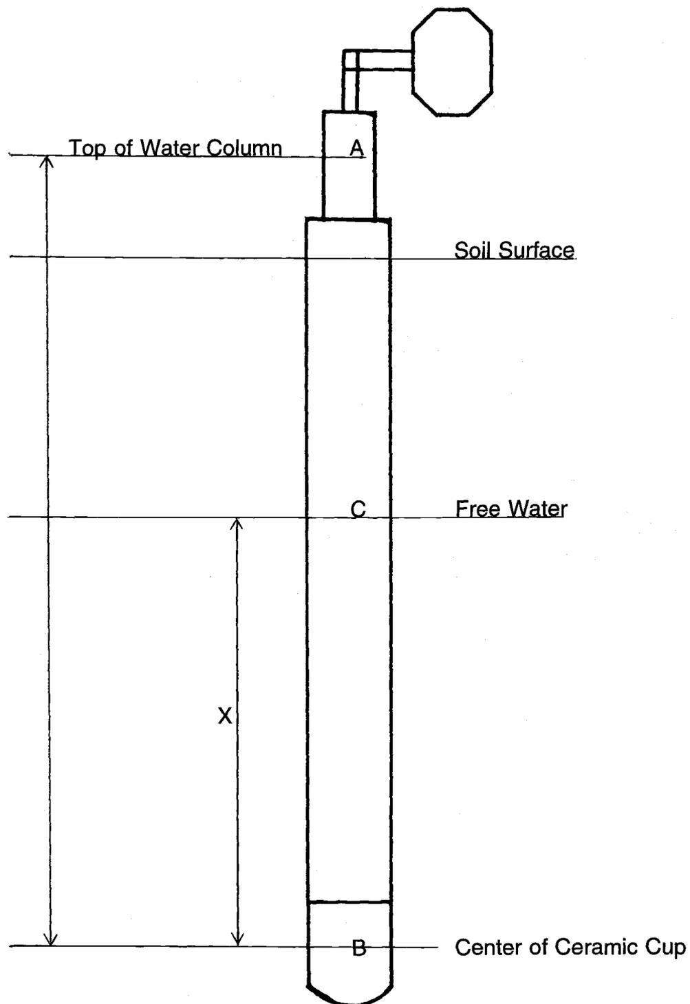
Calculation of water table depth using tensiometer data:
